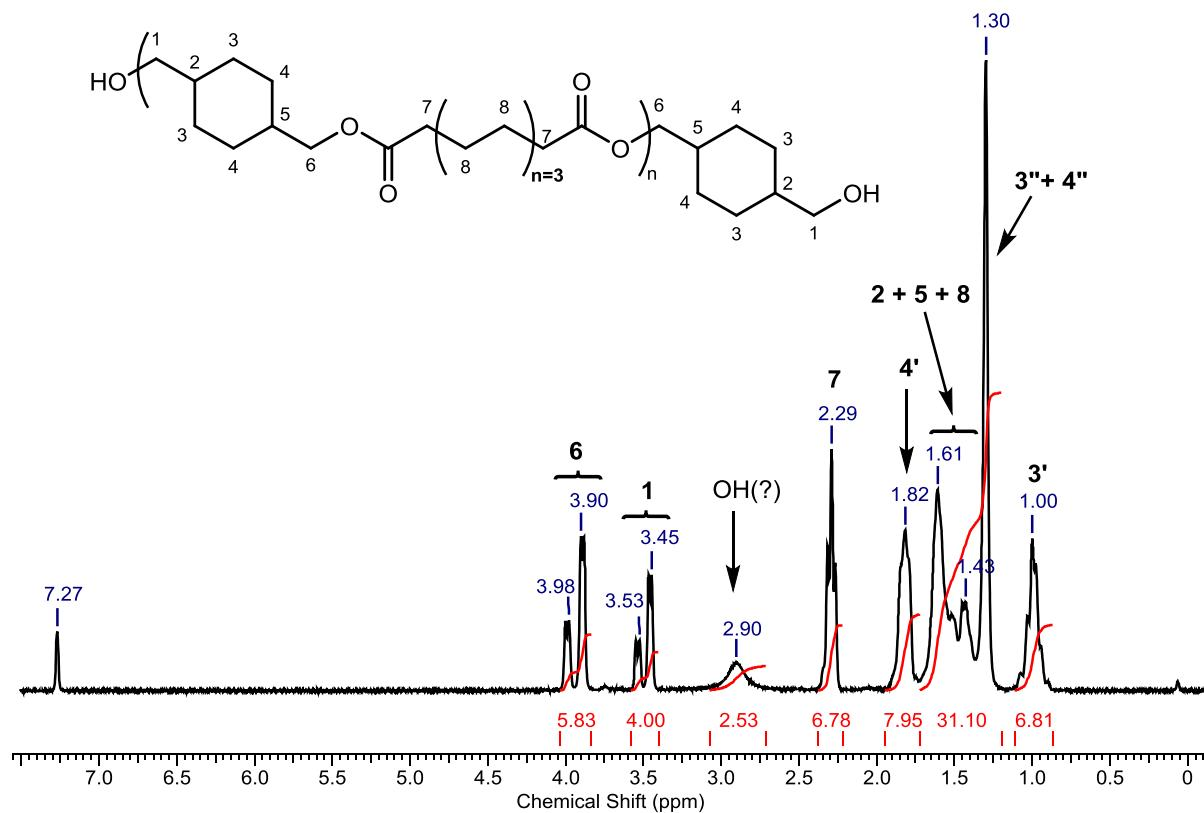
Figure 35.  $^1\text{H}$ -NMR analysis of trimer 1,4-cyclohexanedimethanol-sebacate.
