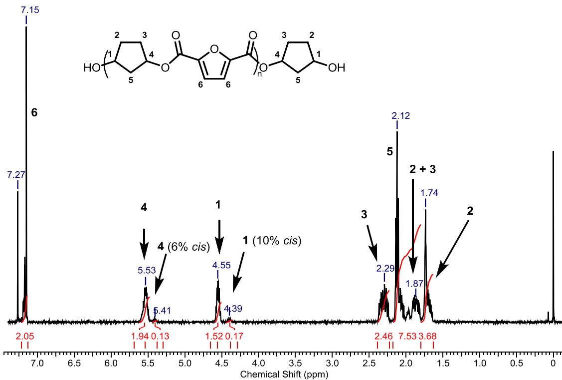
Figure 11. <sup>1</sup>H-NMR analysis of trimer 1,3-cyclopentanediol-furanoate – 8% *cis*.
