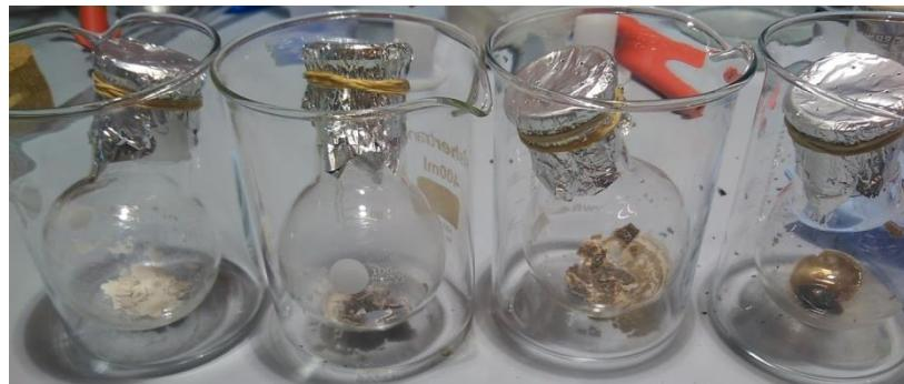
**Figure 3.** Obtained trimers of 1,3-CP-F, with varying *cis* content (8%, 20%, 30%, 40%, left to right), after drying at 110 °C, showing various stages of discoloration.
