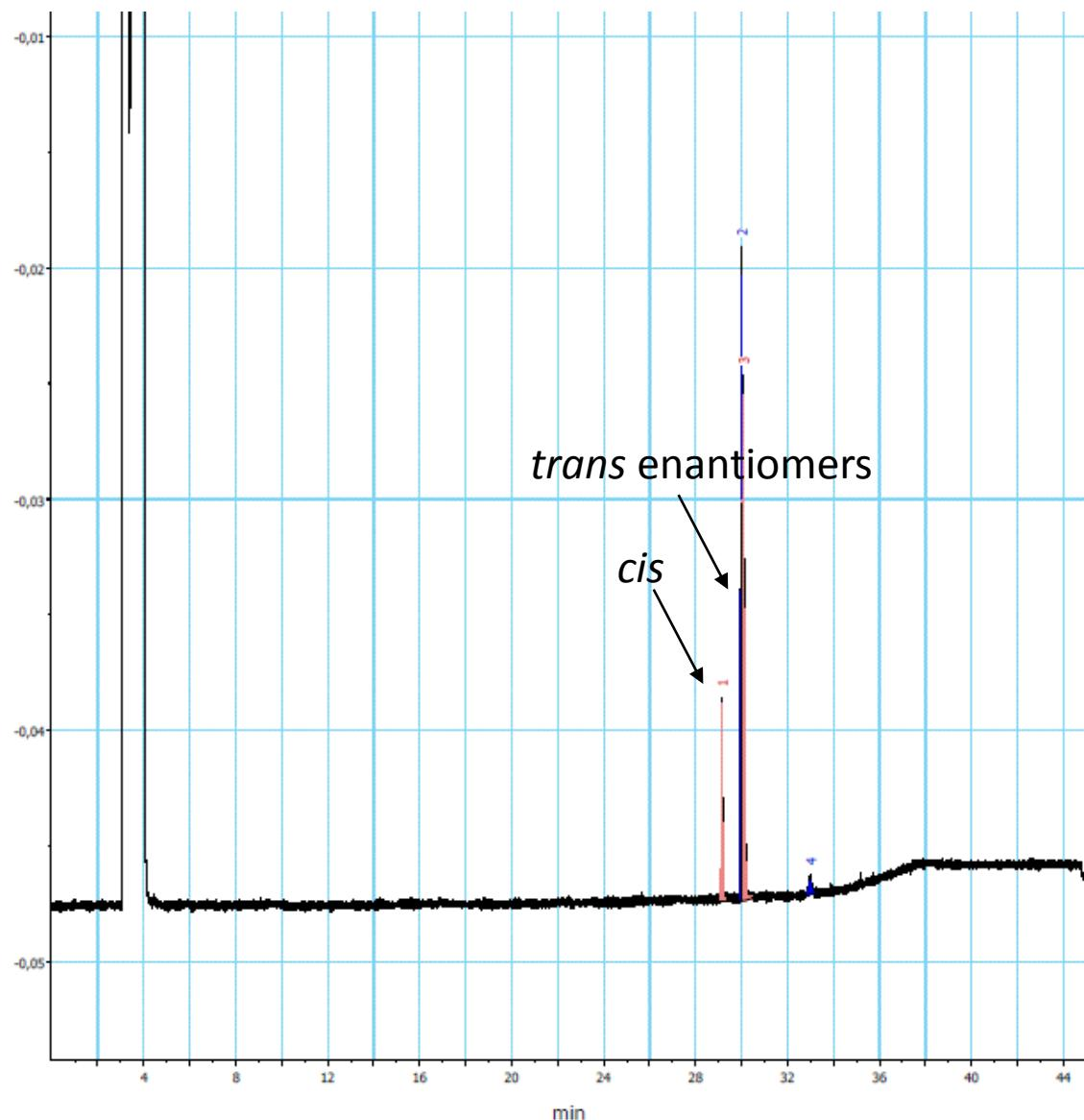
**Figure 1.** Chiral GC chromatogram on the commercial batch of 1,3-cyclopentanediol.
