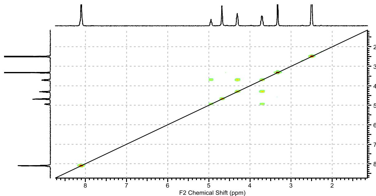
Figure 6. COSY (<sup>1</sup>H-<sup>1</sup>H) NMR analysis of trimer 1,2-ethyleneglycol-terephthalate.
