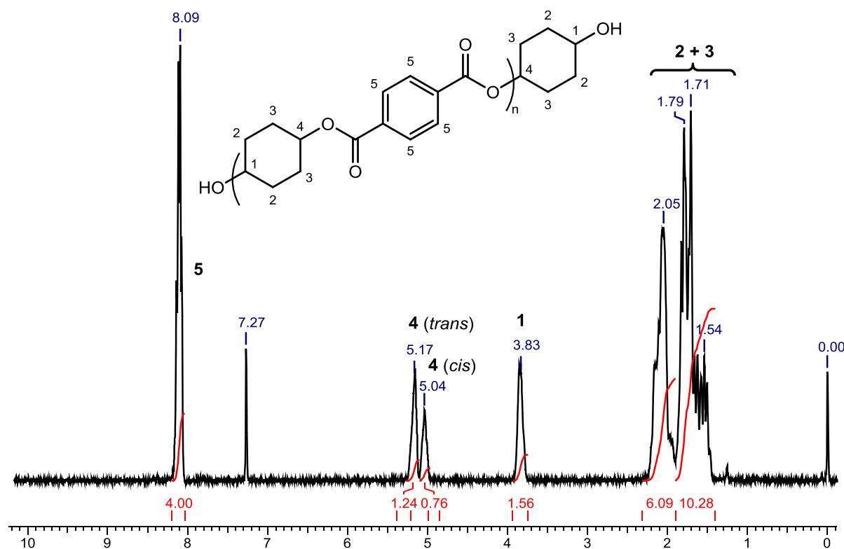
Figure 21.  $^1\text{H}$ -NMR analysis of trimer 1,4-cyclohexanediol-terephthalate.
