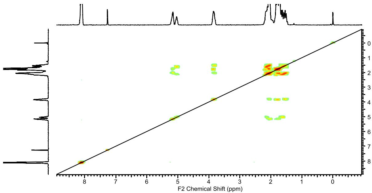
Figure 23. COSY ( $^1\text{H}$ - $^1\text{H}$ ) NMR analysis of trimer 1,4-cyclohexanediol-terephthalate.
