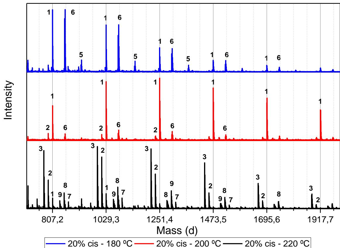
**Figure 41.** Obtained MALDI-ToF-MS spectra for poly(1,3-CP-F) with 20% cis, after thermal stability experiments at 180 °C (blue, top), 200 °C (red, middle), and 220 °C (black, bottom).
