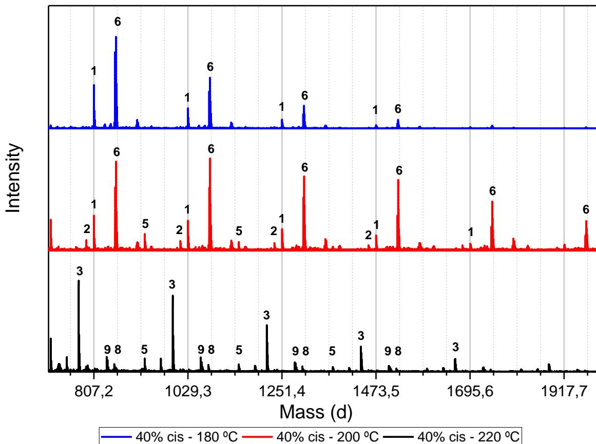
**Figure 43.** Obtained MALDI-ToF-MS spectra for poly(1,3-CP-F) with 40% cis, after thermal stability experiments at 180 °C (blue, top), 200 °C (red, middle), and 220 °C (black, bottom).
