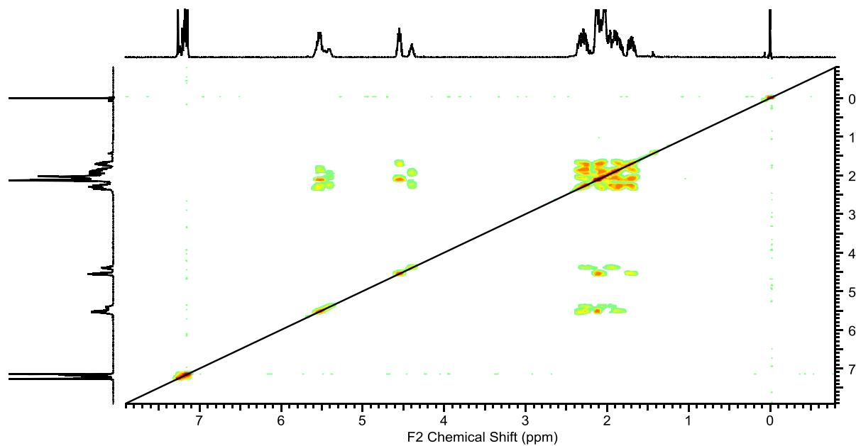
Figure 14. COSY ( $^1\text{H}$ - $^1\text{H}$ ) NMR analysis of trimer 1,3-cyclopentanediol-furanoate – 30% *cis*.
