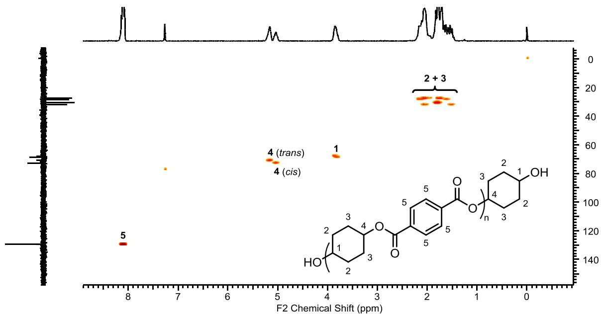
Figure 24. HSQC ( $^1\text{H}$ -DEPT) NMR analysis of trimer 1,4-cyclohexanediol-terephthalate.
