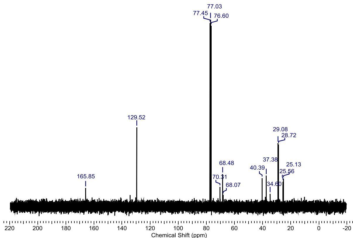
Figure 30.  $^{13}\text{C}$ -NMR analysis of trimer 1,4-cyclohexanedimethanol-terephthalate.
