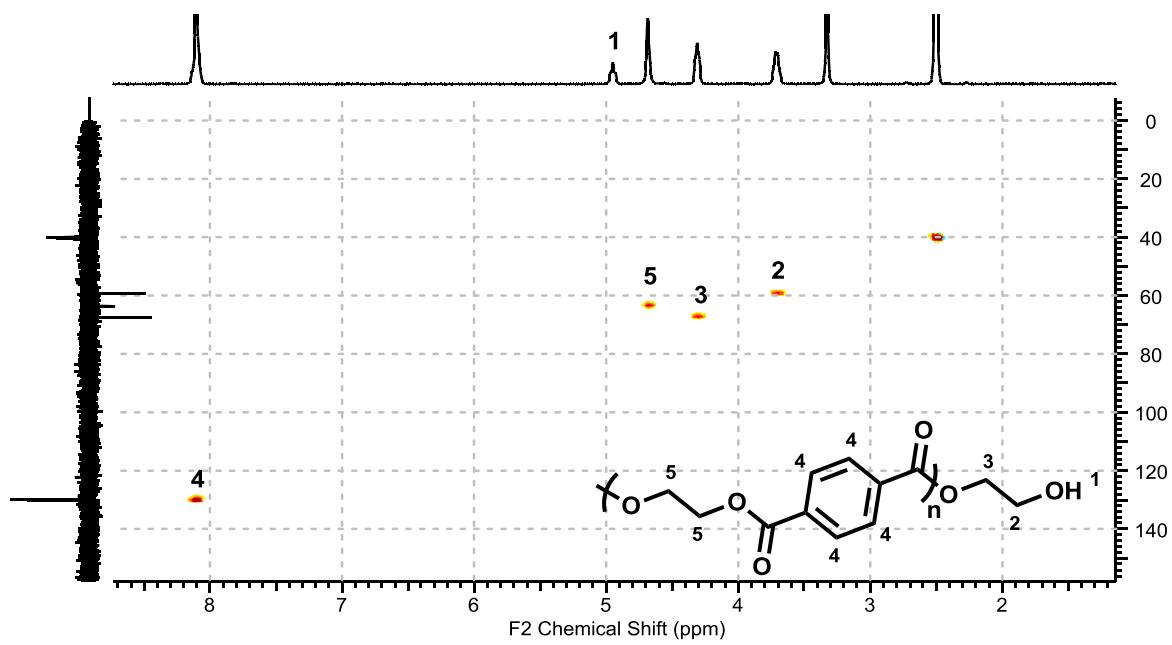
Figure 7. HSQC ( $^1\text{H}$ -DEPT) NMR analysis of trimer 1,2-ethyleneglycol-terephthalate.
