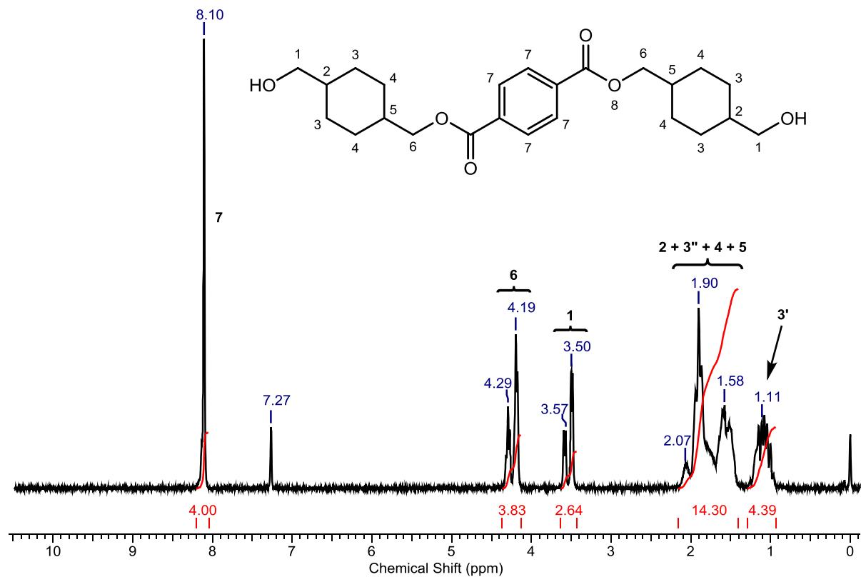
Figure 29.  $^1\text{H}$ -NMR analysis of trimer 1,4-cyclohexanedimethanol-terephthalate.
