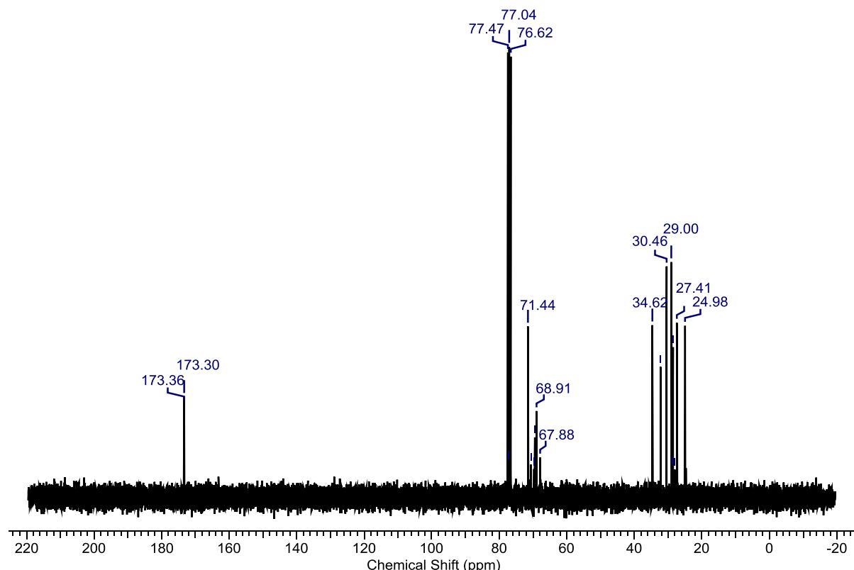
Figure 28.  $^{13}\text{C}$ -NMR analysis of trimer 1,4-cyclohexanediol-sebacate.
