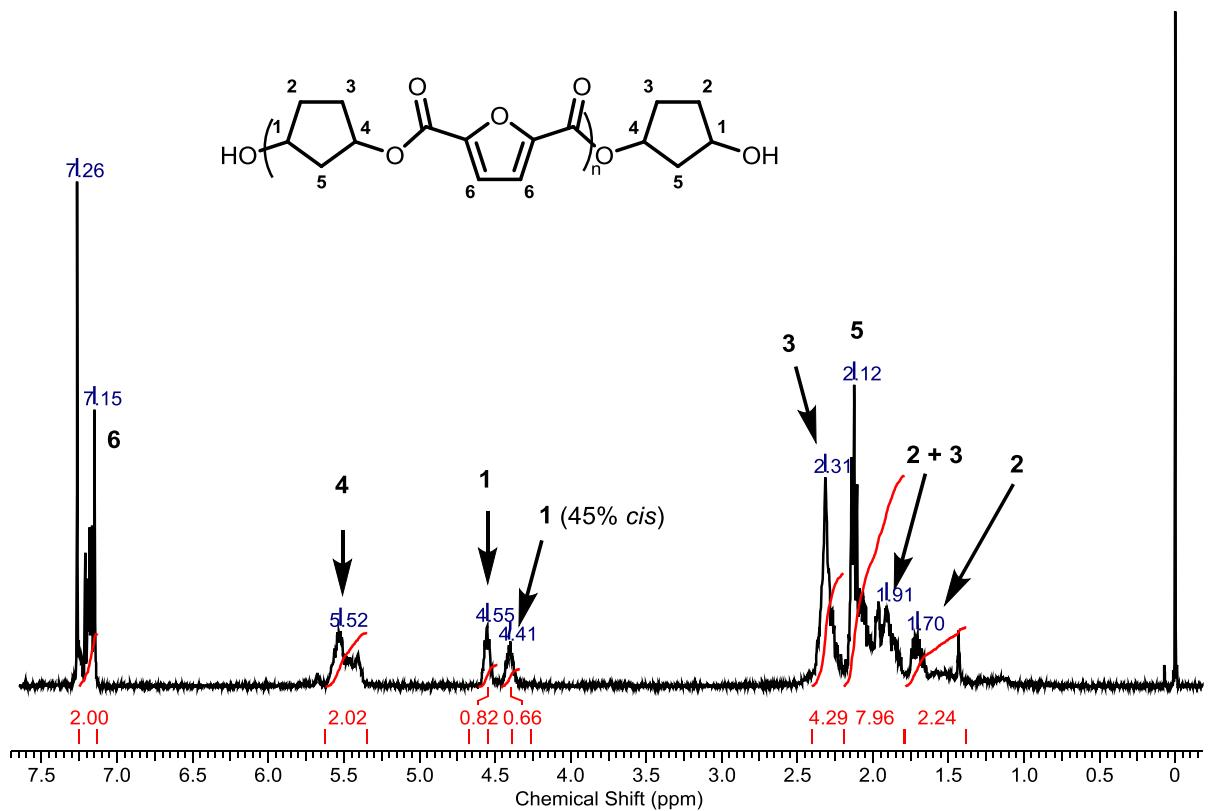
Figure 16.  $^1\text{H}$ -NMR analysis of trimer 1,3-cyclopentanediol-furanoate – 40% *cis*.
