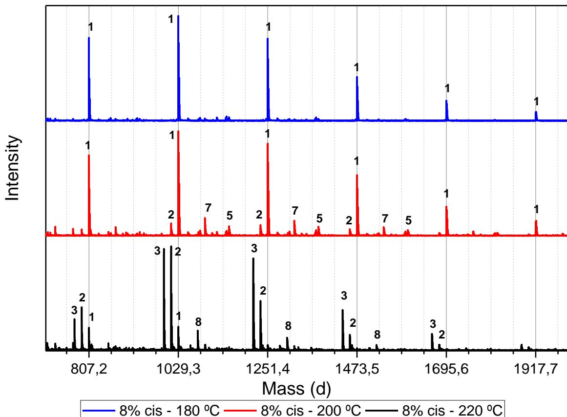
**Figure 40.** Obtained MALDI-ToF-MS spectra for poly(1,3-CP-F) with 8% cis, after thermal stability experiments at 180 °C (blue, top), 200 °C (red, middle), and 220 °C (black, bottom).
