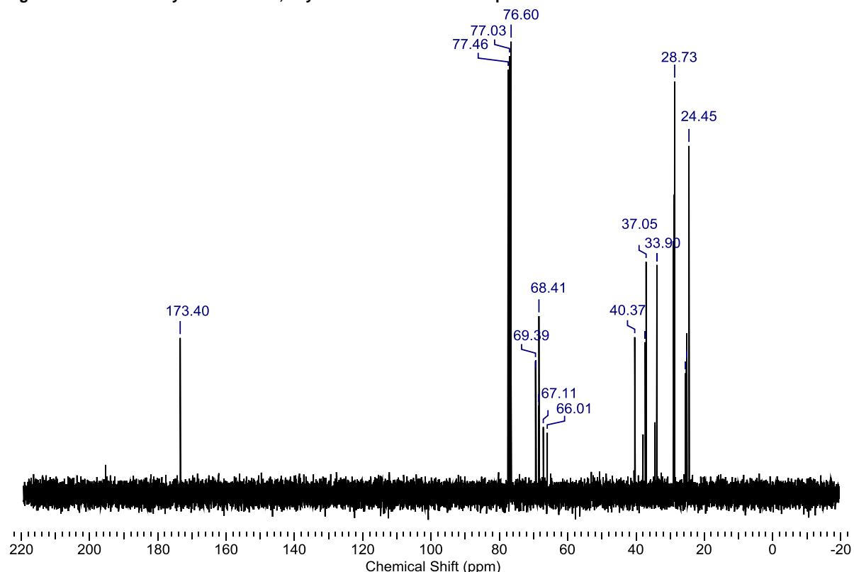
Figure 34.  $^{13}\text{C}$ -NMR analysis of trimer 1,4-cyclohexanedimethanol-adipate.
