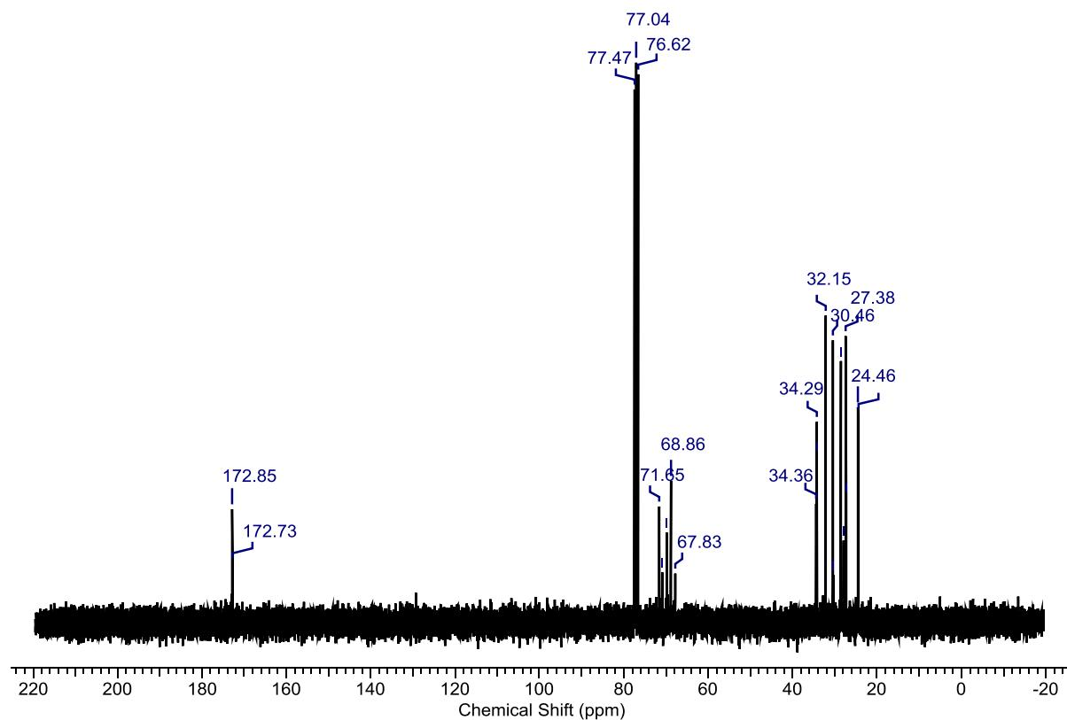
Figure 26.  $^{13}\text{C}$ -NMR analysis of trimer 1,4-cyclohexanediol-adipate.
