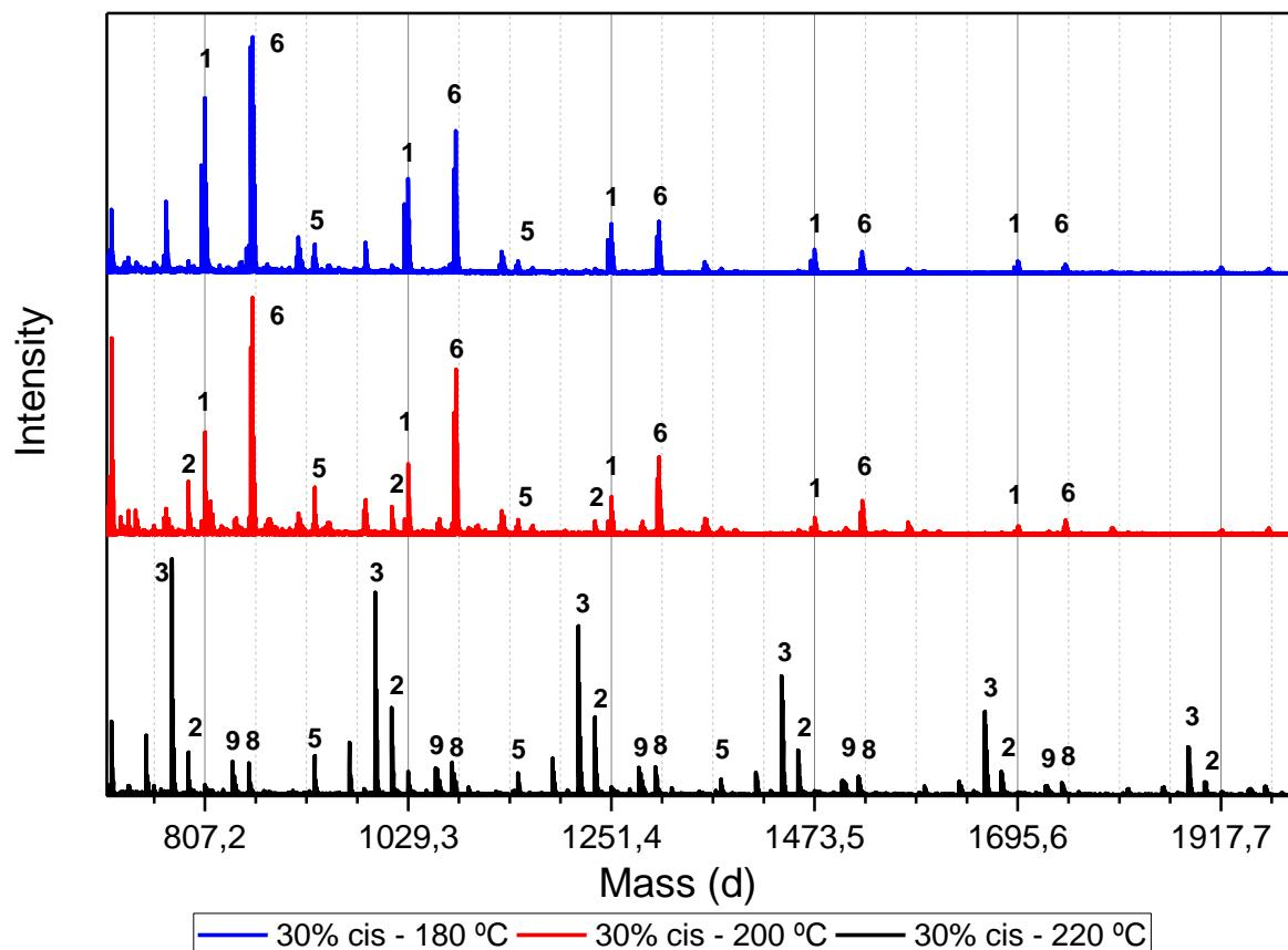
**Figure 42.** Obtained MALDI-ToF-MS spectra for poly(1,3-CP-F) with 30% cis, after thermal stability experiments at 180 °C (blue, top), 200 °C (red, middle), and 220 °C (black, bottom).
