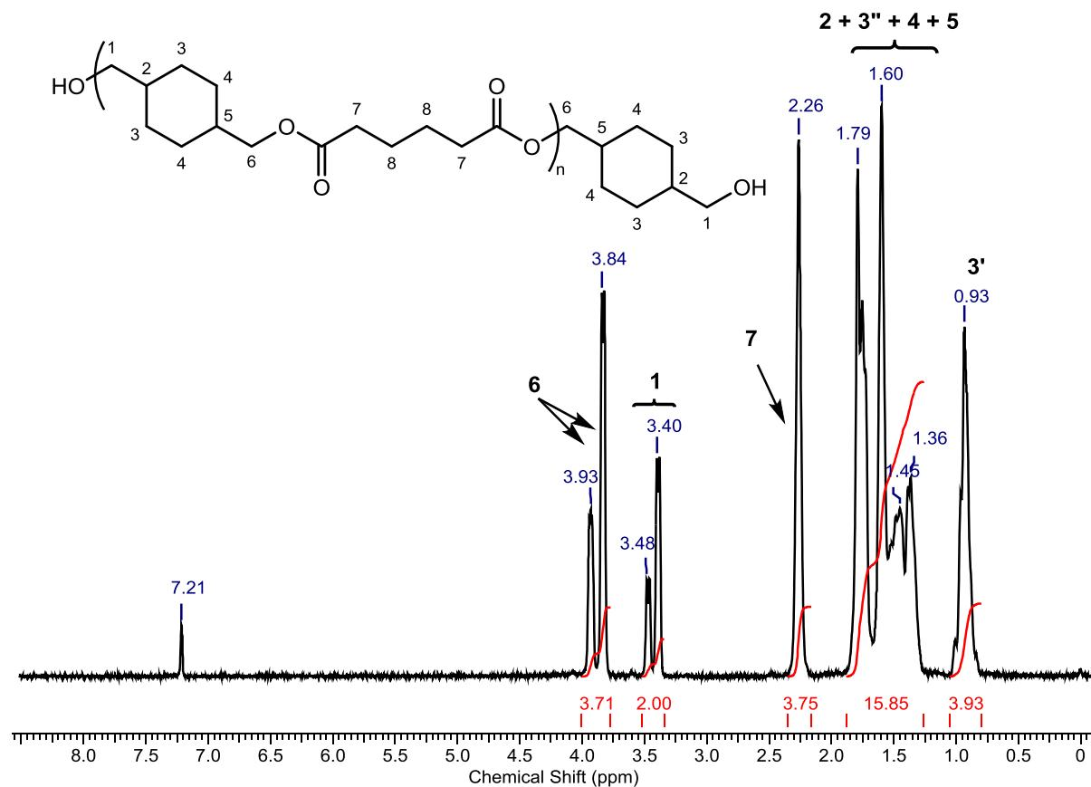
Figure 33.  $^1\text{H}$ -NMR analysis of trimer 1,4-cyclohexanedimethanol-adipate.
