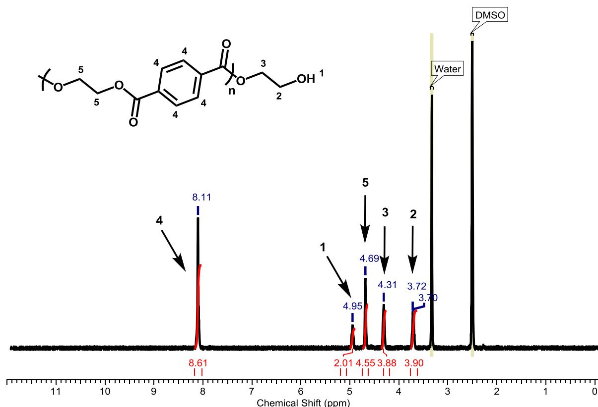
Figure 5. <sup>1</sup>H-NMR analysis of trimer 1,2-ethyleneglycol-terephthalate.
