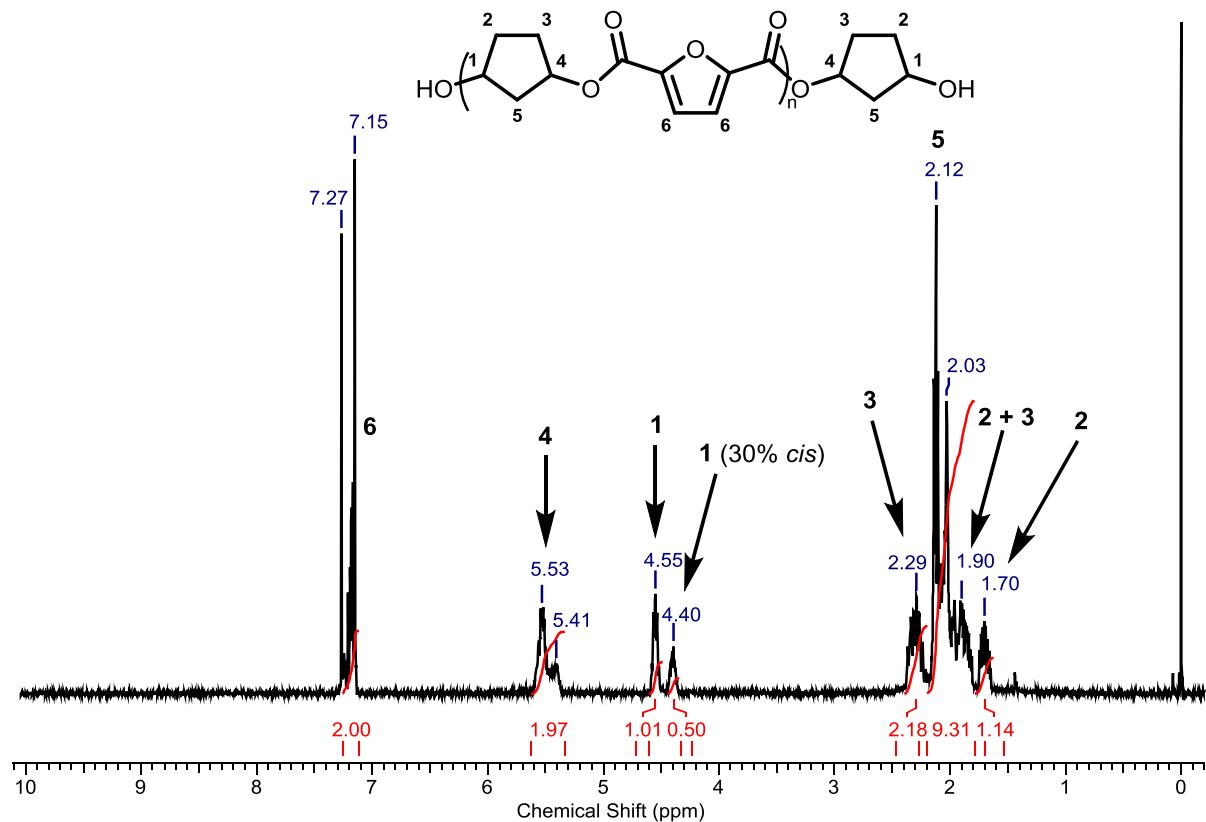
Figure 13.  $^1\text{H}$ -NMR analysis of trimer 1,3-cyclopentanediol-furanoate – 30% *cis*.
