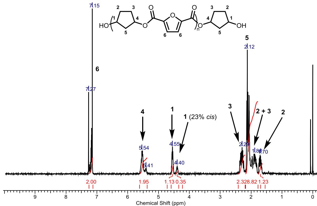
Figure 12. <sup>1</sup>H-NMR analysis of trimer 1,3-cyclopentanediol-furanoate – 20% *cis*.
