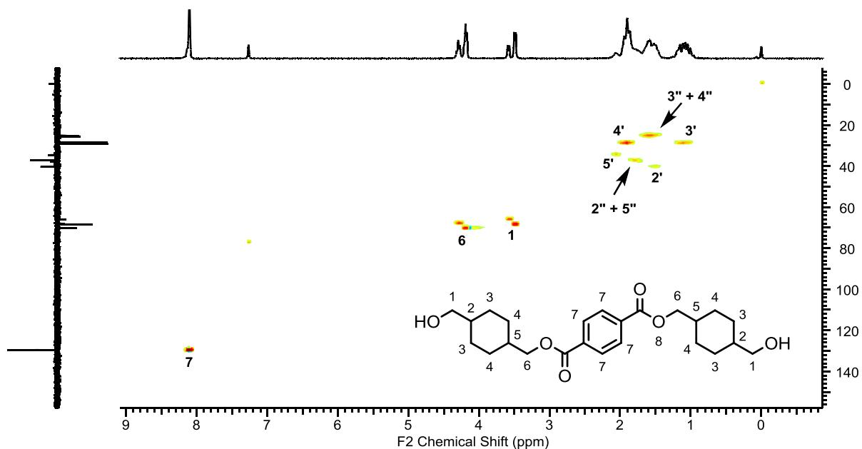
Figure 32. HSQC ( $^1\text{H}$ -DEPT) NMR analysis of trimer 1,4-cyclohexanedimethanol-terephthalate.
