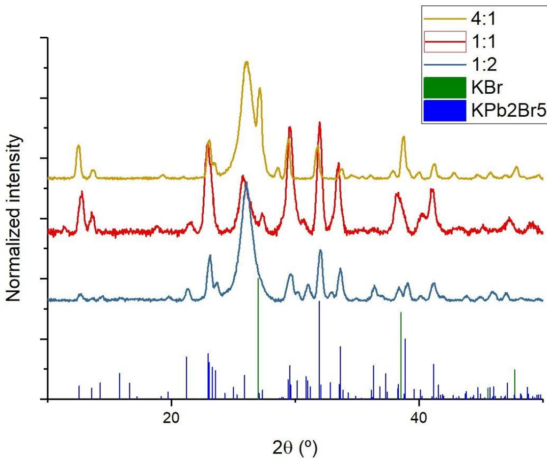
Figure S 2. Diffractograms of powders prepared by ball-milling KBr and  $\text{PbBr}_2$  in different molar ratios (1:2, 1:1, and 4:1). Reference patterns for bulk KBr (ICSD: 18015) and  $\text{KPb}_2\text{Br}_5$  (ICSD: 250266) are presented as green and blue columns. The broad signal around  $2\theta = 25^\circ$  corresponds to the substrate on which the powders are deposited for XRD characterization.
