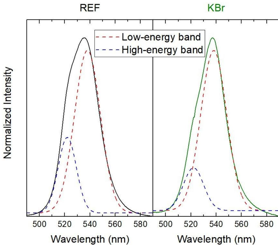
Figure S 4. Photoluminescence spectra of reference and KBr sample fitted with two gaussian peaks. The KBr sample shows a reduction in the relative intensity of the high-energy component as explained in the main text.
