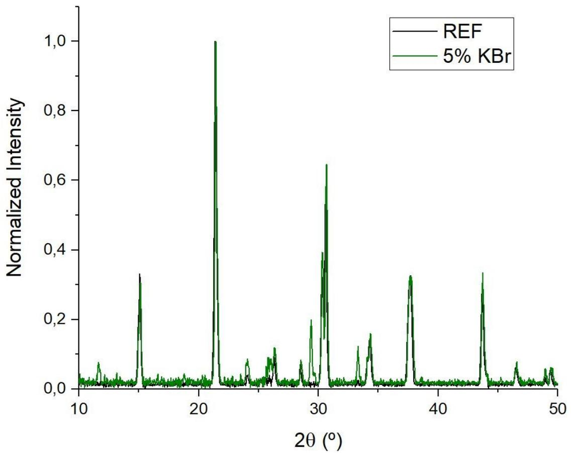
Figure S 3. XRD signal of samples prepared from pure CsBr (black line) and partly (5%) substituted by KBr (green line). Effects of KBr are qualitatively similar than in the case of 20% (Figure S1 and Figure 1) although to a lesser extent, as may be expected by a lower percentage of KBr.
