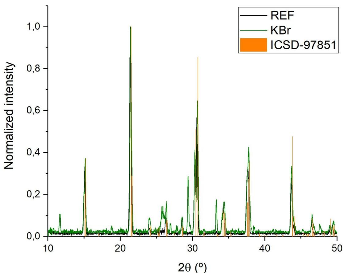
Figure S 1. XRD signal of samples prepared from pure CsBr (black line) and partly (20%) substituted by KBr (green line). Selected areas of the diffractograms are shown in Figure 1. Reference pattern for bulk orthorhombic CsPbBr<sub>3</sub> is shown as orange columns.
