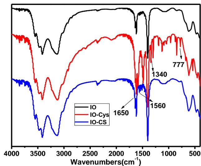
Figure S1. FTIR spectrum of IO, IO-Cys and IO-CS. The peak appeared at 777 cm<sup>-1</sup> was due to stretch of C-S after conjugation of cysteine on the surface of IO. -COOH group of cysteine appeared at 1340 cm<sup>-1</sup>[1]. C=O in amide group (amide I band) appeared at 1650 cm<sup>-1</sup> after modification of IO with chitosan. The peak at 1560 cm<sup>-1</sup> was attributed to NH-bending vibration in amide group[2].
