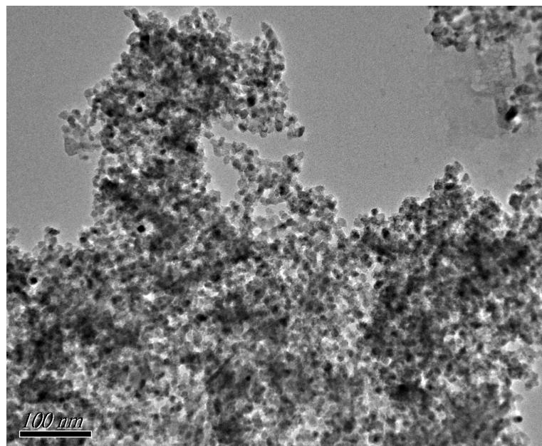
Fig. S1 TEM image of as-prepared  $\text{Ag}_3\text{PO}_4$  nanocrystals
