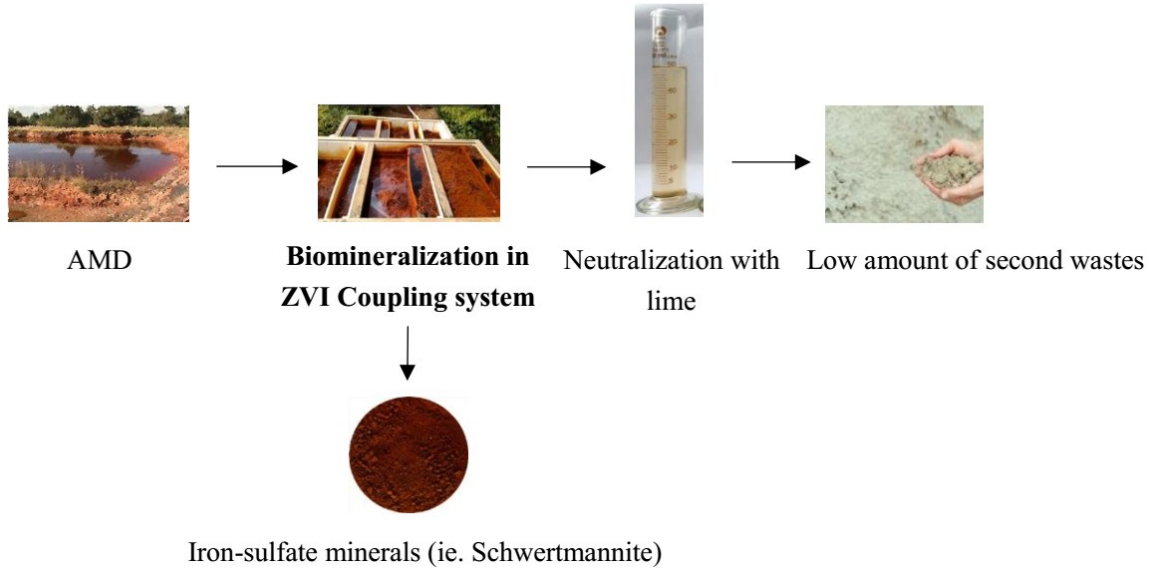
Fig. S1 The flow chart of (A) AMD treatment by neutralization with lime and (B) AMD treatment by biological mineralization in A. ferrooxidans system coupling with zero-valent iron before neutralization with lime
