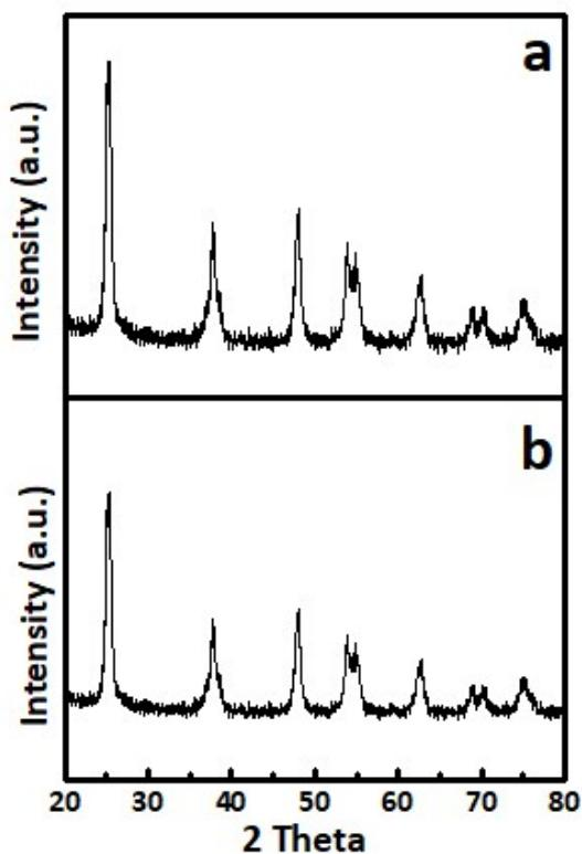
Fig. S11. XRD pattern of (a) 5% Cr-TiO<sub>2</sub> calcined at 400°C and (b) 5% Cr-TiO<sub>2</sub> recovered after 3<sup>rd</sup> cycles of photo-degradation of spentwash solution under sunlight
