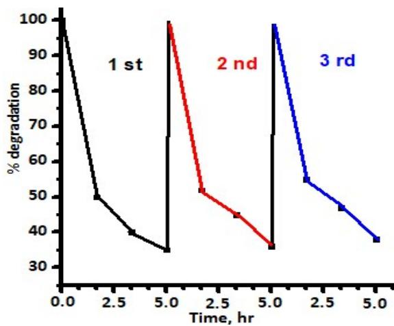
Fig. S12. Degradation of spent wash using 5% Cr-TiO<sub>2</sub> catalyst under natural sunlight for 3 consecutive cycles.
