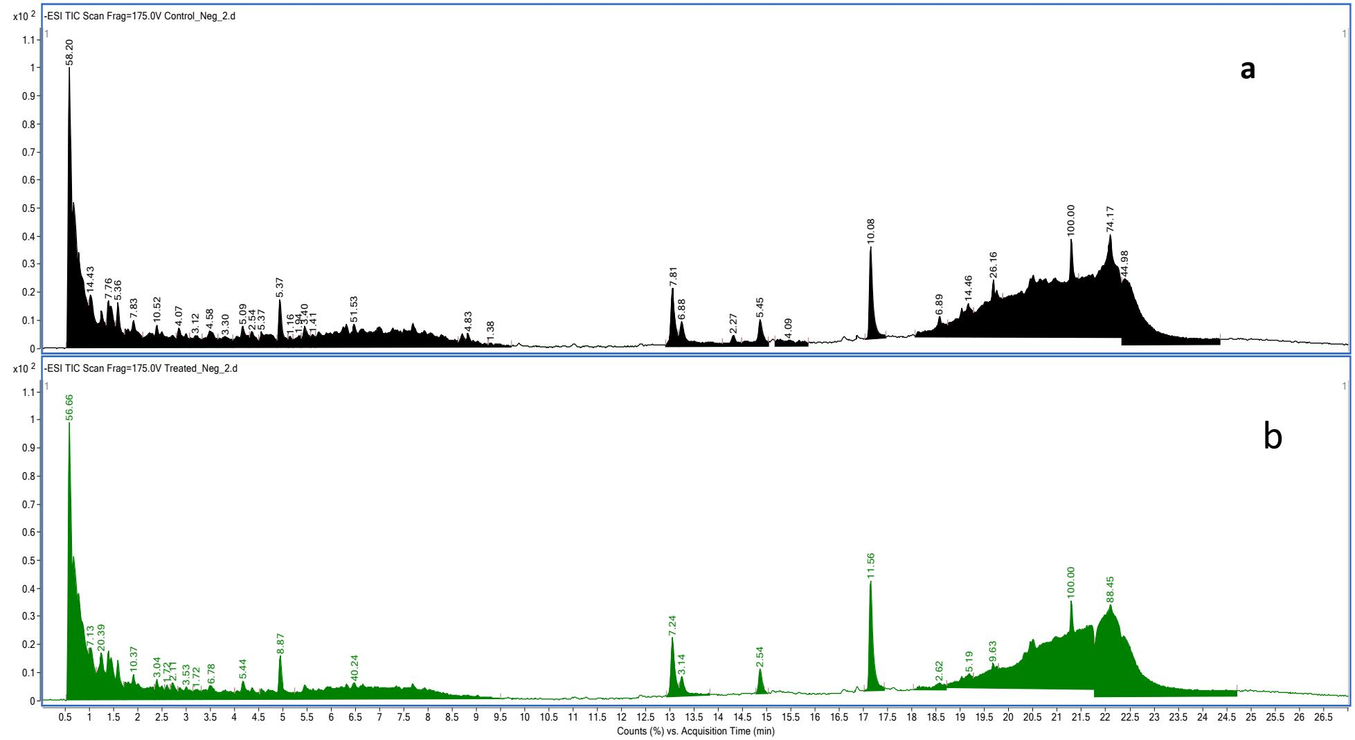
Fig.S8 Negative ESI TIC fragmentation spectra of spentwash after irradiation with sunlight (a) Undoped TiO<sub>2</sub>, (b) 5% Cr- TiO<sub>2</sub>.
