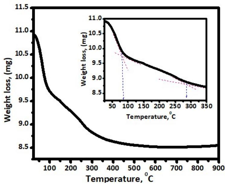
Fig.S1. Thermo-gravimetric analysis of 5% Cr-TiO<sub>2</sub> powdered gel sample.
