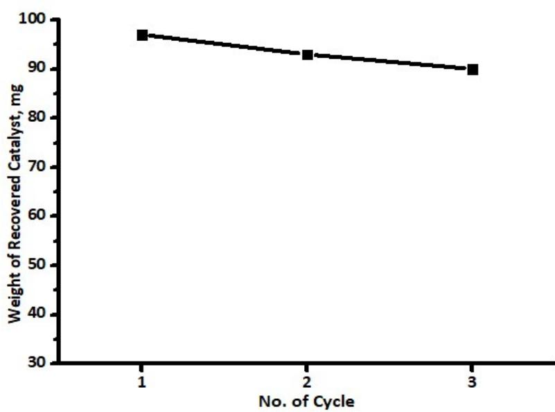
Fig. S13 Recovery of 5% Cr-TiO<sub>2</sub> catalyst with respect to number of cycle.
