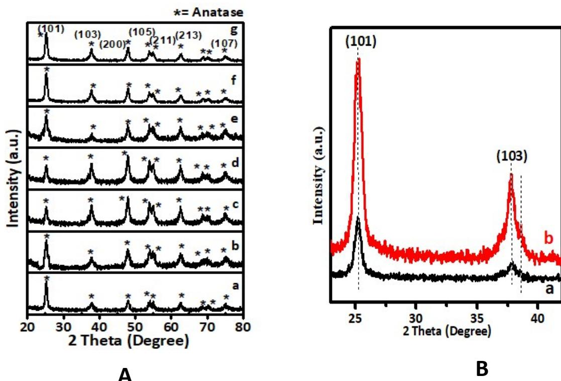
Fig. S2 (A) XRD pattern of (a) Undoped TiO<sub>2</sub> (b) 0.5% Cr-TiO<sub>2</sub> (c) 1% Cr-TiO<sub>2</sub> (d) 2% Cr-TiO<sub>2</sub>, (e) 3% Cr-TiO<sub>2</sub>, (f) 4% Cr-TiO<sub>2</sub> and (g) 5% Cr-TiO<sub>2</sub> samples obtained by Calcination at 400°C. and (B) Enlarged version XRD pattern of (110) plane (a) Undoped TiO<sub>2</sub> and (b) 5% Cr-TiO<sub>2</sub>
