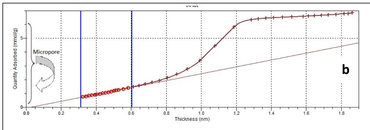
Fig.S4. t plot of mesoporous catalyst (a) Undoped TiO<sub>2</sub>. (b) 5% Cr-TiO<sub>2</sub>.
