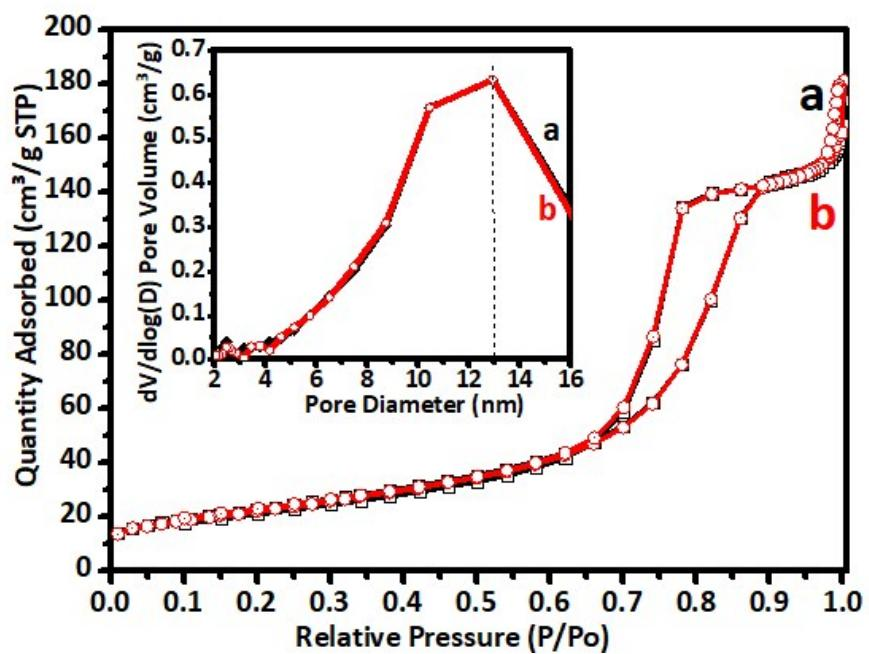
Fig.S3. Nitrogen sorption isotherm of (a) Cr-TiO<sub>2</sub> at 500°C and (b) Cr-TiO<sub>2</sub> at 600°C. In inset BJH pore size distribution curve of (a) 5% Cr-TiO<sub>2</sub> at 500°C and (b) 600°C of 5% Cr-TiO<sub>2</sub> catalyst
