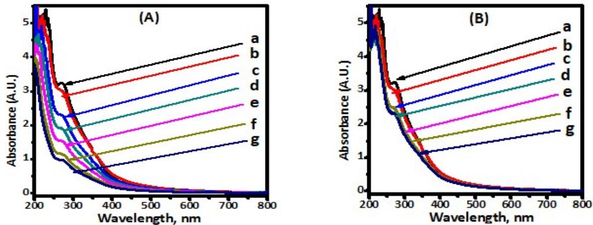
Fig.S6. UV Visible spectra of spentwash solution after irradiation with sunlight (A) for 5% Cr- TiO<sub>2</sub> catalyst and (B) for P-25 Degussa Catalyst for (a) 0 hr, (b) 1 hr, (c) 2 hr, (d) 2.30 hr, (e) 3 hr, (f) 4 hr and (g) 5 hr.
