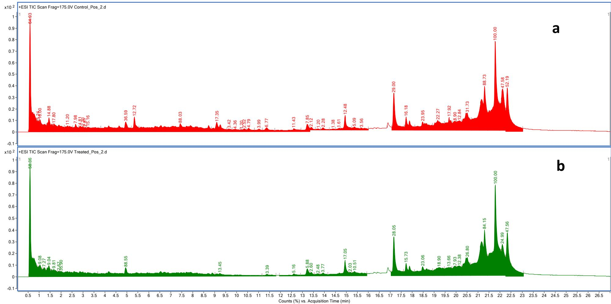
Fig.S9. Positive ESI TIC fragmentation spectra of spentwash after irradiation with sunlight (a) Undoped TiO<sub>2</sub>, (b) 5% Cr-TiO<sub>2</sub>
