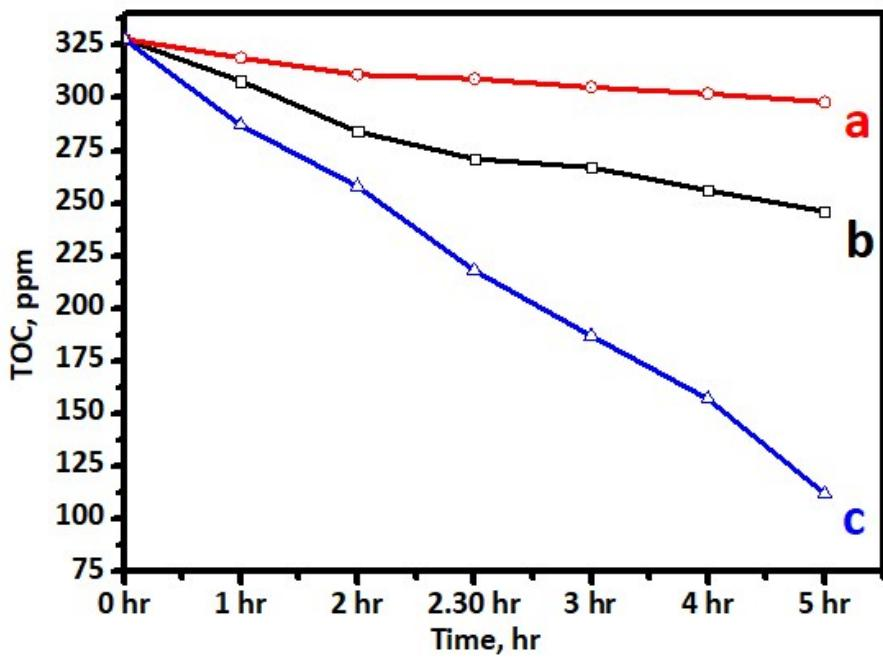
Fig. S10 Reduction of TOC during photocatalytic trial on spentwash for (a) Undoped TiO<sub>2</sub>, (b) Degussa P-25, (c) 5% Cr-TiO<sub>2</sub> catalyst.
