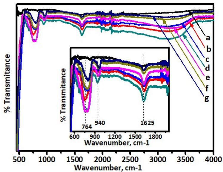
Fig.S5. FT-IR spectra of (a)Undoped TiO<sub>2</sub> (b) 0.5% Cr-TiO<sub>2</sub> (c) 1% Cr-TiO<sub>2</sub> (d) 2% Cr-TiO<sub>2</sub>, (e) 3% Cr-TiO<sub>2</sub>, (f) 4% Cr-TiO<sub>2</sub> and (g) 5% Cr-TiO<sub>2</sub> samples
