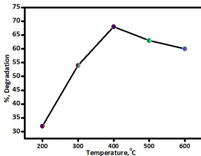
Fig. S7. Degradation of spent wash using 5% Cr-TiO<sub>2</sub> catalyst calcined at different temperature.
