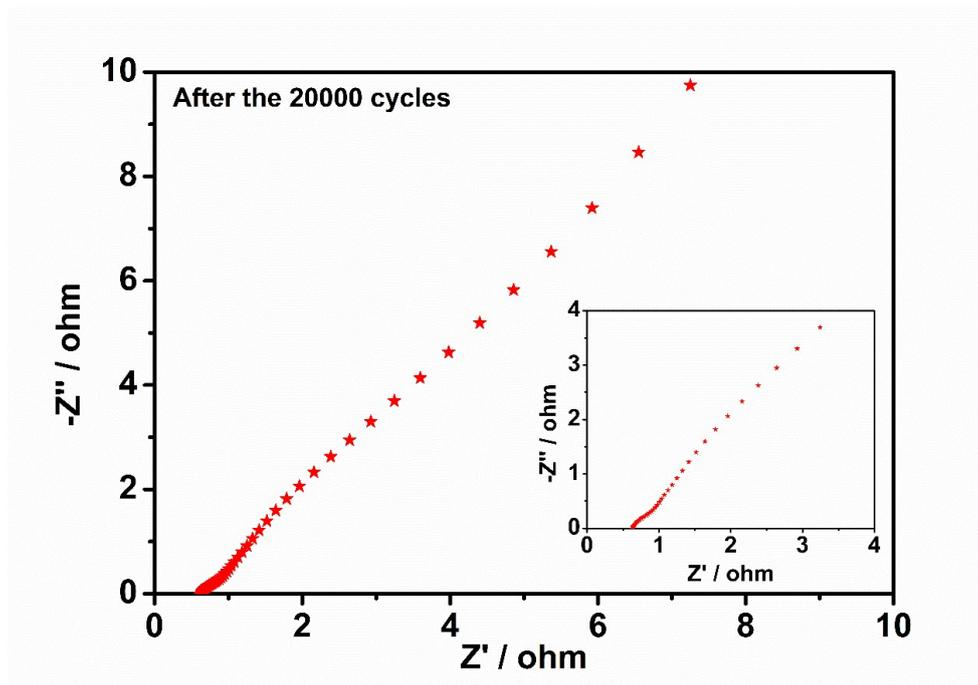
Fig. S7. EIS curves of the  $\text{CoV}_2\text{O}_6$  (inset shows the magnified) after 20,000 cycles
