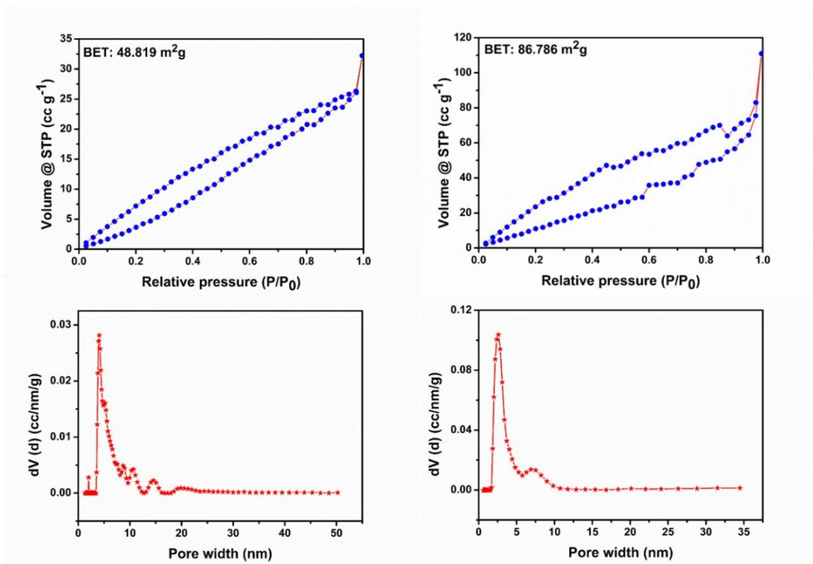
**Fig. S2.**  $N_2$  adsorption and desorption isotherms and the corresponding pore size distributions of (a, c)  $CoV_2O_6 \cdot 4H_2O$  and (b, d)  $CoV_2O_6$ .
