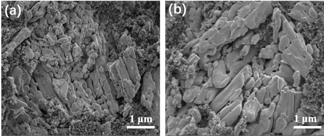
**Fig. S5** SEM patterns of  $\text{CoV}_2\text{O}_6$  after 20,000 cycles
