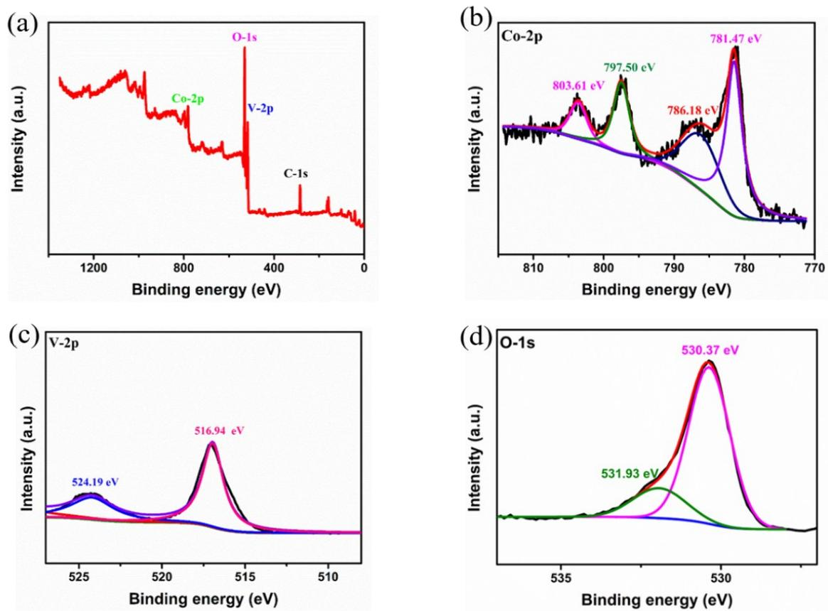
**Fig. S1.** XPS patterns of (a) full scan of the  $\text{CoV}_2\text{O}_6$ . (b) Co 2p, (c) V 2p and (d) O 1s
