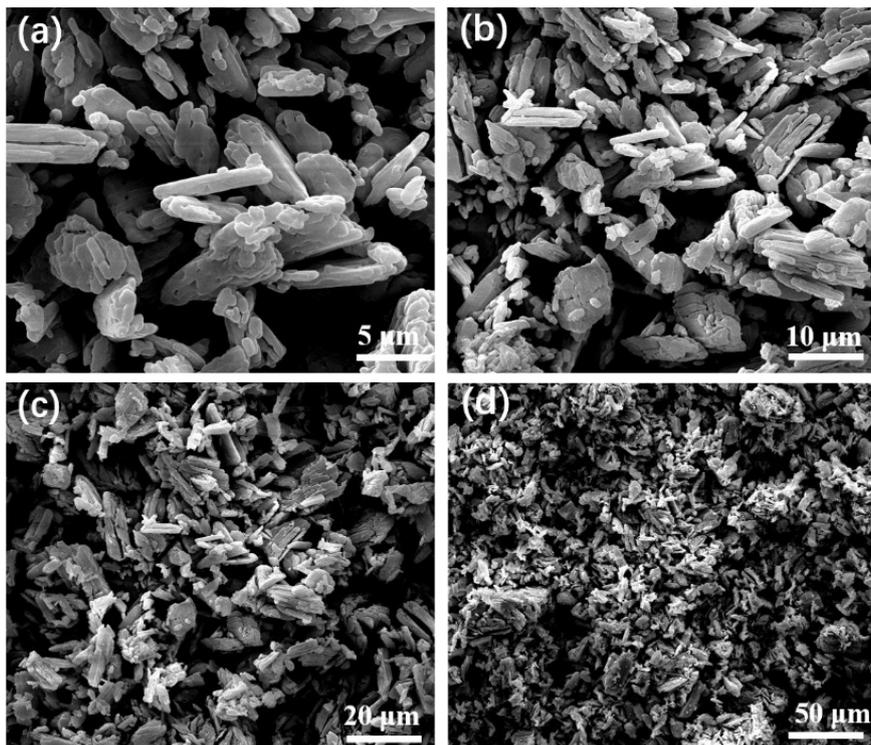
**Fig. S3** SEM images of  $\text{CoV}_2\text{O}_6$
