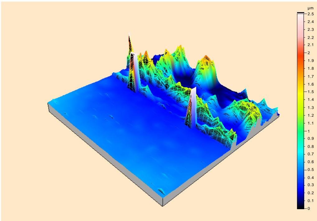
**Figure S 14.** SP profile scan of a polycarbonate (PC) surface partially treated with **3a**.
