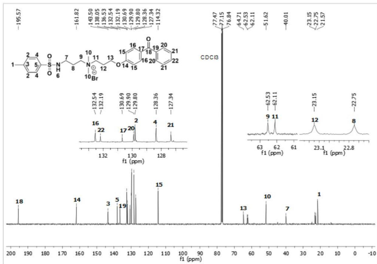
**Figure S 66.**  $^{13}\text{C}$  NMR (101 MHz,  $\text{CDCl}_3$ ) spectrum of **2a**.
