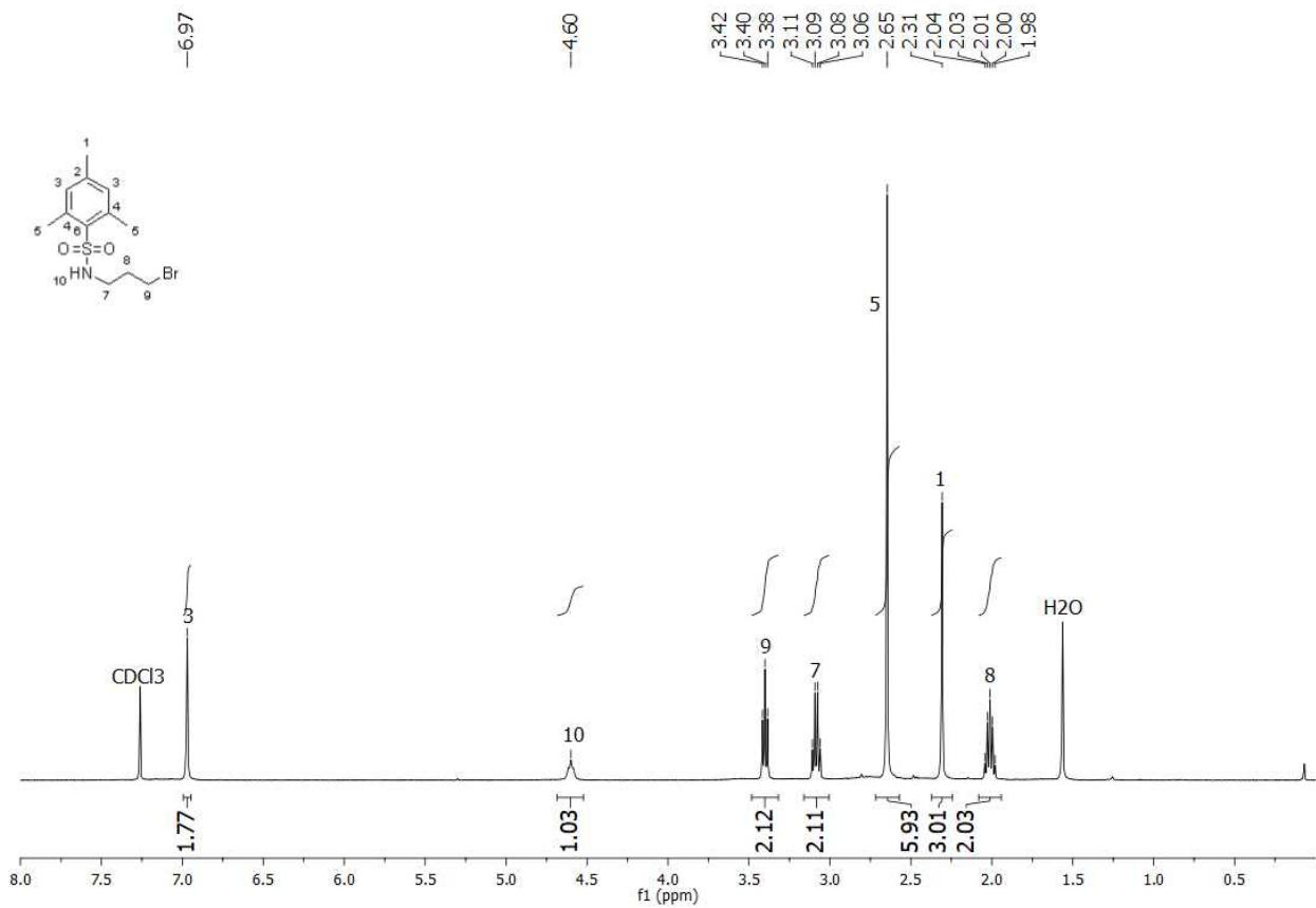
**Figure S 53.**  $^1\text{H}$  NMR (400 MHz,  $\text{CDCl}_3$ ) spectrum of **9**.
