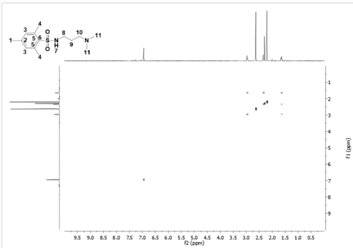
**Figure S 29.** COSY 2D NMR ( $\text{CDCl}_3$ ) spectrum of **3**.
