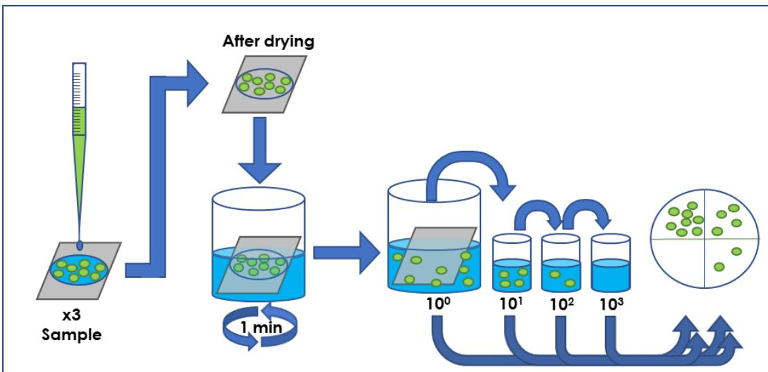
**Figure S 16.** Simplified schematic representation of the large drop inoculation (LDI) method.
