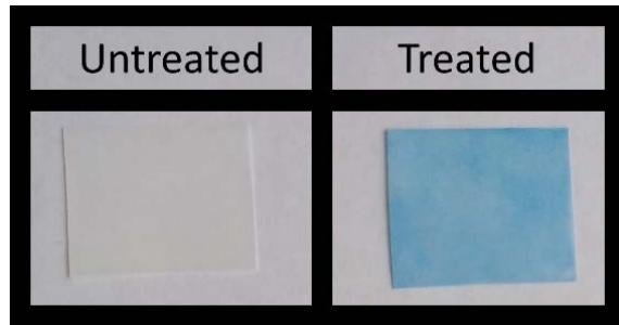
**Figure S 18.** Representative polystyrene samples, one left untreated (left) and treated (right) with **3a**, stained with bromophenol blue.
