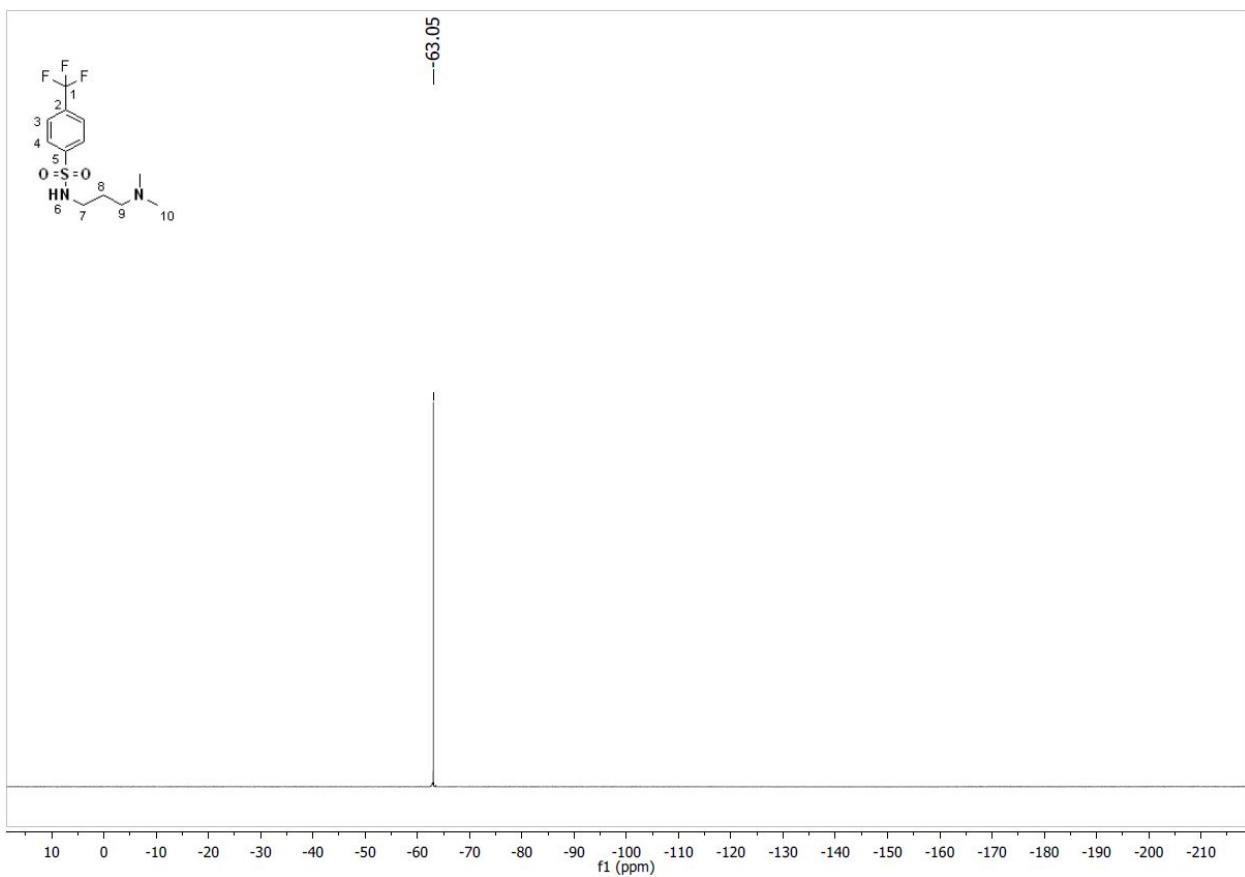
**Figure S 37.** <sup>19</sup>F NMR (376 MHz, CDCl<sub>3</sub>) spectrum of **5**.
