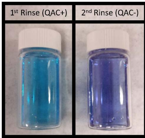
**Figure S 17.** Successive wash solutions of polystyrene coated with **3a**, exposed to 3 drops (~0.1 mL) 1000 ppm bromophenol blue dye. Samples were shaken for 30 seconds in sealed tubes containing 10 mL of distilled water. The blue colour indicates the first rinse contains the presence QAC, while the purple colour indicates the second rinse does not.
