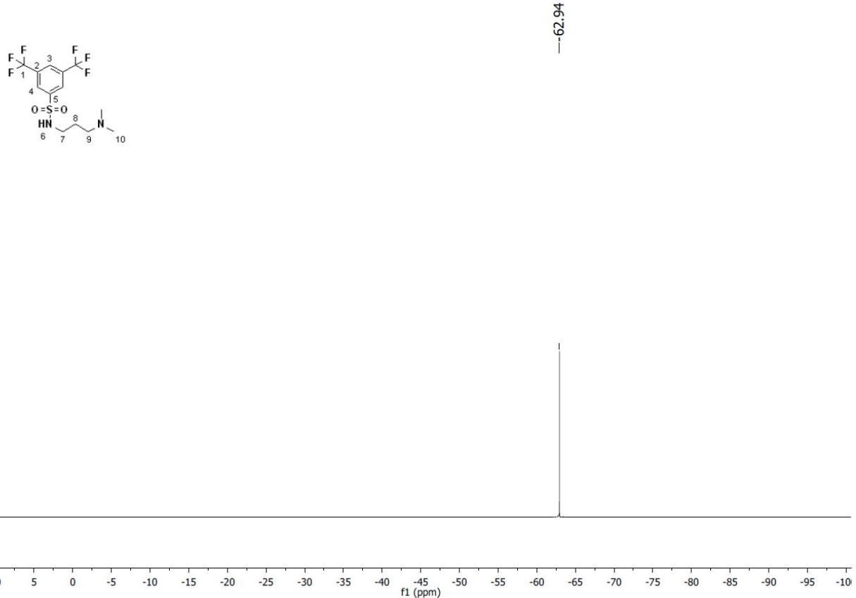
**Figure S 42.**  $^{19}\text{F}$  NMR (376 MHz,  $\text{CDCl}_3$ ) spectrum of **6**.
