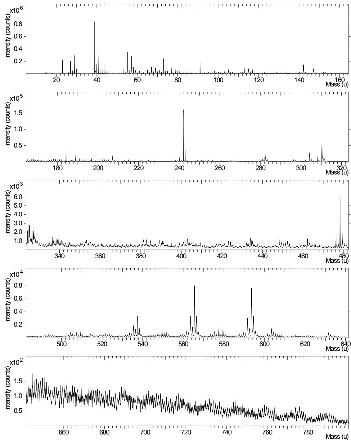
**Figure S 7.** Positive ion ToF-SIMS survey of control CPVC material.
