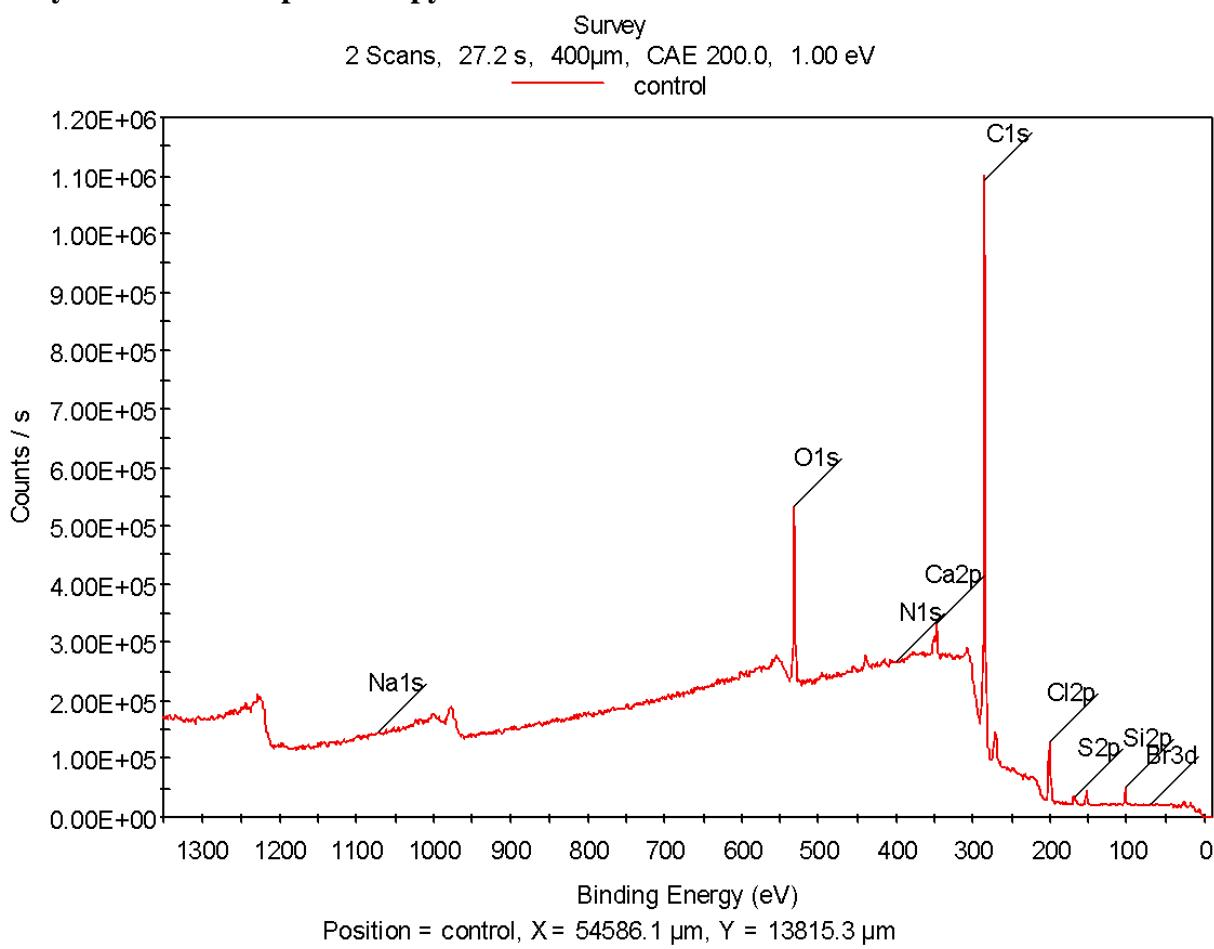
**Figure S 1.** Control (untreated) CPVC XPS survey data.
