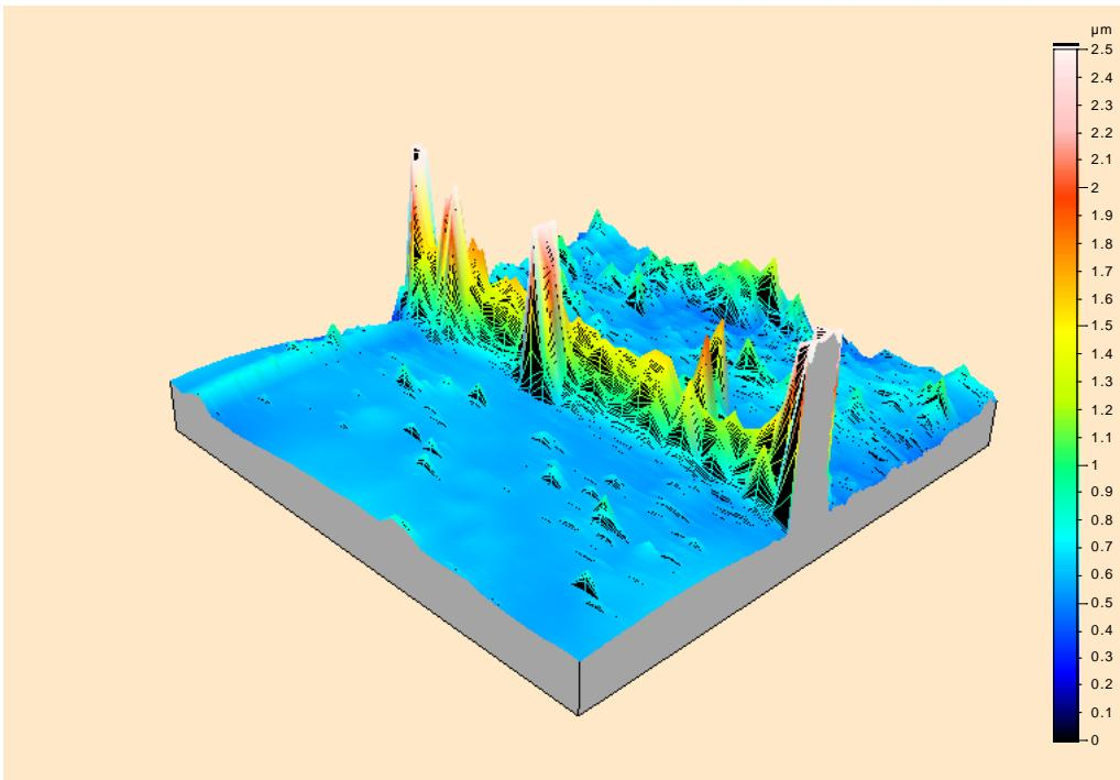
**Figure S 15.** SP profile scan of a polycarbonate (PC) surface partially treated with **6a**.
