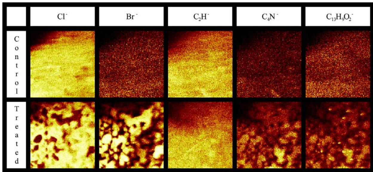
**Figure S 11.** Composite negative ion ToF-SIMS image of  $500.0 \times 500.0 \mu\text{m}$  section of control and **3a** treated samples. Intensity is a function of fragment quantity during analysis. Images correspond to negative ionic fragmentation products of chlorine ( $\text{Cl}^-$ ), bromine ( $\text{Br}^-$ ), ethane ( $\text{C}_2\text{H}^-$ ), tetracarbonyl ammonium ( $\text{C}_4\text{N}^-$ ), and hydroxybenzophenone ( $\text{C}_{13}\text{H}_9\text{O}_2^-$ ).
