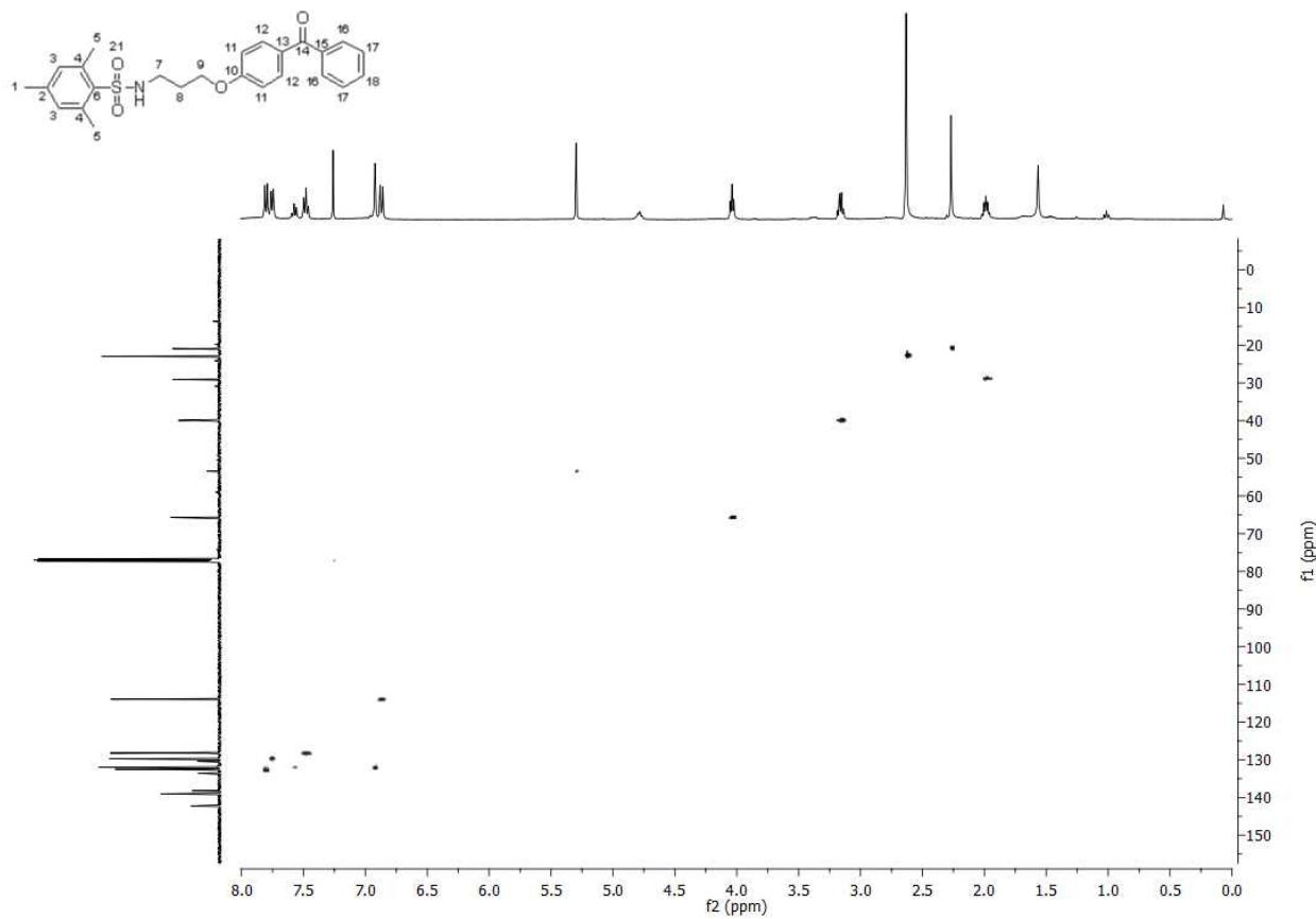
**Figure S 60.** HSQC 2D NMR ( $\text{CDCl}_3$ ) spectrum of **10**.
