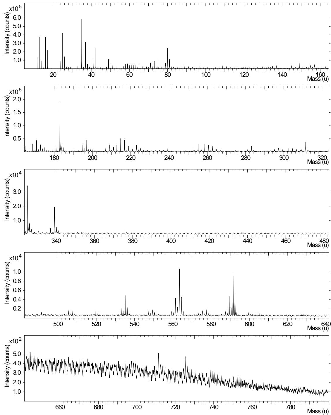
**Figure S 9.** Negative ion ToF-SIMS survey of control CPVC material.
