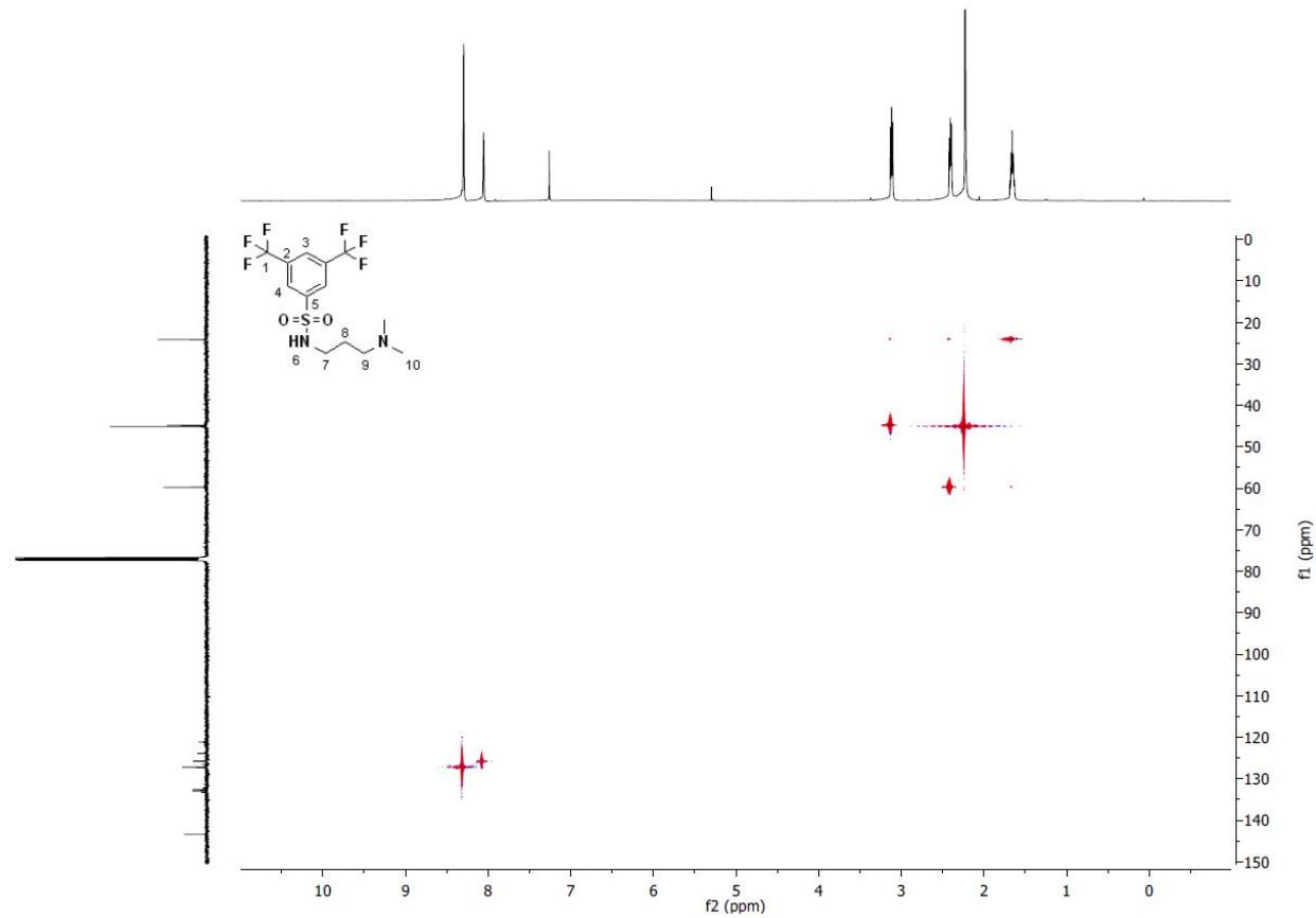
**Figure S 44.** HSQC 2D NMR (CDCl<sub>3</sub>) spectrum of **6**.
