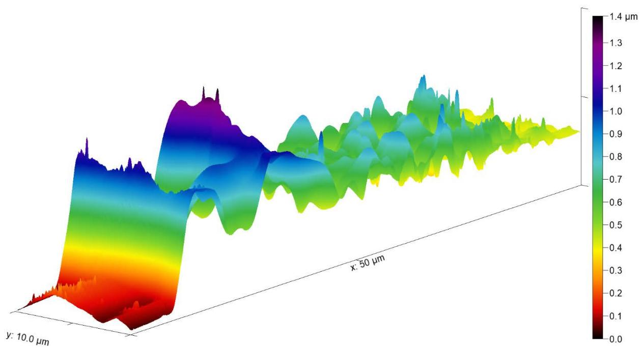
**Figure S 13.** Tapping AFM profile scan of a polycarbonate (PC) surface partially treated with **6a**.
