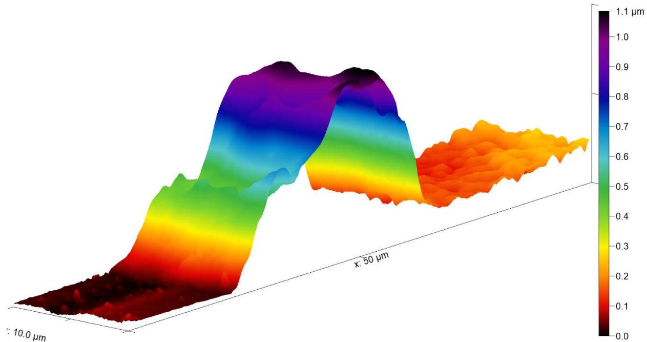
**Figure S 12.** Contact AFM profile scan of a polycarbonate (PC) surface partially treated with **3a**.
