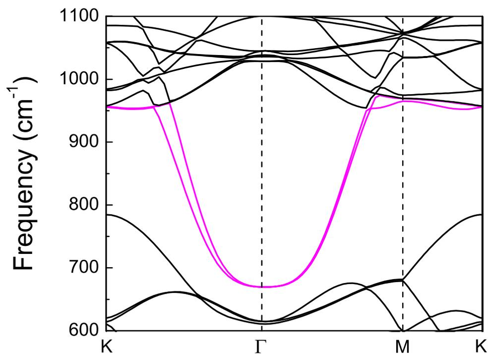
**Figure S6.** Phonon dispersion of 12.5 % hole-doped phase- $\alpha$  graphane under ambient pressure based on the ideal uniform hole doping model by removing electrons from graphane. The softened phonon branches at  $\Gamma$  point induced by the nesting in fermi surface are shown in pink.
