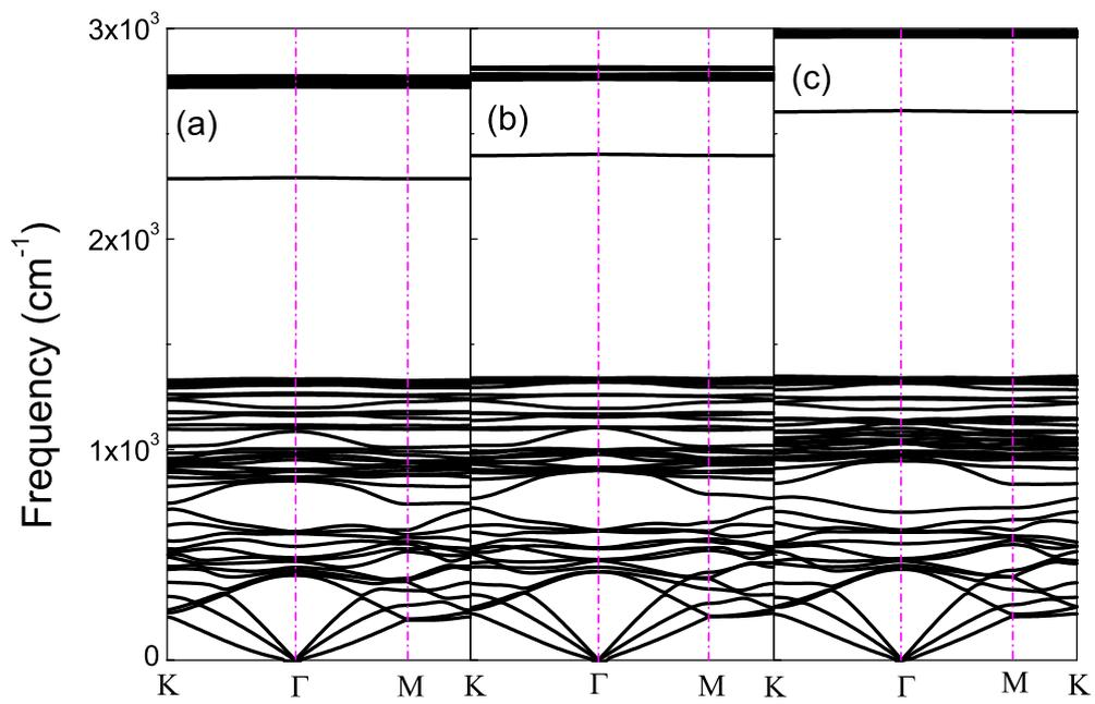
**Figure S5.** (a), (b), and (c) show the phonon dispersions of phase- $\alpha$  at 5 GPa, 10 GPa, and 200 GPa, respectively.
