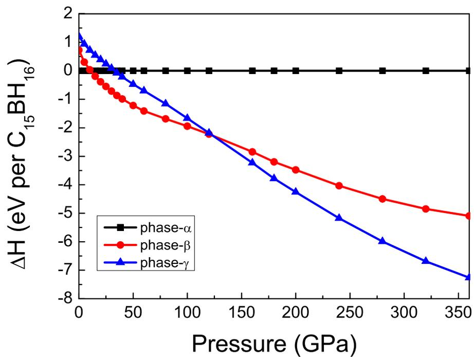
**Figure S2.** Calculated enthalpies of 6.125 mol% B dopant graphene as a function of pressure in phase- $\alpha$ , phase- $\beta$ , and phase- $\gamma$ , and phase- $\alpha$  is taken as a reference.
