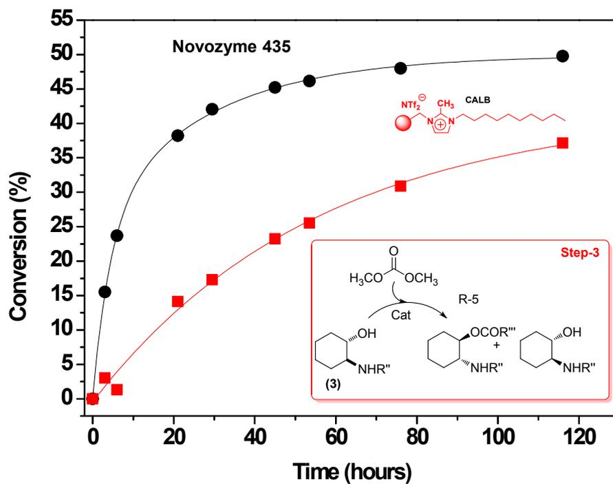
**Fig. SI.4.** Kinetic resolution of *trans*-2-phenylamine cyclohexanol (*rac*-4a) in DMC (0.1 M) as the solvent and acylating agent, under batch conditions, at 50 °C, 250 rpm. ●: 50 mg of Novozyme 435. ■: 50 mg of cat-2.
