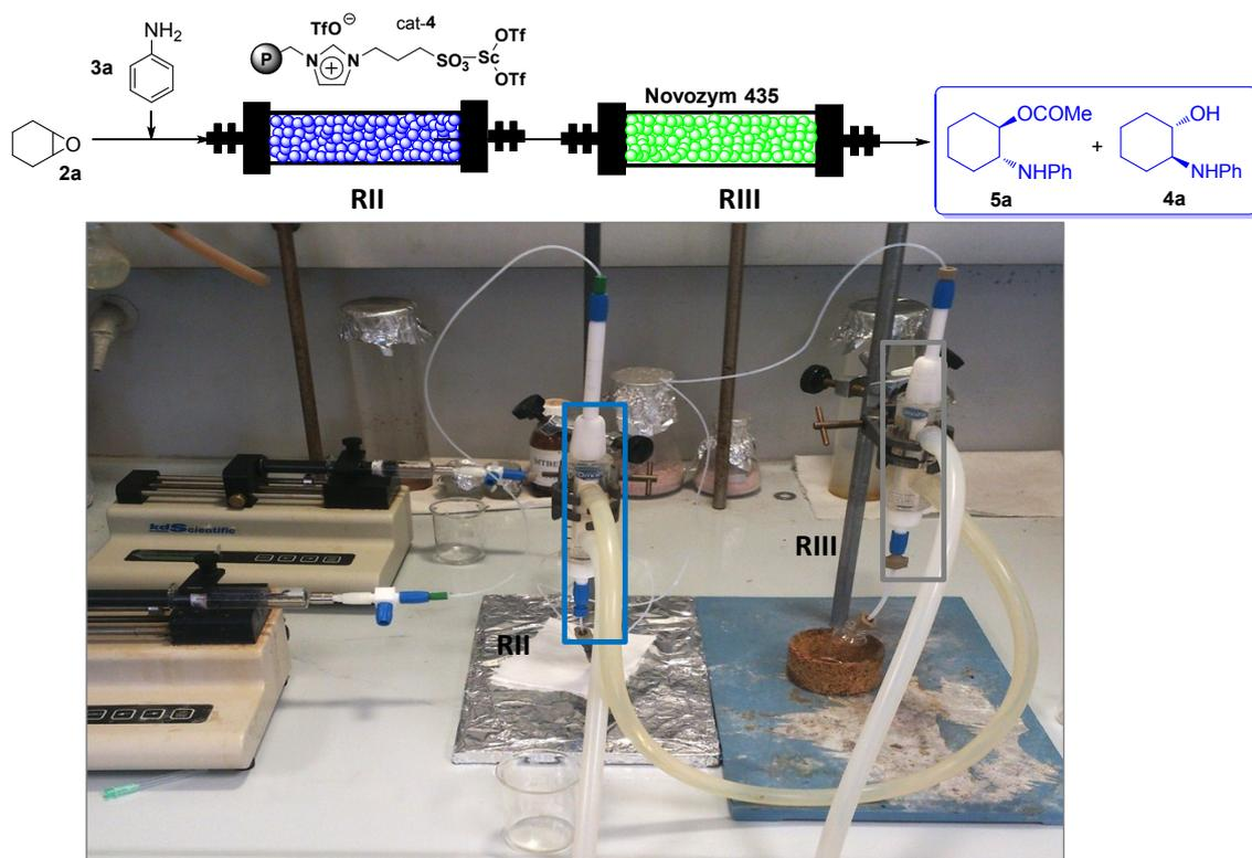
**Fig. SI.5.** Experimental set-up for the coupling of steps 2 and 3: ring opening of the cyclohexene oxide (**2a**) and kinetic resolution of the *trans*-2-phenylamine cyclohexanol (*rac*-**4a**).
