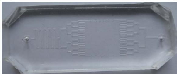
**Figure ESI-9.** Glass slide with hexagonally patterned hydrogel dots covered by the PDMS-mold with microfluidic chamber reactor.
