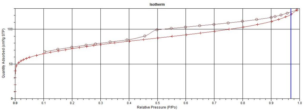
The adsorption-desorption isotherm of Pd/GNP CO
