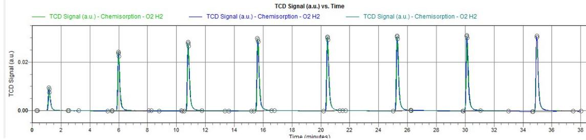
Chemisorption result of Pd/ NiGCNT BM sample, the surface area of Pd is, the estimated Pd nanoparticle size is around 11 nm. The surface area of the metal is 36 m<sup>2</sup>/g.
