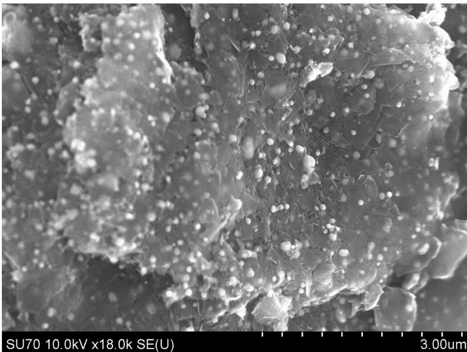
Figure S6 Ni/GNP produced by ball milling and microwave irradiation in a water bath. Large Ni nanoparticles on graphene were generated. No carbon nanotube was synthesized.
