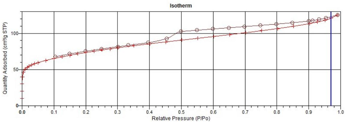
The adsorption-desorption isotherm of GNP BM KMW 2 MIN
