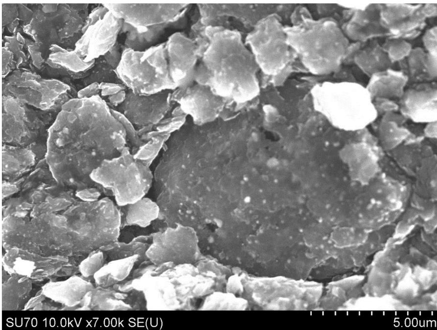
Figure S5 Ni/AC produced by ball milling and 1100 W fix power microwave irradiation. No carbon nanotube was generated.
