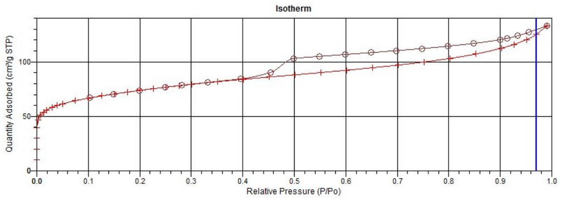
The adsorption-desorption isotherm of Pd/NiGCNT CO
