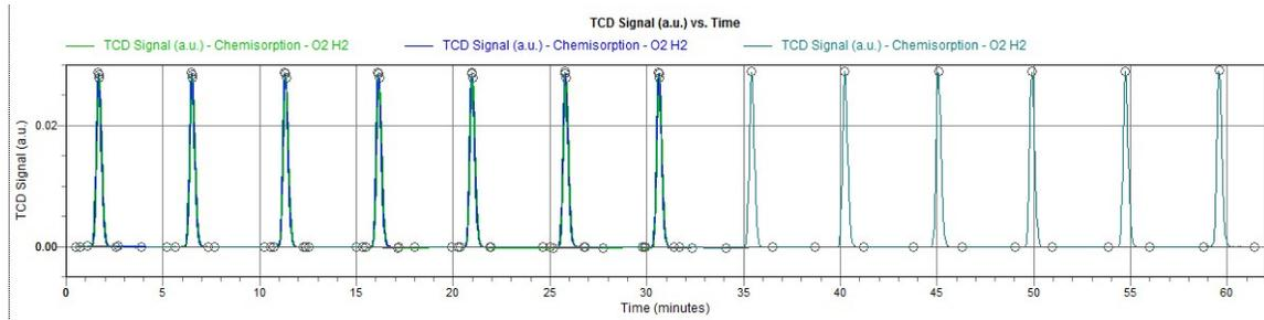
Chemisorption of the NiGCNT which shows no H<sub>2</sub> uptake for Ni NPs under the test condition.
