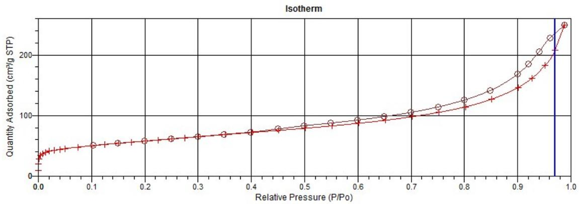
The adsorption-desorption isotherm of Ni/GNP BM
