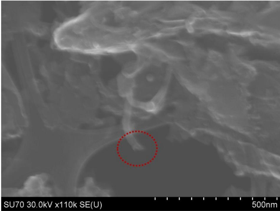
Figure S7 SEM image shows CNT has been broken by the second ball milling process
