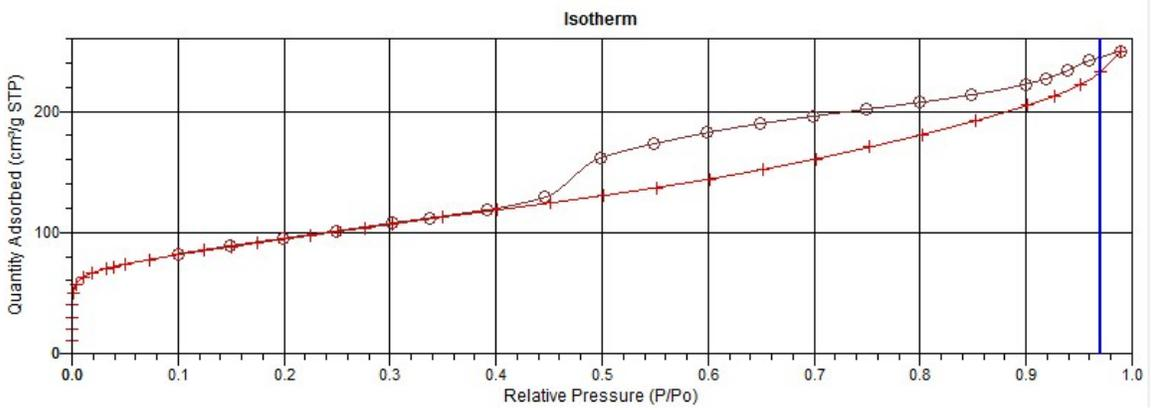
The adsorption-desorption isotherm of GNP BM
