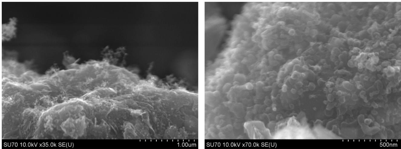
Figure S4 Graphene is coated by small fragments of carbon nanotube/GNP. The exact cause of the coating process is still unknown.
