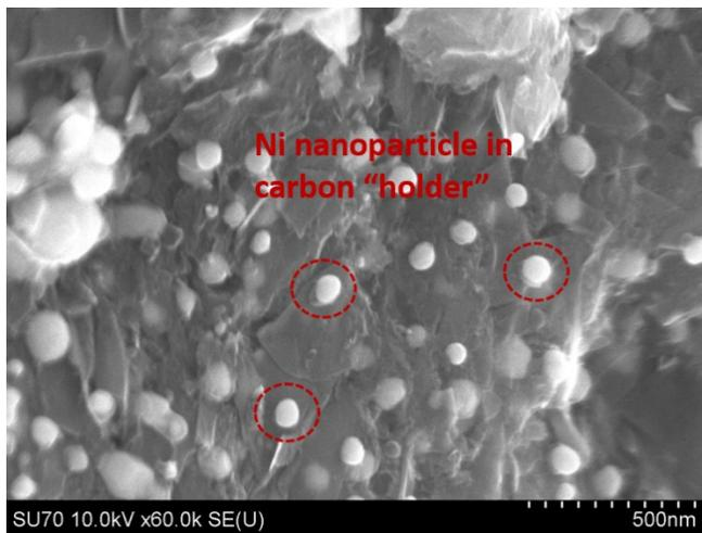
Figure S2 Bare Ni nanoparticles sit in carbon "holder". SEM images of NiGCNT 3 mins is shown. Some Ni nanoparticles are not successfully induced the growth of carbon nanotube. However, some bare Ni nanoparticle were partially coated with carbon which demonstrates the initial state of the growth process.
