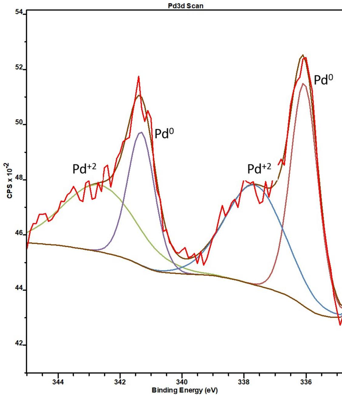
Figure S8 Pd 3d XPS spectrum of Pd/NiGCNT BM. Pd<sup>+2</sup> content in Pd/NiGCNT BM is higher than that in Pd/NiGCNT CO sample presented in Figure 2 (E).
