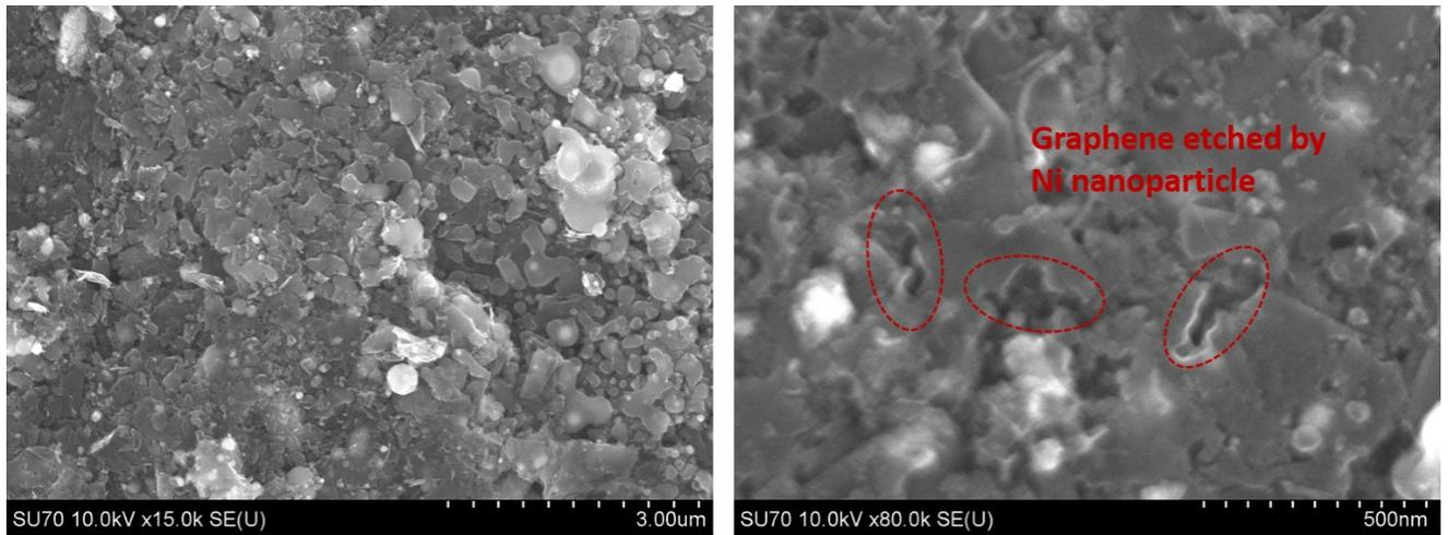
Figure S3 Graphene etched by Ni nanoparticles during the microwave process. The consumed carbon in the graphene is thought to be the source of carbon to grow carbon nanotube.
