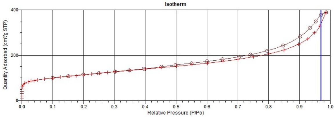
The adsorption-desorption isotherm of Pd/NiGCNT BM
