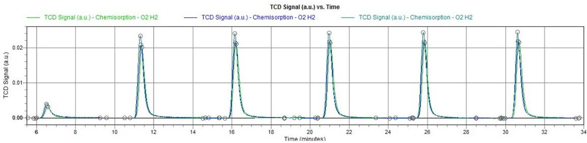
Chemisorption result of Pd/ NiGCNT CO sample, the surface area of Pd is, the estimated Pd nanoparticle size is around 18 nm. The surface area of the metal is 21 m<sup>2</sup>/g.
