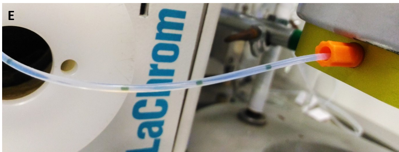
Figure S2. Key details of the system during operation: (A) The substrate solution and flow devices of steps 1 and 2. (B) The buffer flask BF1 and pump P3 . (C) Syringe pumps with the reagent solutions and reactor R2 . (D) Close-up of the biphasic mixture inside buffer flask BF2 . (E) Close-up of the biphasic stream exiting reactor R3/H .
