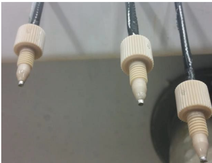
Figure S7: Assembled sensors ready to be implemented into the reactors. A two component epoxy resin was used to attach glass fibres in 1/16" stainless steel tubes which were further glued into HPLC fittings. The sensors were ready to use within the reactor after application of indicator and protection coating.
