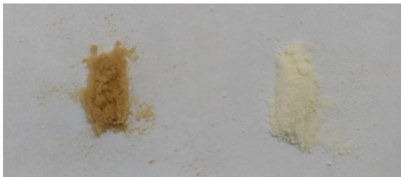
ESI Figure 2.3: Images of resin prior to regeneration (left) and post-regeneration (right)
