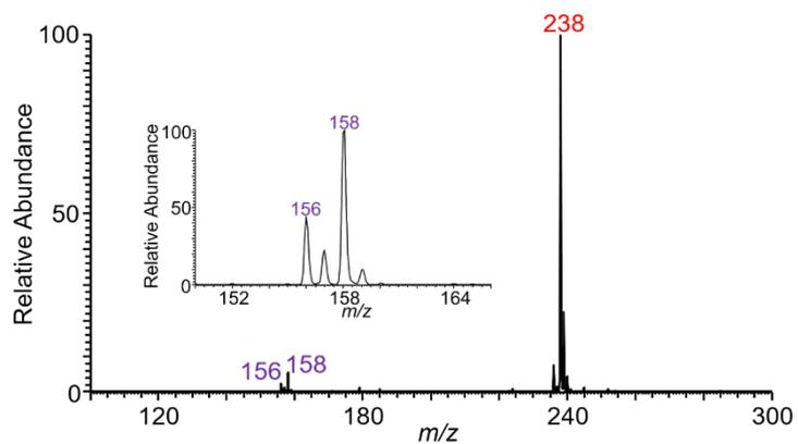
**Figure S24.** The nESI MS mass spectrum of the electrooxidation of 2-(4-methoxyphenyl)-1,2,3,4-tetrahydroisoquinoline (10  $\mu$ M in ACN) with TEMPO (10 mol%) at 0.5 min. Inset is the enlarged mass spectrum in the range of  $m/z$  150 to 166.
