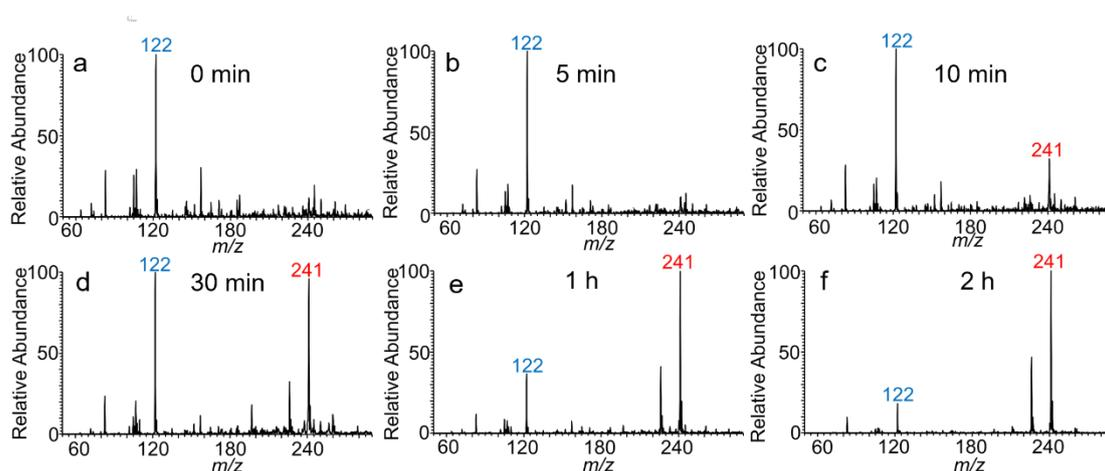
**Figure S6.** Use of the classical undivided electrolytic cell and mass spectrometry to monitor the progress of electrocatalytic oxidation of DMA ( $MW$  121 g/mol) to  $N,N,N',N'$ -tetramethylbenzidine (TMB,  $MW$  240 g/mol). Direct current 2 V was continuously applied to electrolyte ( $100 \mu\text{M}$ ) for 0 min (**a**), 5 min (**b**), 10 min (**c**), 30 min (**d**), 60 min (**e**) and 120 min (**f**), respectively.
