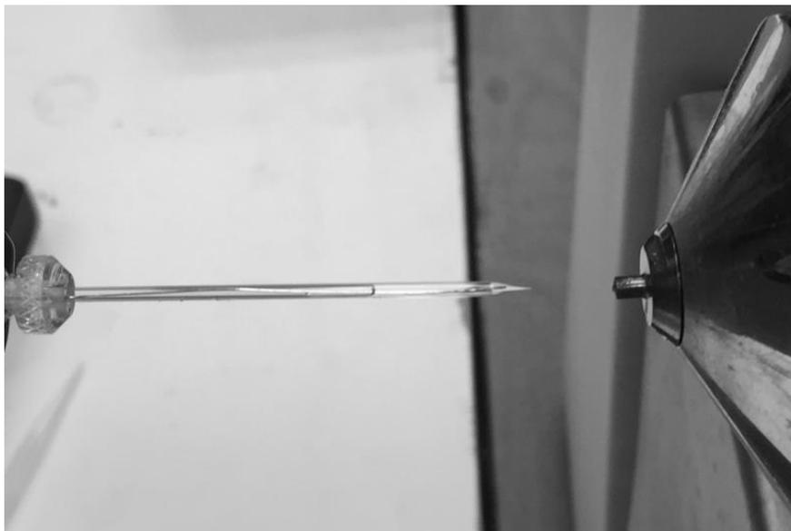
**Figure S1.** Experimental setup of the real time electrochemical reaction platform. The borosilicate glass capillary is used with O.D. = 1.5 mm and I.D. = 0.86 mm. The distance of Pt electrode away from the capillary tip is ~ 2 mm. 10  $\mu\text{L}$  sample was transferred into the capillary, the distance of sample liquid level to the capillary tip is about 1.6 cm. The distance between the capillary tip and MS inlet was kept at 0.8 cm. The diameter of Pt electrode is 0.2 mm.
