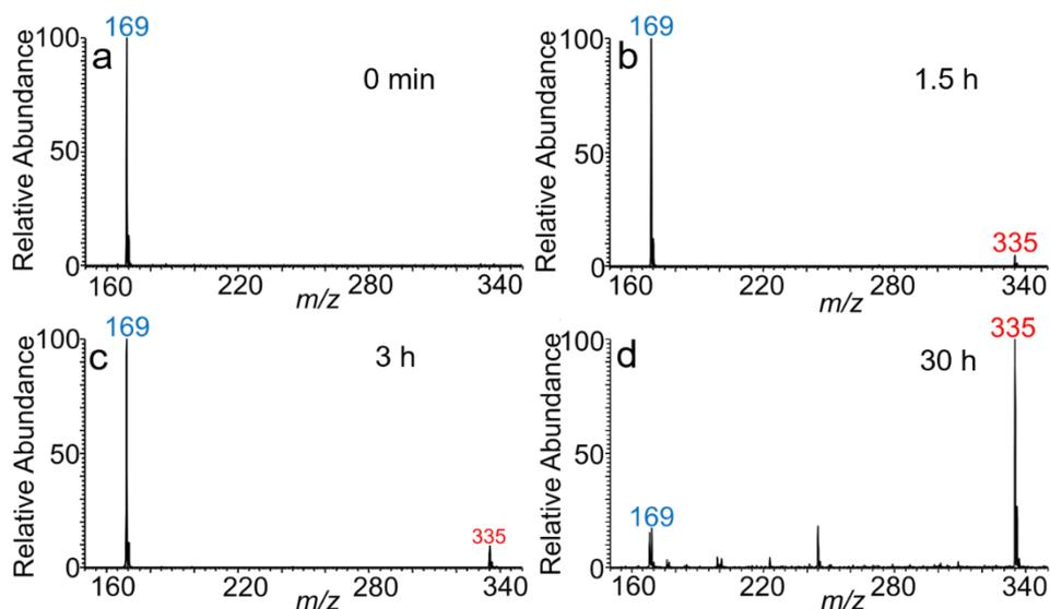
**Figure S10.** Use of the classical undivided electrolytic cell and mass spectrometry to monitor the progress of electrocatalytic oxidation of  $\beta$ -carbolines ( $MW$  168 g/mol) to its product **8** ( $MW$  334 g/mol). Direct current 2 V was continuously applied to  $\beta$ -carbolines (100  $\mu$ M) and tetraethylammonium perchlorate (100  $\mu$ M) solution for 0 min (**a**), 1.5 h (**b**), 3 h (**c**) and 30 h (**d**), respectively.
