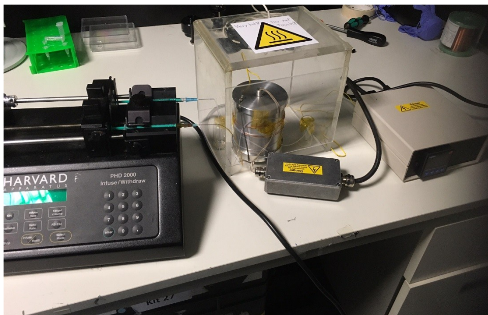
Figure S29. Photograph of the set-up used for the in flow synthesis showing syringe pump, solid state heater, around which the PTFE taped is wrapped, and PID controller.
