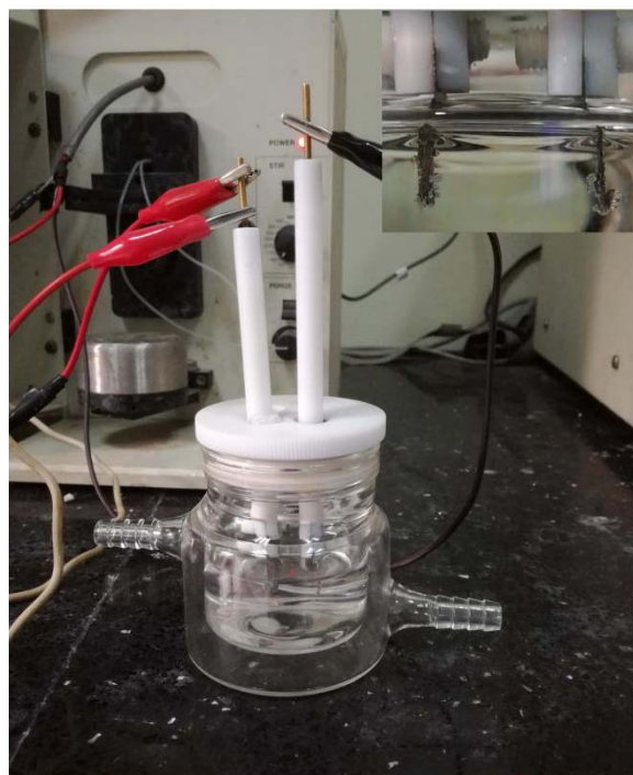
Figure S30. The photograph for overall water splitting reaction in a two-electrode configuration. The inset is an optical photograph showing the generation of \text{H}_2 and \text{O}_2 bubbles for PMo/ZIF-67-6-6N||PMo/ZIF-67-6-7N on Ni foam.
