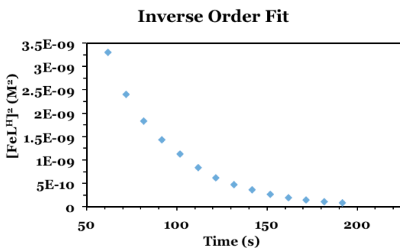
Figure S8. Representative plots (0.1 mM) for order determination of iron in \text{O}_2 reduction mechanism with 1^{\text{H}} in DMA. The iron concentration was varied (0.050 mM, 0.10 mM, 0.13 mM, 0.16 mM, 0.2 mM) and treated with 0.75 atm \text{O}_2 at 20 °C. Each concentration was repeated in triplicate and the linearized integrated rate expressions were plotted. The first order plot provided the best fit (shown upper left) with data from the five concentrations (shown upper right).
