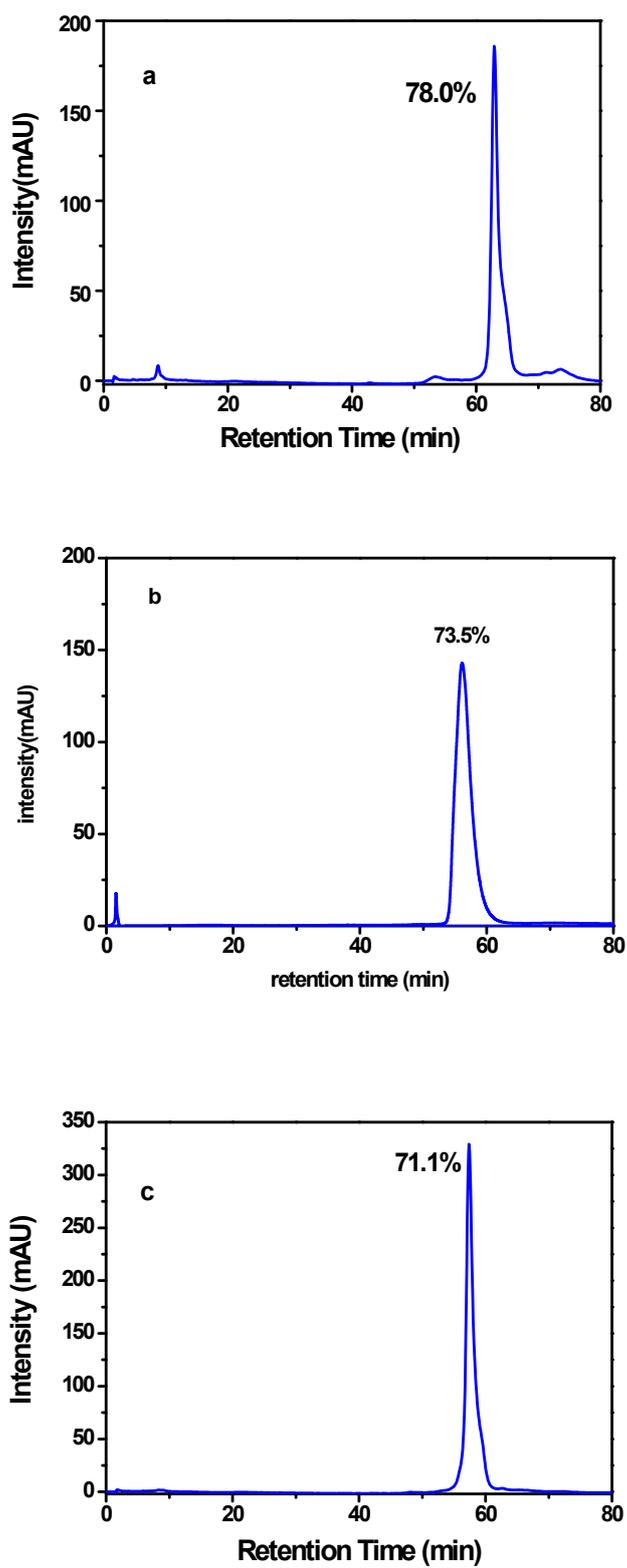
**Figure S5. RPC HPLC analysis of purified lipid-DNAs:** a. U4T; b. U4T28; c. CrU4T. Numbers beside the elution peaks represent the buffer B contents when lipid-DNAs were eluted.
