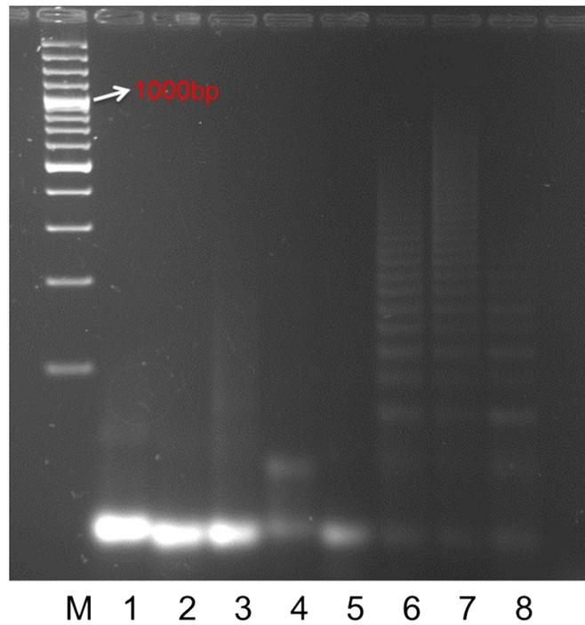
**Figure S9. Agarose gel electrophoresis analysis of DNA HCR.** Lane 1: M1; lane 2: M2; lane 3: M1+M2; lane 4: M1+U4T28; lane 5: M1+U4T28; lanes 6–8: three different molar ratios of initiator (1/1/1, 1/1/0.5, 1/1/2, M1/M2/U4T28).
