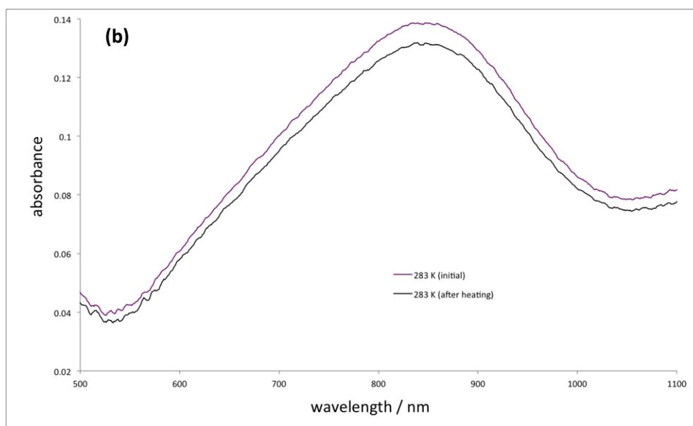
**Figure S13.** (a) Variable temperature UV-Vis spectra of  $[1]^+[\text{BAr}_4]^-$  taken under an atmosphere of  $\text{H}_2$  (1 atm.) are consistent with reversible release of  $\text{H}_2$  from  $[1 \cdot \text{H}_2]^+[\text{BAr}_4]^-$  to form  $[1]^+[\text{BAr}_4]^-$  (evidenced by the increasing absorption centred at 618 nm), as temperature is increased. (b) Partial decomposition at elevated temperature is evidenced by reduced absorption upon returning to low temperature.
