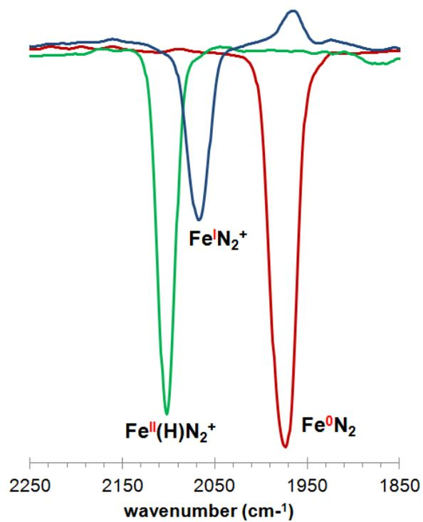
**Figure S9.** IR spectra of the  $\nu_{\text{NN}}$  region:  $1 \cdot \text{N}_2$  (red),  $[1 \cdot \text{N}_2]^+[\text{BAR}_4^{\text{F}}]^-$  (from  $[1]^+[\text{BAR}_4^{\text{F}}]^-$  in a glove-box under a  $\text{N}_2$  atmosphere; blue), and *trans*- $[\text{Fe}(\text{depe})_2(\text{H})(\text{N}_2)]^+[\text{BAR}_4^{\text{F}}]^-$  (green). All prepared as 0.1 M  $\text{Et}_2\text{O}$  solutions.
