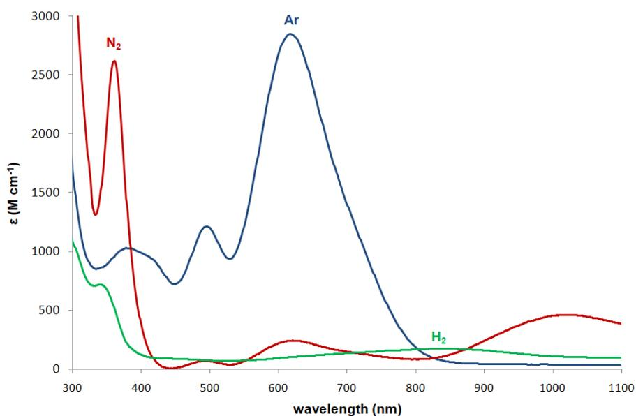
**Figure S10.** UV-vis spectra of  $[1]^+[\text{BARF}_4]^-$  under Ar (blue),  $\text{N}_2$  (red), and  $\text{H}_2$  (green) atmosphere in DFB (293 K, 1 atm.).
