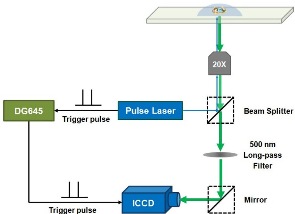
**Scheme S3.** Schematic diagram of time-gated transient microscope for fluorescence lifetime imaging.
