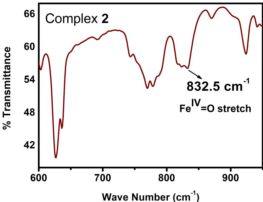
**Figure S17.** FT-IR spectra of complex **1** and **2**
