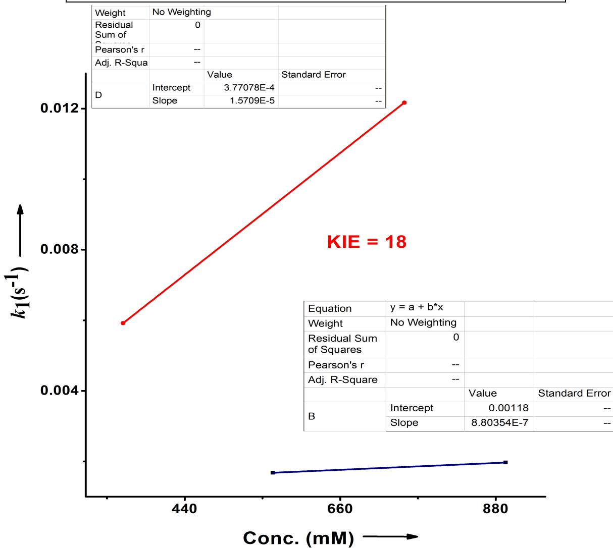
**Figure S36.** Kinetic isotope effect (KIE) study plot during  $sp^3$  C–H bromination
