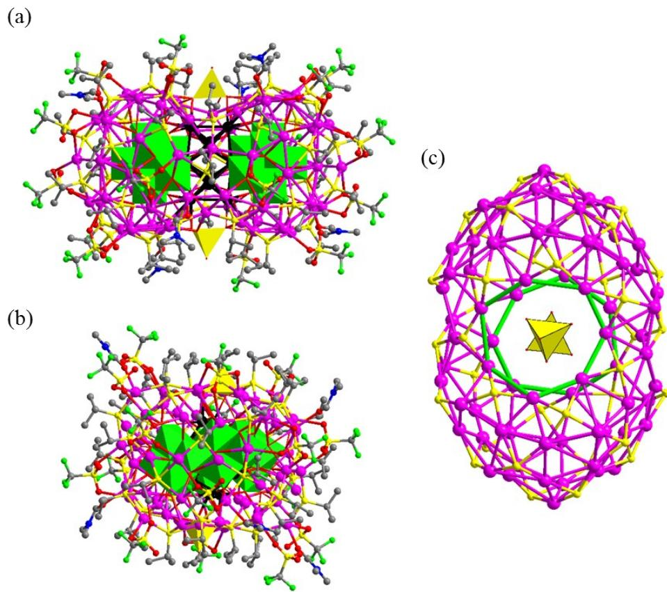
(a) and (b) The X-ray crystal structure of  $\text{Ag}_{10}@\text{(Mo}_7\text{O}_{26})_2@\text{Ag}_{70}$  nanocluster viewed along two orthogonal directions. The inner silver atoms of  $\text{Ag}_{10}$  kernel are highlighted by black. The  $\text{Mo}_7\text{O}_{26}^{10-}$  and  $\text{MoO}_4^{2-}$  are represented by green and yellow polyhedral, respectively. (c) The  $\text{Ag}_{70}\text{S}_{36}$  shell with silver heptagons highlighted by green.
