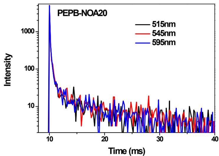
**Fig. S21** Transient luminescence decays of PEPB-NTA20 and PEPB-NOA20 powders measured at different emission peaks.
