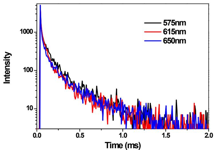
**Fig. S19** Transient luminescence decays of PEPB-NTA100 film measured at different emission peaks.
