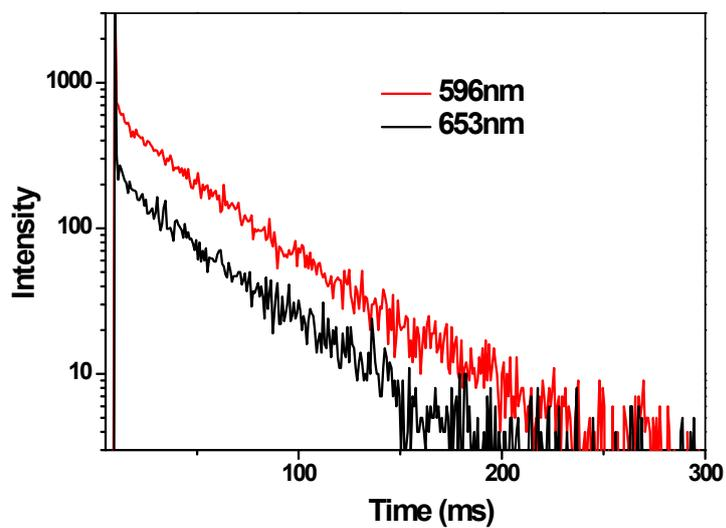
**Fig. S8** Transient luminescence decays of PEPC-NIA22 film measured at different emission peaks.
