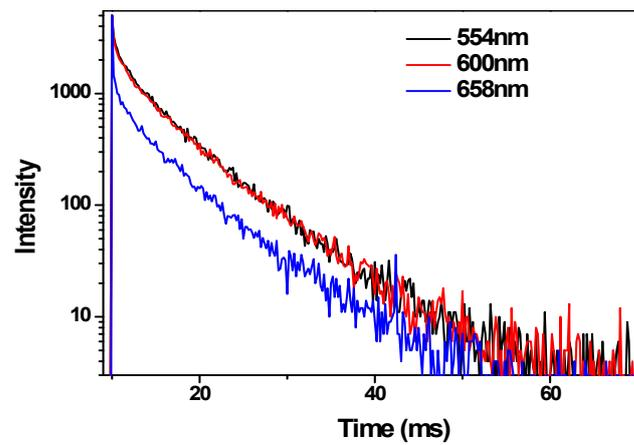
**Fig. S2** Transient luminescence decays of PEPB-NIA5 film measured at different emission peaks.
