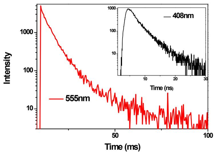
**Fig. S12** Transient luminescence decays of PEPB-NIA5 powder measured at different emission peaks.
