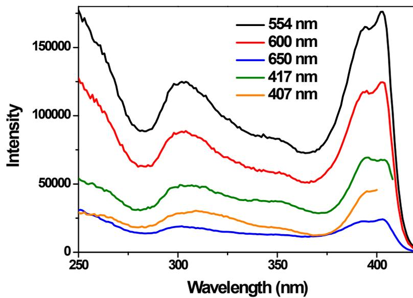
**Fig. S5** Excitation spectra of PEPB-NIA22 film measured at different emission peaks.
