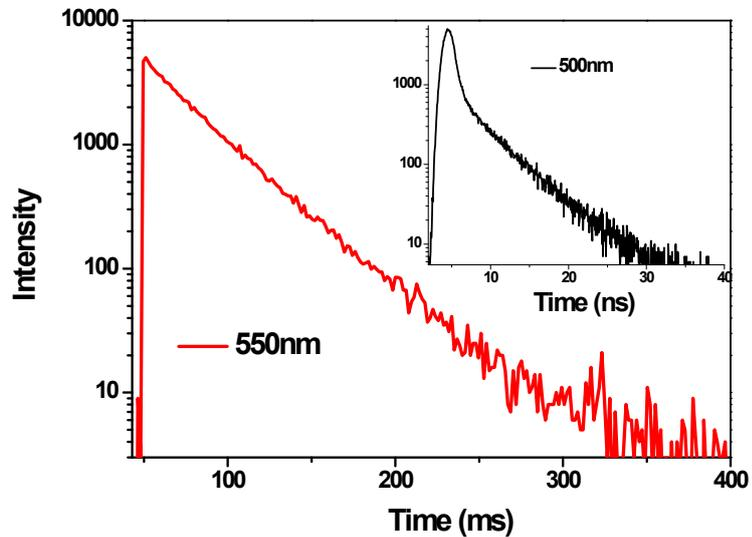
**Fig. S15** Transient luminescence decays of PEPC-NIA5 powder measured at different emission peaks.
