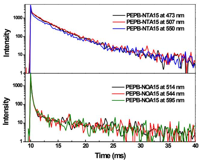
**Fig. S20** Transient luminescence decays of PEPB-NTA15 and PEPB-NOA15 film measured at different emission peaks.
