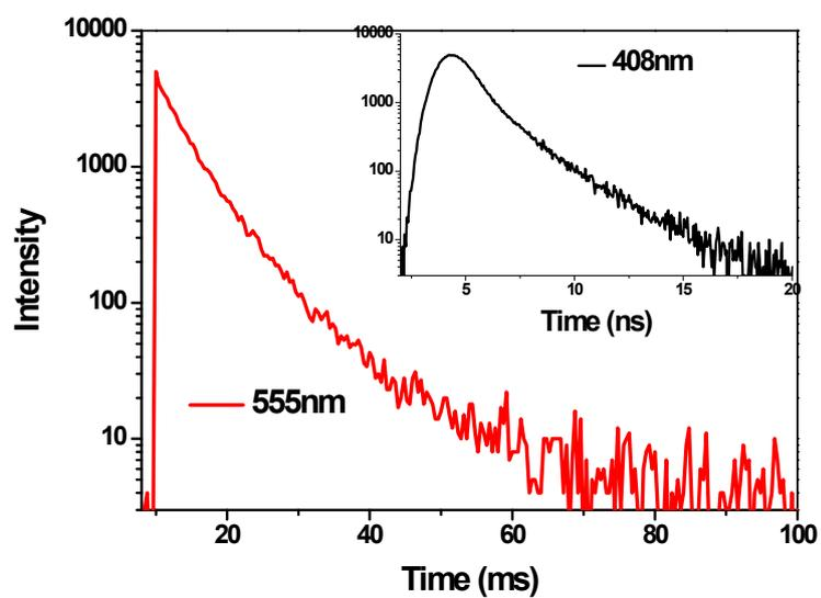
**Fig. S14** Transient luminescence decays of PEPB-NIA20 powder measured at different emission peaks.
