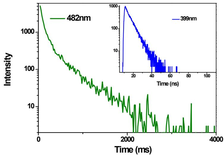
**Fig. S22** Transient luminescence decays of PEPC-NAA5 powder measured at different emission peaks.
