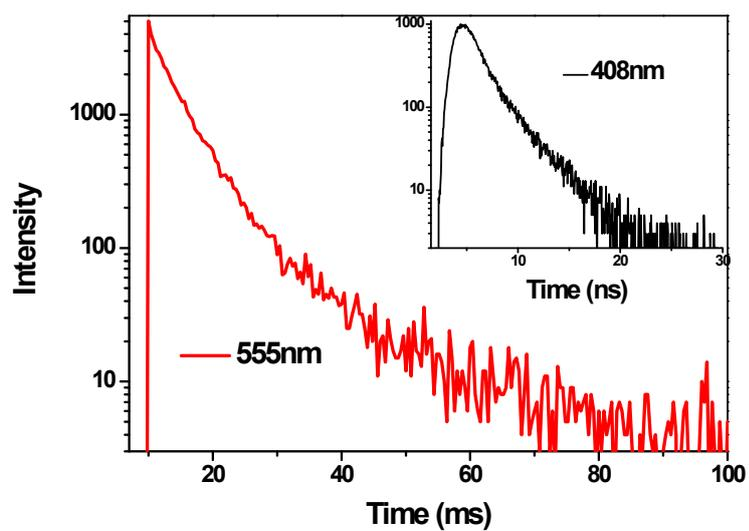
**Fig. S13** Transient luminescence decays of PEPB-NIA10 powder measured at different emission peaks.
