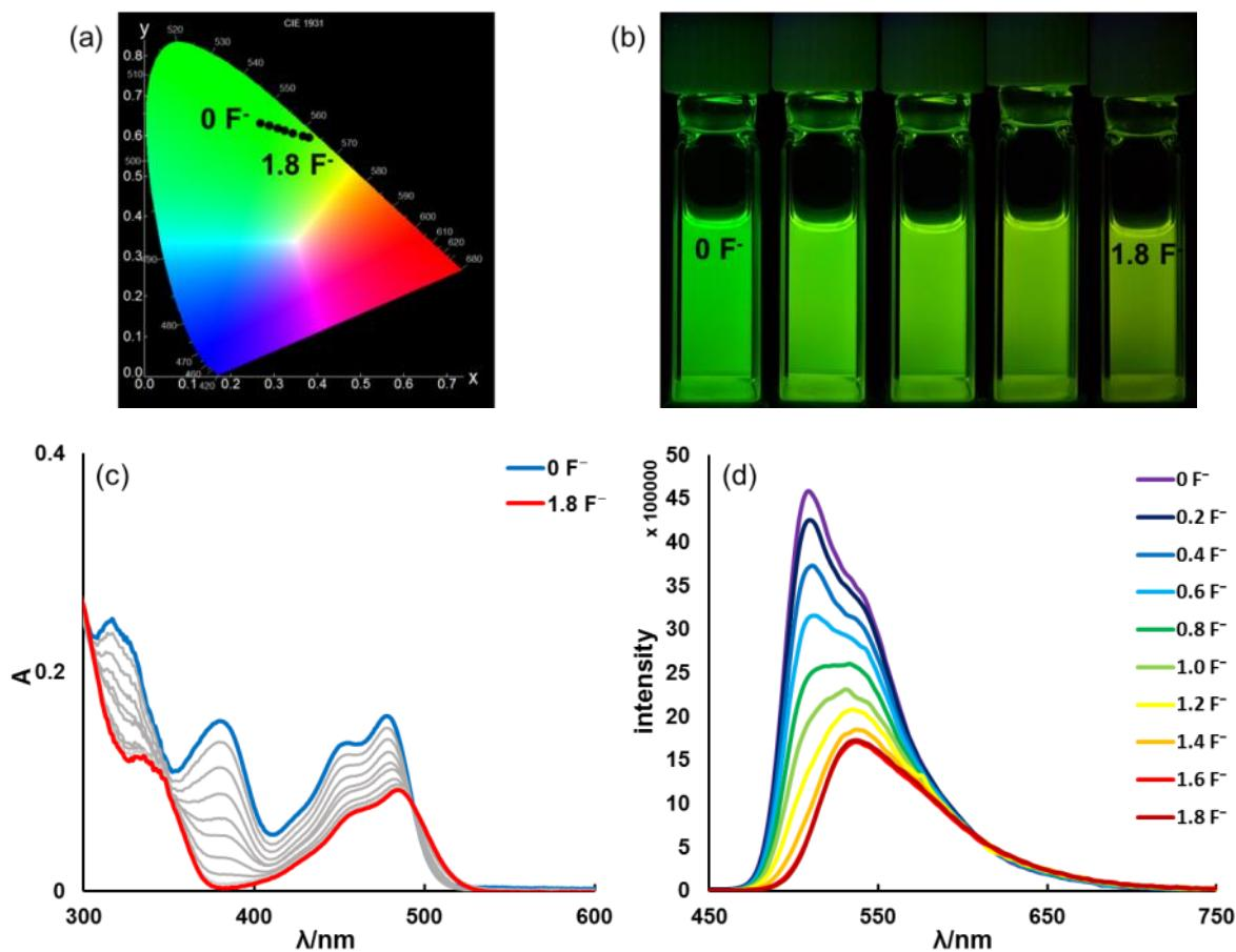
**Figure S16.** (a): CIE coordinates (CIE 1931). (b): Photographs of the solutions. (c): The UV-Vis titration spectra, (d): Fluorescent titration spectra of **1a** ( $c = 1 \times 10^{-5}\text{ M}$ ,  $\lambda_{\text{ex}} = 320\text{ nm}$ , under air) by TBAF in THF at 298 K.
