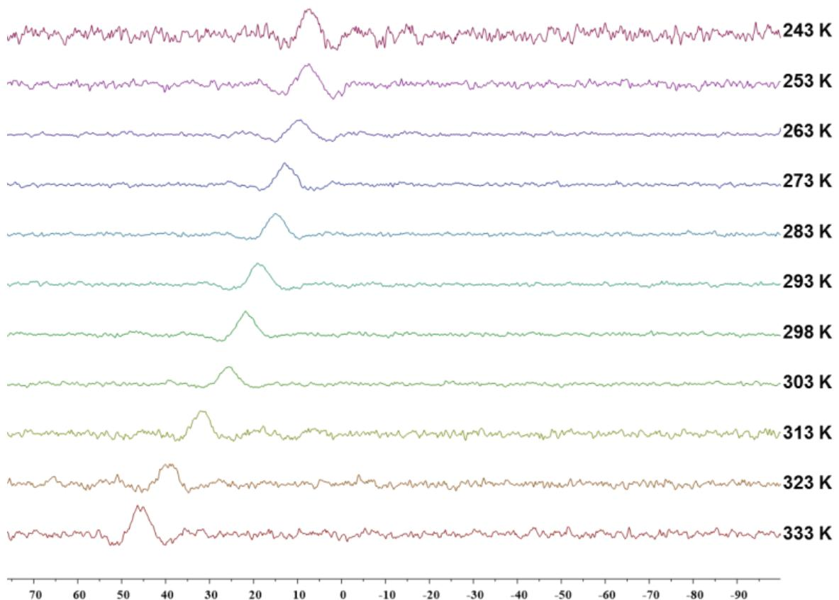
**Figure S92:** <sup>11</sup>B NMR spectral change of **2a** with temperature in CDCl<sub>3</sub>.
