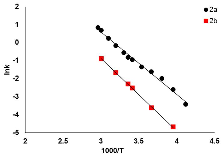
**Figure S29:** The  $\ln K$  vs.  $T^{-1}$  (kelvin) plots and fittings for **2a** and **2b**, using variable temperature  $^{11}\text{B}$  NMR data for the determination of  $\Delta H$  and  $\Delta S$  ( $\Delta H = 28.77 \text{ kJ/mol}$  for **2a**;  $33.5 \text{ kJ/mol}$  for **2b**,  $\Delta S = 91 \text{ J/mol/K}$  for **2a**;  $93 \text{ J/mol/K}$  for **2b**).
