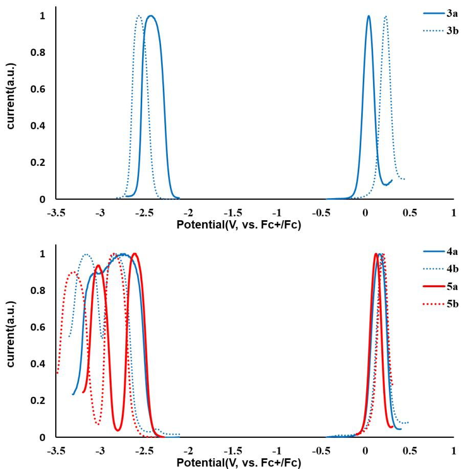
**Figure S27:** DPV diagrams of **3a/3b-5a/5b** showing the oxidation/ reduction waves (scan rate = 100 mV/s, using 0.1 M of [NBu<sub>4</sub>]PF<sub>6</sub> as the electrolyte, recorded in CH<sub>2</sub>Cl<sub>2</sub> (oxidation), and THF (reduction)).
