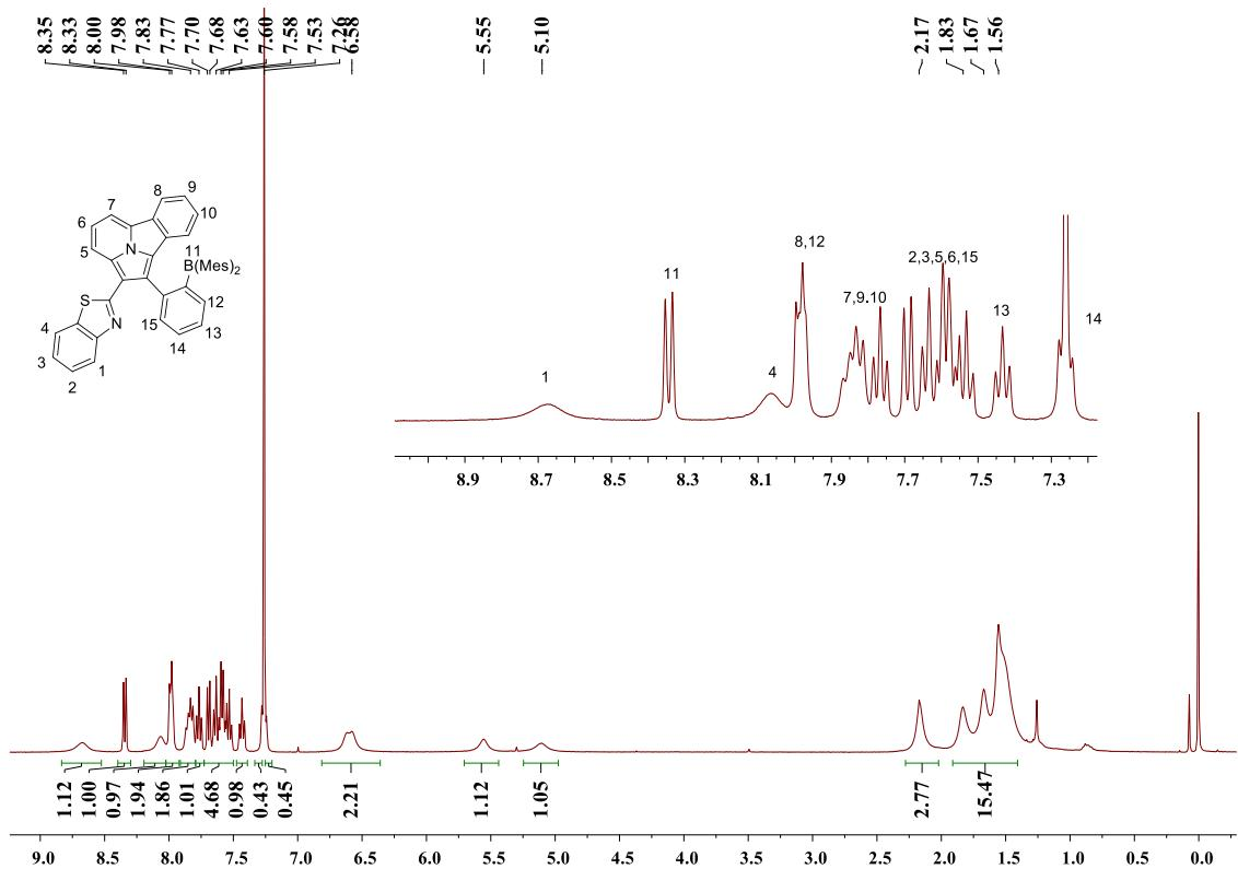
**Figure S81:**  $^1\text{H}$  NMR spectrum of compound **4b** in  $\text{CDCl}_3$
