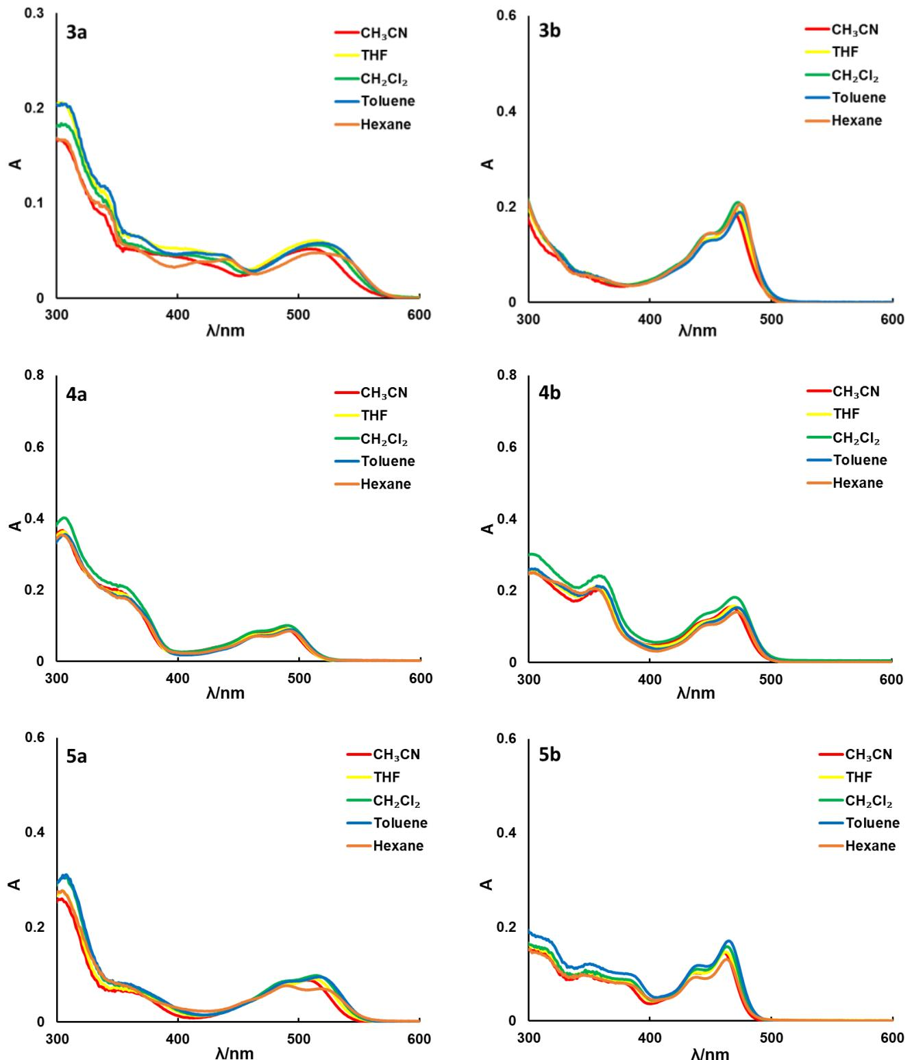
**Figure S4:** UV-vis Spectra of Compounds 3a/3b-5a/5b in Different Solvents ( $c = 1 \times 10^{-5} \text{ mol/L}$ ).
