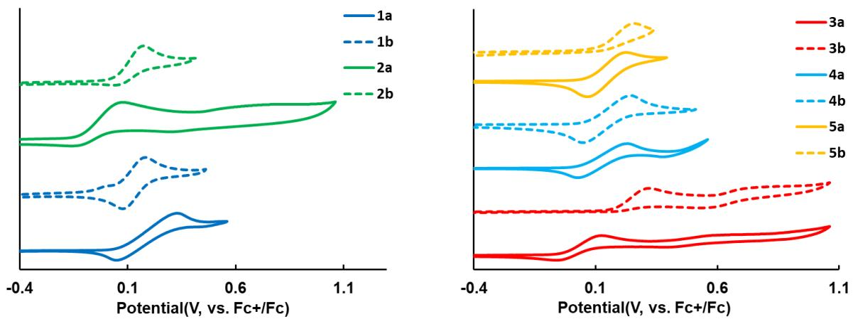
**Figure S28:** CV diagrams of **1a/1b-5a/5b** showing the oxidation waves at 50 mV/s with 0.1 M of  $[\text{NBu}_4]\text{PF}_6$  as the electrolyte in  $\text{CH}_2\text{Cl}_2$ .
