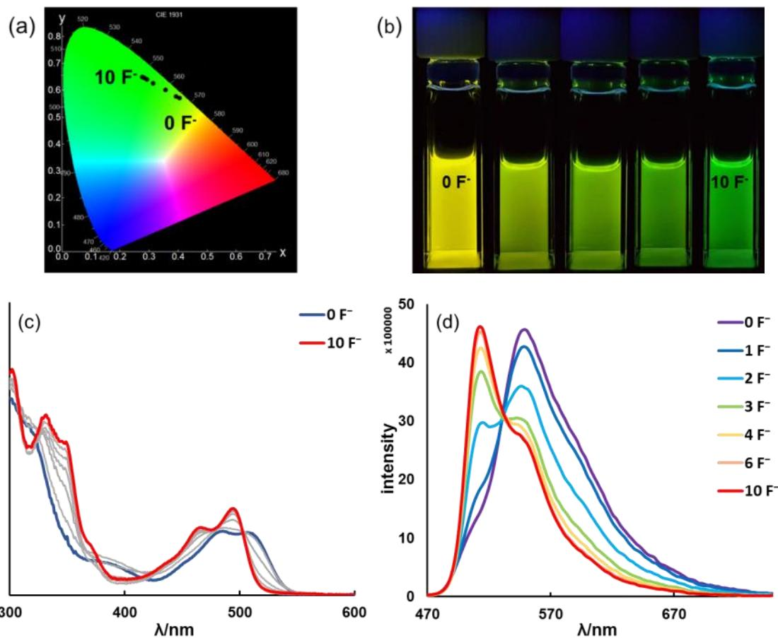
**Figure S18.** (a): CIE coordinates (CIE 1931). (b): Photographs of the solutions. (c): The UV-Vis titration spectra, and (d): Fluorescent titration spectra of **2a** ( $c = 1 \times 10^{-5}\text{ M}$ ,  $\lambda_{\text{ex}} = 320\text{ nm}$ , under air) by TBAF in THF at 298 K.
