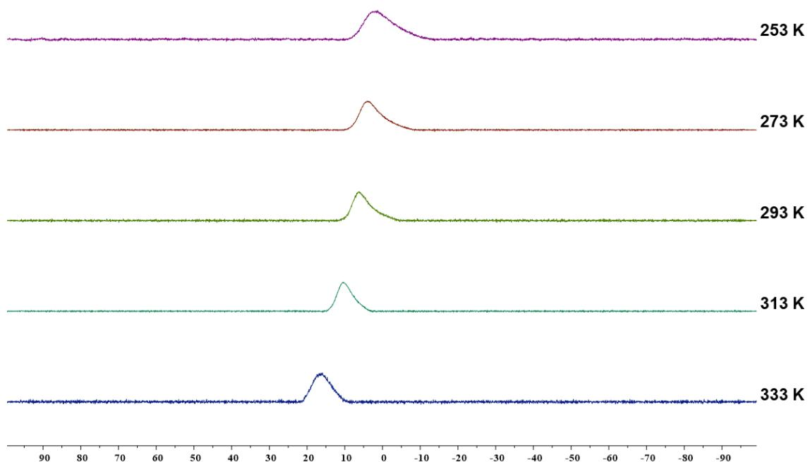
**Figure S99:**  $^{11}\text{B}$  NMR spectral change of **5a** with temperature in  $\text{CDCl}_3$ .
