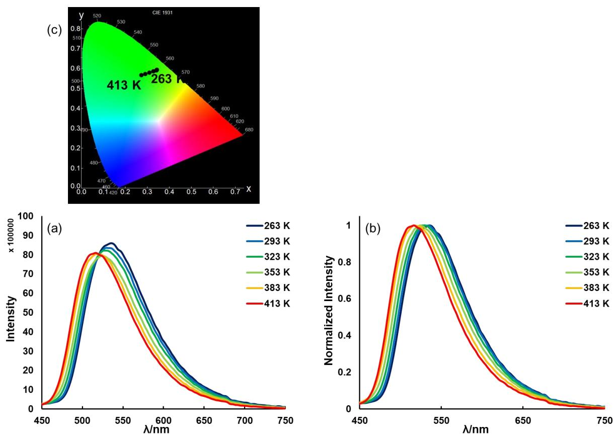
**Figure S13:** (a) CIE coordinates (CIE 1931) of **3b**. (b) Emission spectra, and (c) Normalized emission spectra of **3a** recorded between 263 K and 413 K ( $c = 1 \times 10^{-5}$  M, in mesitylene,  $\lambda_{\text{ex}} = 360$  nm, under  $\text{N}_2$ )
