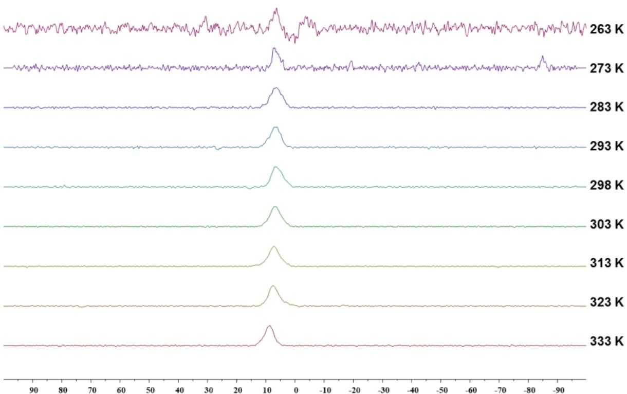
**Figure S96:** <sup>11</sup>B NMR spectral change of **3a** with temperature in CDCl<sub>3</sub>.
