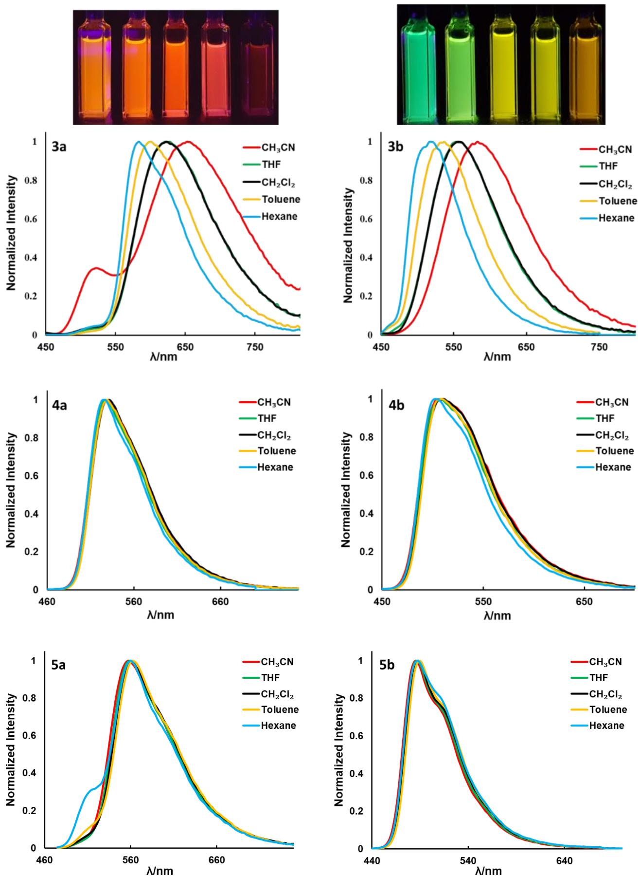
**Figure S6:** Fluorescence Spectra of Compounds 3a/3b-5a/5b in Different Solvents ( $c = 1 \times 10^{-5} \text{ mol/L}$ ).
