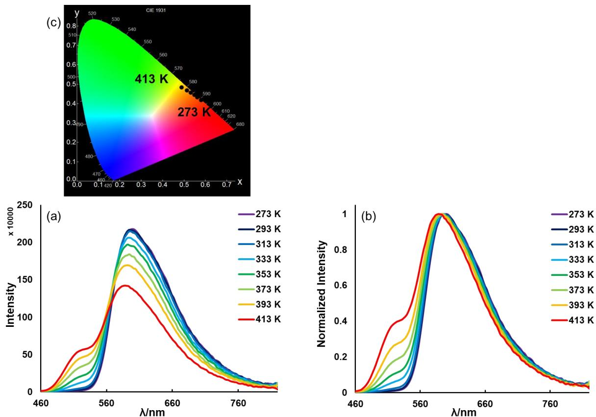
**Figure S12:** (a) CIE coordinates (CIE 1931) of **3a**. (b) Emission spectra, and (c) Normalized emission spectra of **3a** recorded between 273 K and 413 K ( $c = 1 \times 10^{-5}$  M, in mesitylene,  $\lambda_{\text{ex}} = 370$  nm, under N<sub>2</sub>)
