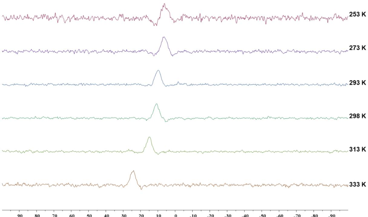
**Figure S94:** <sup>11</sup>B NMR spectral change of **2b** with temperature in CDCl<sub>3</sub>.
