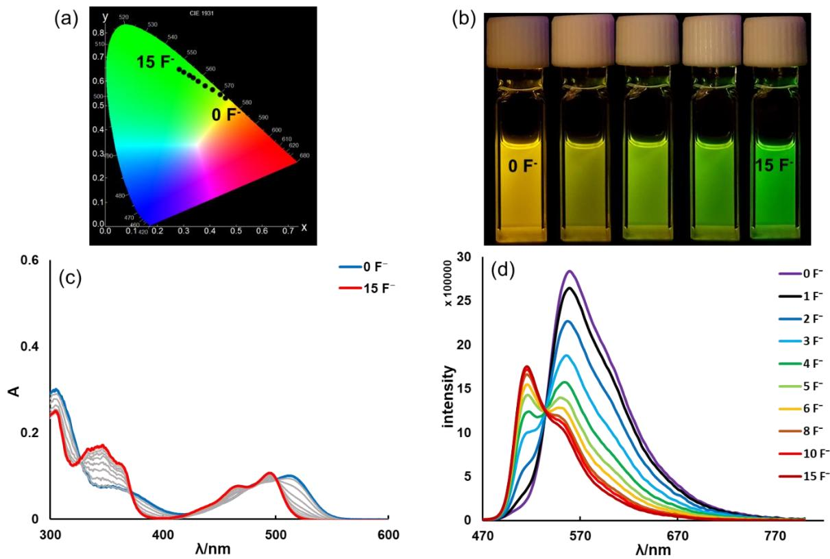
**Figure S24.** (a): CIE coordinates (CIE 1931). (b): Photographs of the solutions. (c): The UV-Vis titration spectra, and (d): Fluorescent titration spectra of **5a** ( $c = 1 \times 10^{-5}$  M,  $\lambda_{\text{ex}} = 320$  nm, under air) by TBAF in THF at 298 K.
