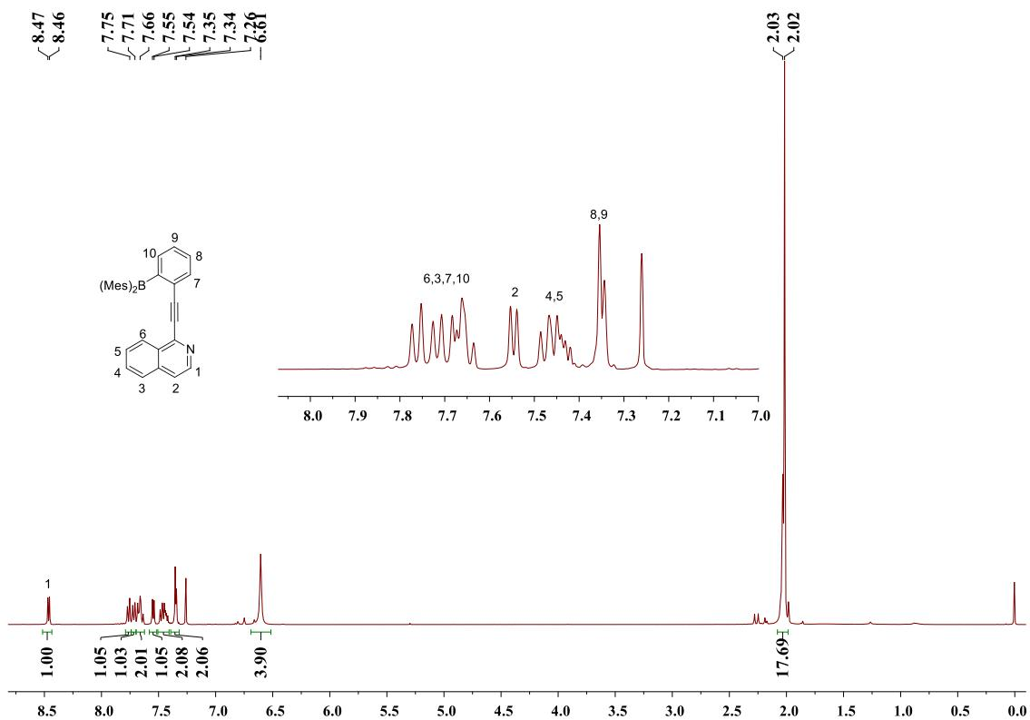
**Figure S69:**  $^1\text{H}$  NMR spectrum of compound **3** in  $\text{CDCl}_3$
