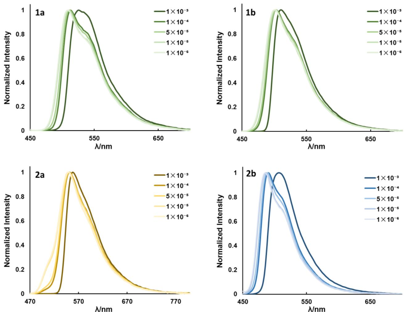
Figure S7: Fluorescence Spectra of Compounds **1a/1b-2a/2b** at different concentrations of THF solution.
