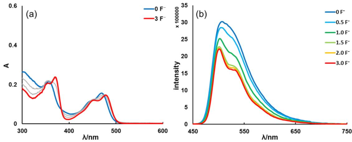
**Figure S23:** (a): The UV-Vis titration spectra, and (b): Fluorescent titration spectra of **4b** ( $c = 1 \times 10^{-5}$  M,  $\lambda_{\text{ex}} = 320$  nm, under air) by TBAF in THF at 298 K.
