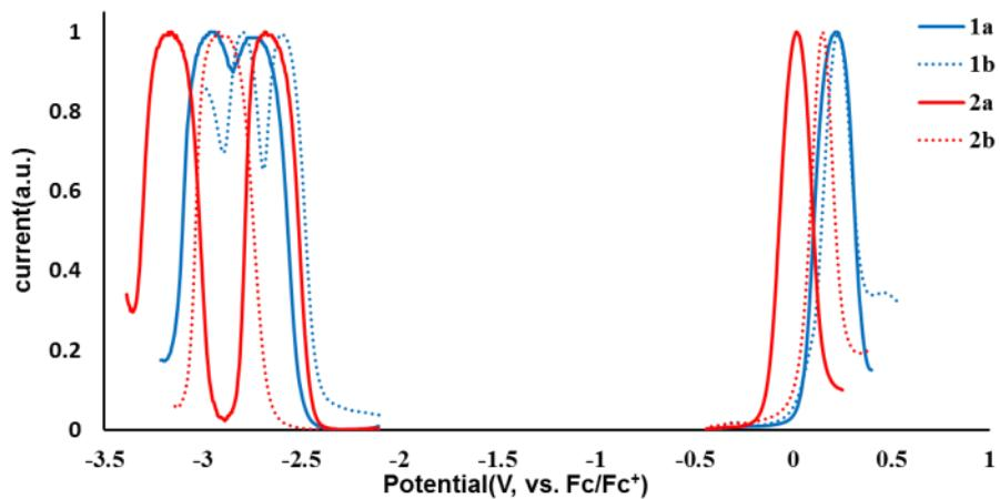
**Figure S26:** DPV diagrams of **1a/1b-2a/2b** showing the oxidation/ reduction waves (scan rate = 100 mV/s, using 0.1 M of [NBu<sub>4</sub>]PF<sub>6</sub> as the electrolyte, recorded in CH<sub>2</sub>Cl<sub>2</sub> (oxidation), and THF (reduction)).
