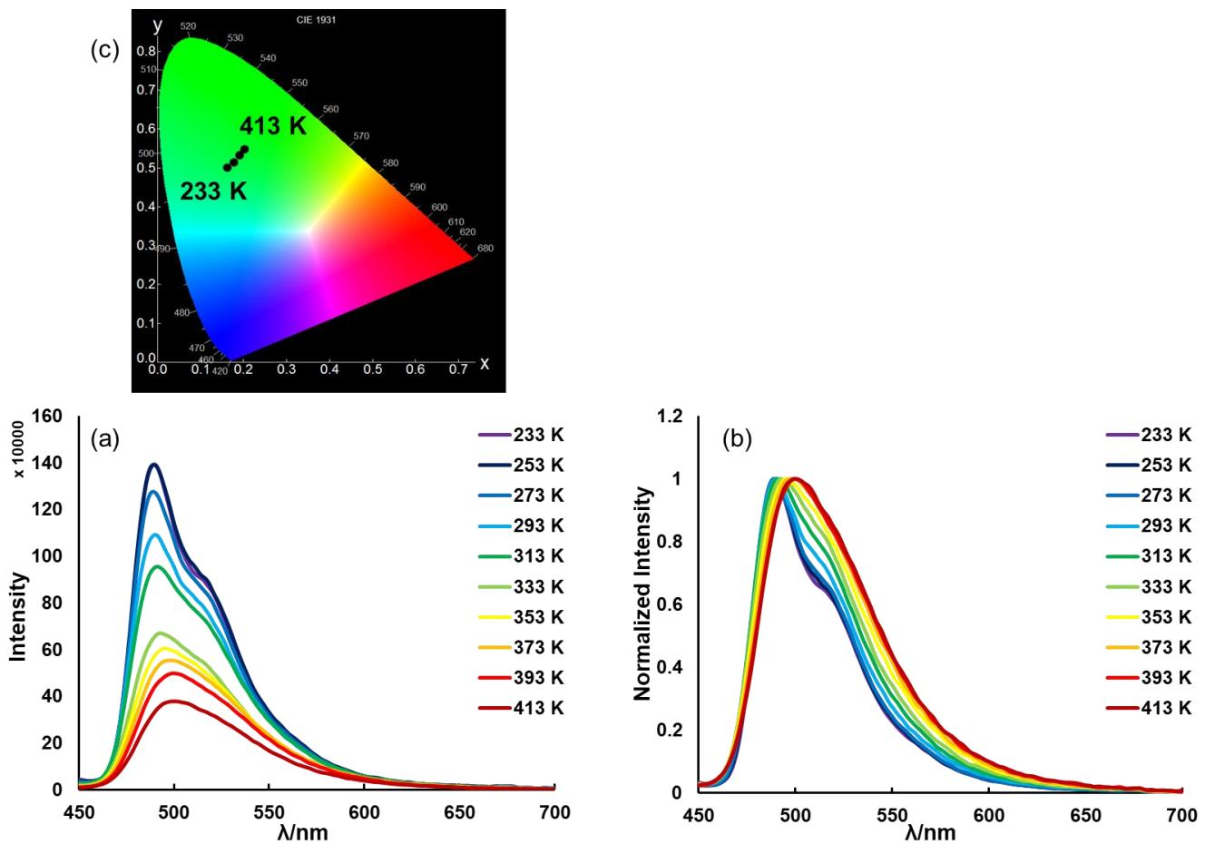
**Figure S11:** (a) CIE coordinates (CIE 1931) of **2b**. (b) Emission spectra, and (c) Normalized emission spectra of **2b** recorded between 233 K and 413 K ( $c = 1 \times 10^{-5} \text{ M}$ , in mesitylene,  $\lambda_{\text{ex}} = 320 \text{ nm}$ , under  $\text{N}_2$ )
