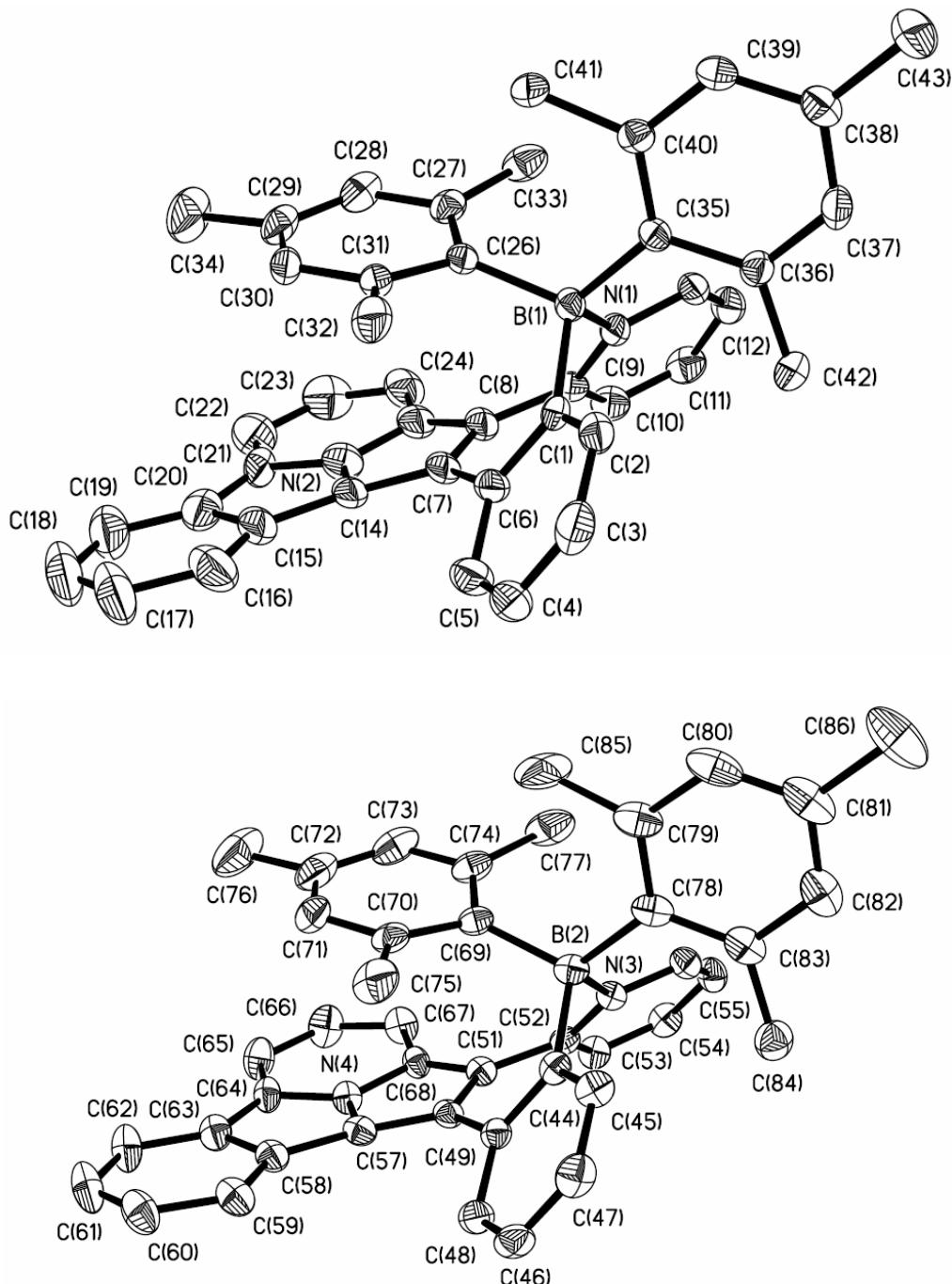
Figure S104. A diagram showing the structures of the two independent molecules in the crystal lattice of **B2b** with labeling schemes, 35% thermal ellipsoids. H atoms are omitted for clarity.
