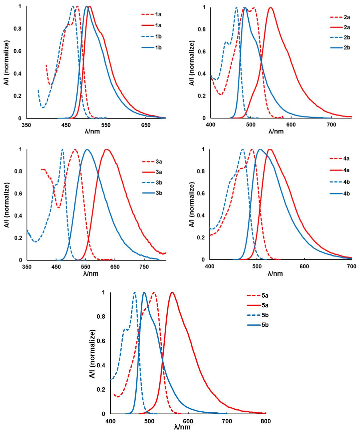
**Figure S2:** Absorption (dotted lines) and fluorescence spectra (solid line) of **1a/1b-5a/5b** in THF ( $C = 1 \times 10^{-5}$  M).
