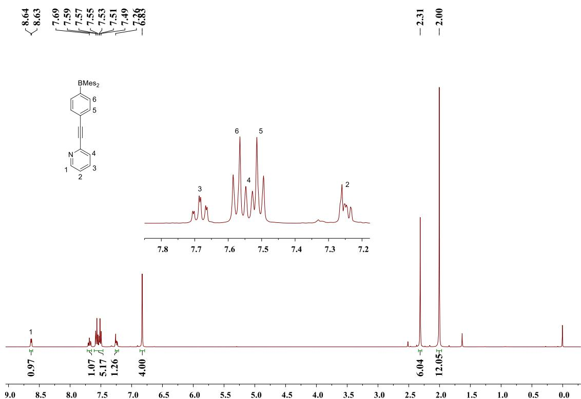
**Figure S57:**  $^1\text{H}$  NMR spectrum of compound **1** in  $\text{CDCl}_3$
