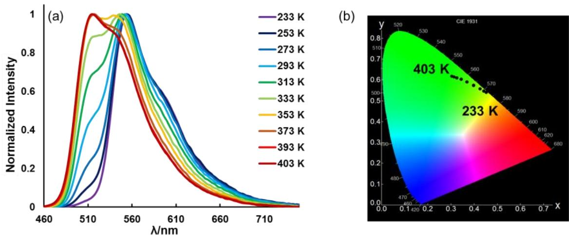
**Figure S10:** (a) Normalized emission spectra of **2a** recorded between 233 K and 403 K ( $c = 1 \times 10^{-5} \text{ M}$ , in Mesitylene,  $\lambda_{\text{ex}} = 322 \text{ nm}$ , under  $\text{N}_2$ ). (b) CIE coordinates (CIE 1931).
