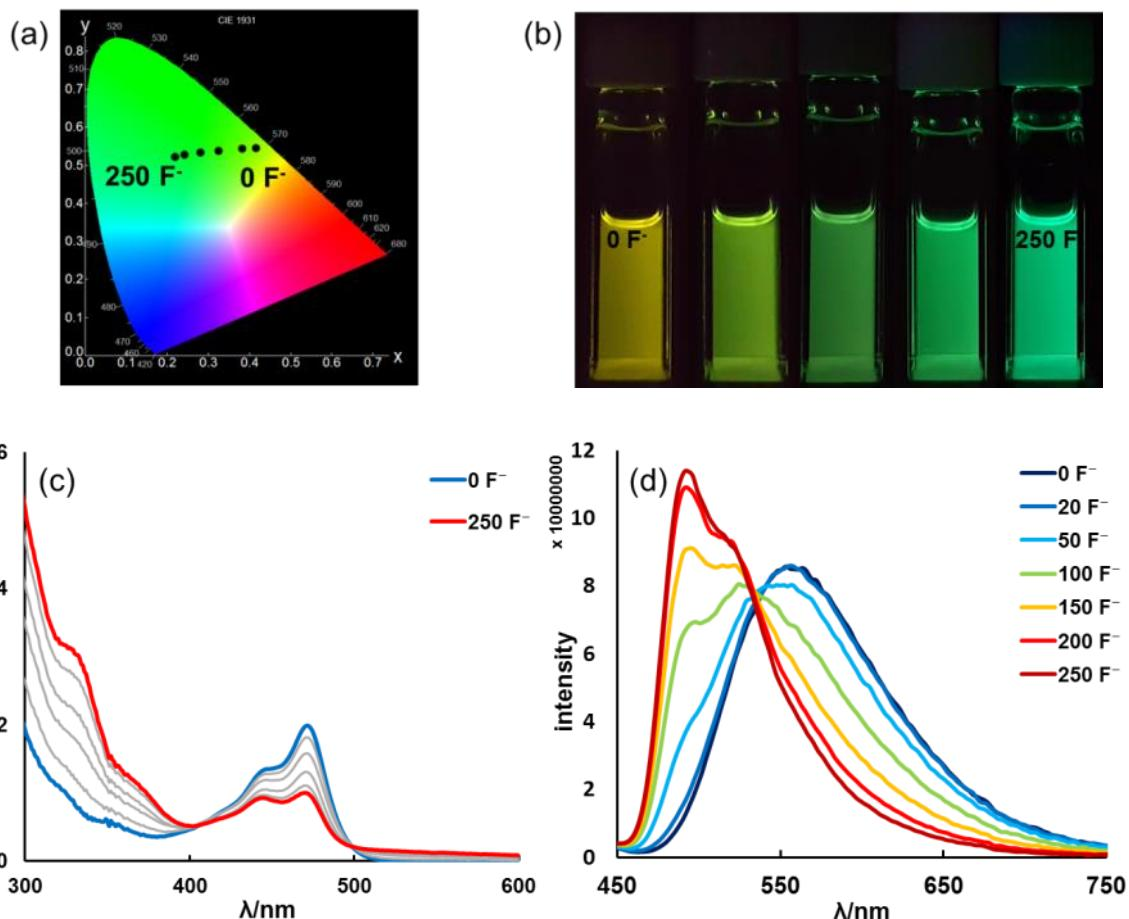
**Figure S21.** (a): CIE coordinates (CIE 1931). (b): Photographs of the solutions. (c): The UV-Vis titration spectra, and (d): Fluorescent titration spectra of **3b** ( $c = 1 \times 10^{-5}\text{ M}$ ,  $\lambda_{\text{ex}} = 313\text{ nm}$ , under air) by TBAF in THF at 298 K.
