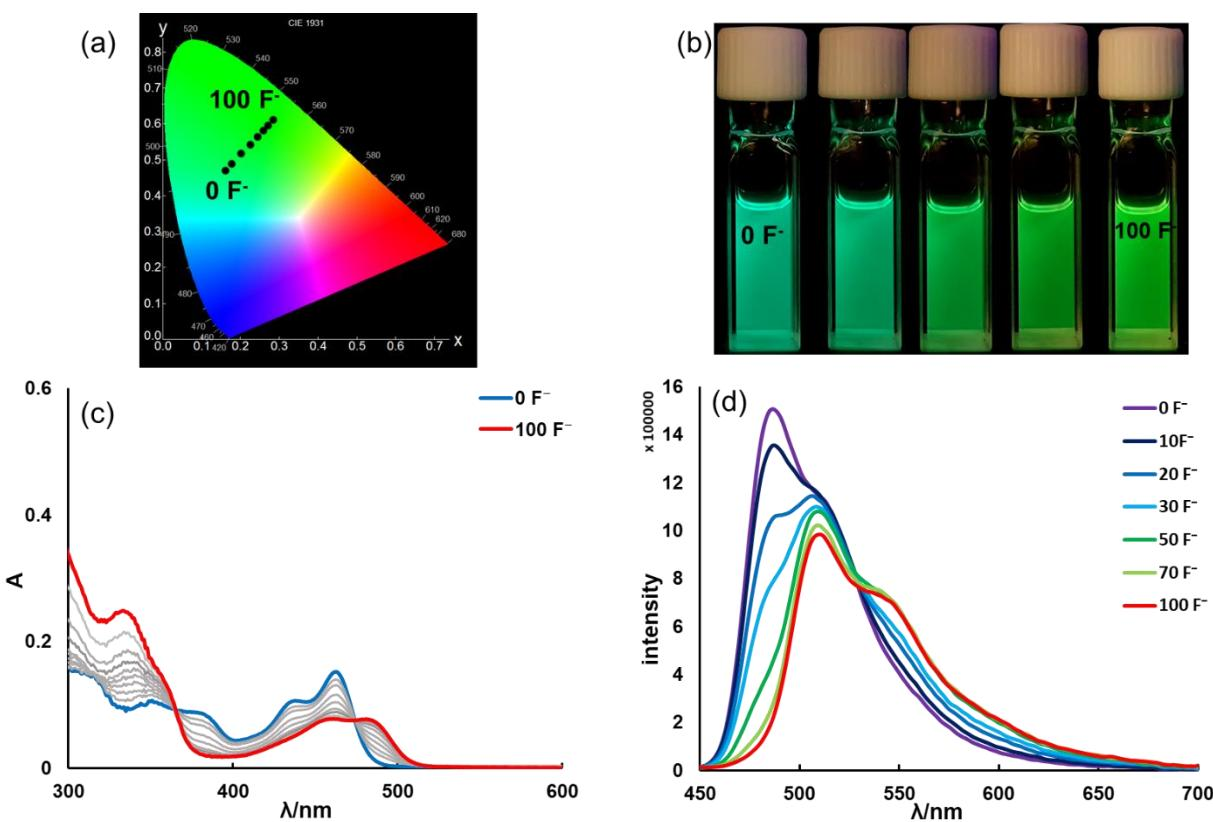
**Figure S25.** (a): CIE coordinates (CIE 1931). (b): Photographs of the solutions. (c): The UV-Vis titration spectra, and (d): Fluorescent titration spectra of **5b** ( $c = 1 \times 10^{-5}$  M,  $\lambda_{\text{ex}} = 320$  nm, under air) by TBAF in THF at 298 K.
