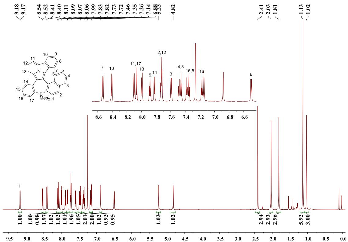
**Figure S71:**  $^1\text{H}$  NMR spectrum of compound **3a** in  $\text{CDCl}_3$
