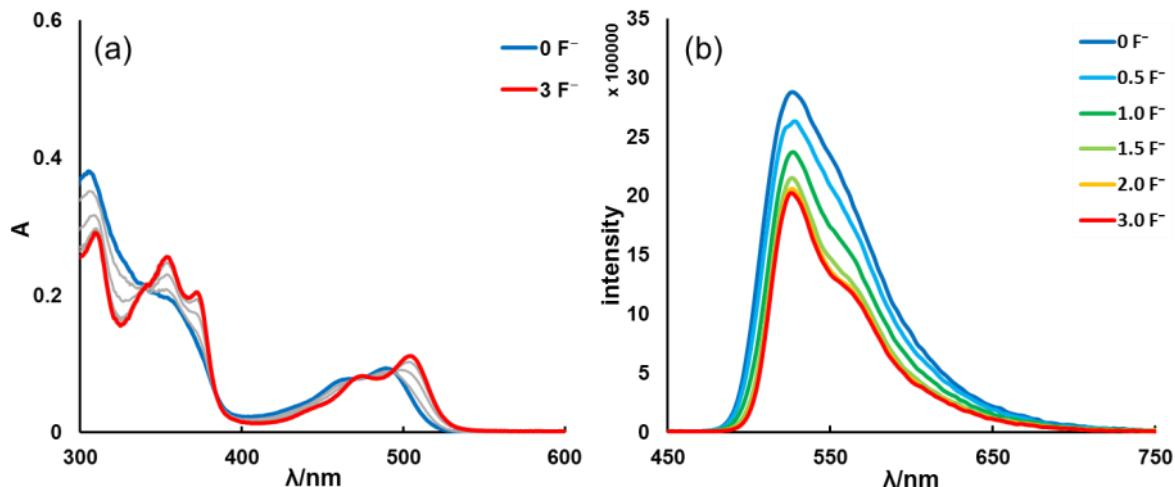
**Figure S22.** (a): The UV-Vis titration spectra, and (b): Fluorescent titration spectra of **4a** ( $c = 1 \times 10^{-5}\text{ M}$ ,  $\lambda_{\text{ex}} = 320\text{ nm}$ , under air) by TBAF in THF at 298 K.
