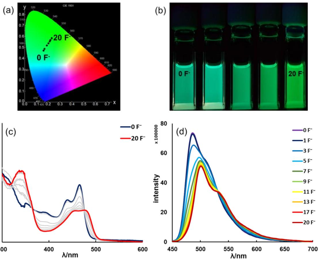
**Figure S19.** (a): CIE coordinates (CIE 1931). (b): Photographs of the solutions. (c): The UV-Vis titration spectra, and (d): Fluorescent titration spectra of **2b** ( $c = 1 \times 10^{-5}\text{ M}$ ,  $\lambda_{\text{ex}} = 320\text{ nm}$ , under air) by TBAF in THF at 298 K.
