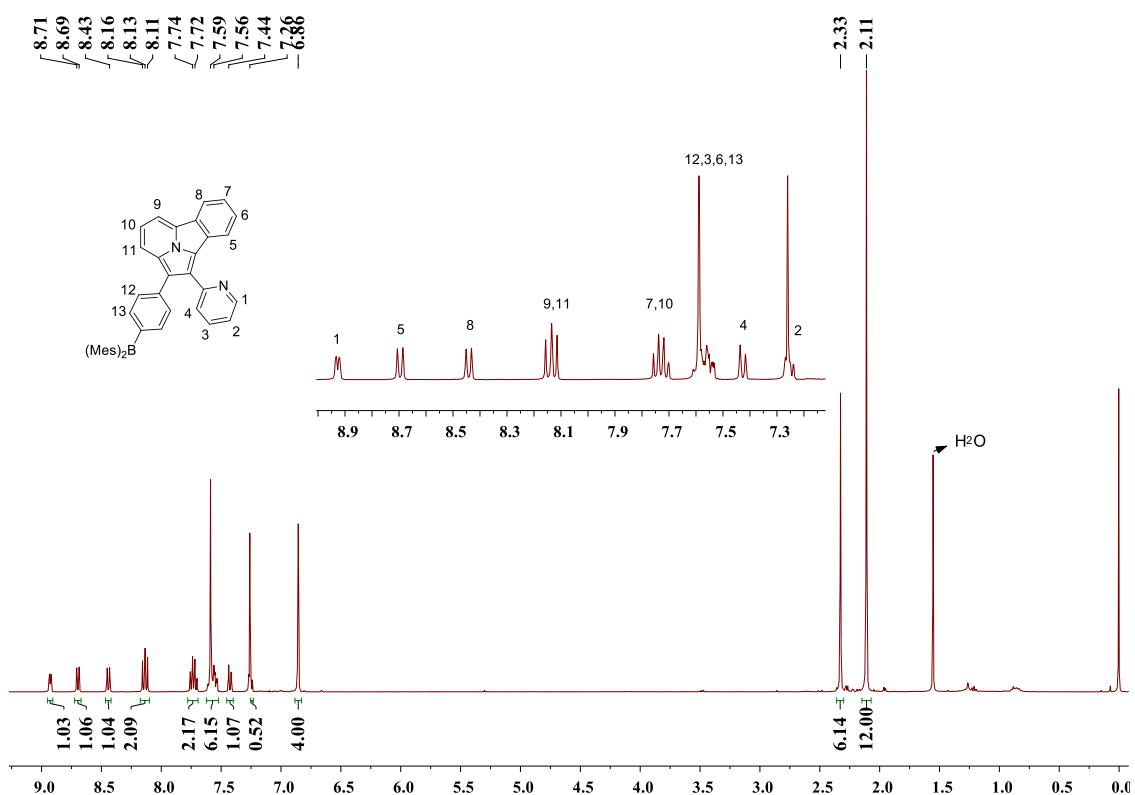
**Figure S59:**  $^1\text{H}$  NMR spectrum of compound **1a** in  $\text{CDCl}_3$
