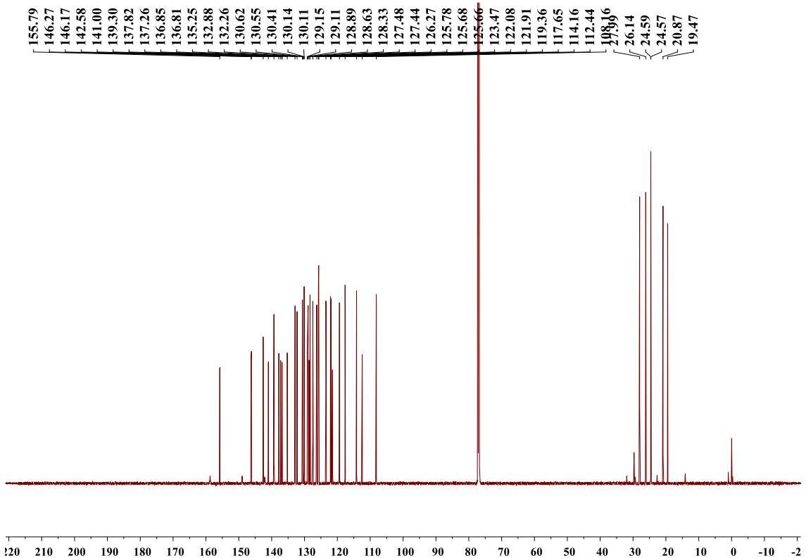
**Figure S75:**  $^{13}\text{C}$  NMR spectrum of compound **3b** in  $\text{CDCl}_3$
