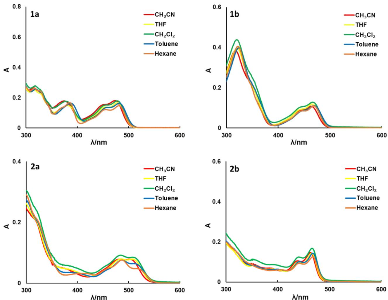
Figure S3: UV-vis Spectra of Compounds **1a/1b-2a/2b** in Different Solvents ( $c = 1 \times 10^{-5}$  mol/L).
