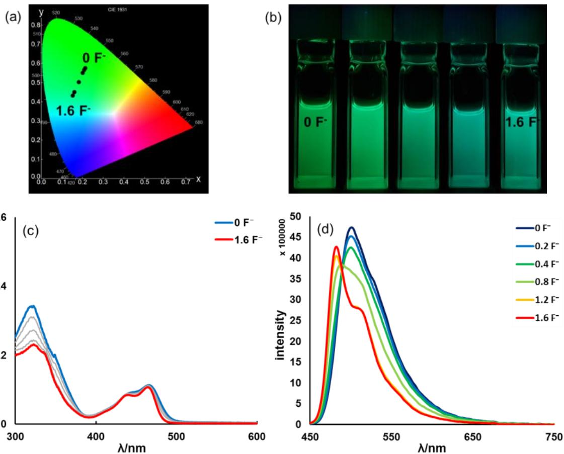
**Figure S17:** (a): CIE coordinates (CIE 1931). (b): Photographs of the solutions. (c): The UV-Vis titration spectra, and (d): Fluorescent titration of **1b** ( $c = 1 \times 10^{-5}$  M,  $\lambda_{\text{ex}} = 320$  nm, under air) by TBAF in THF at 298 K.
