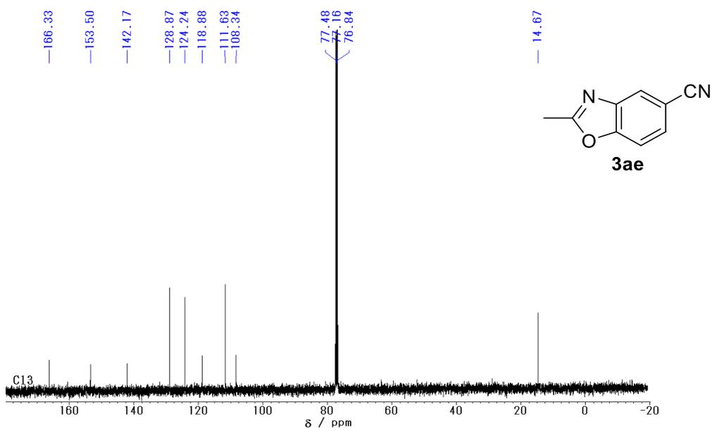
Figure S62. <sup>13</sup>C NMR spectrum of **3ae**.
