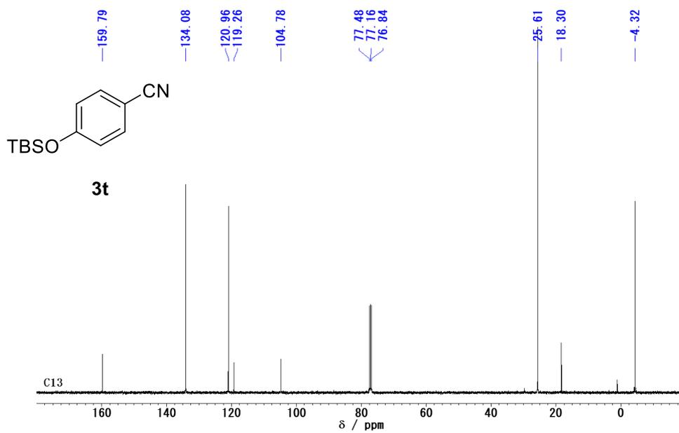
Figure S40.  $^{13}\text{C}$  NMR spectrum of **3t**.
