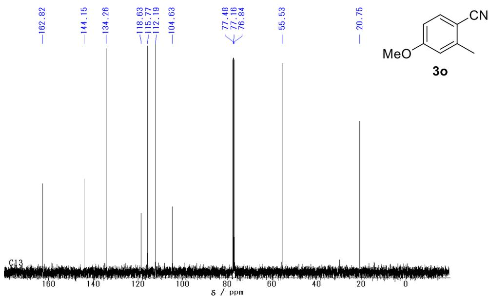
**Figure S30.**  $^{13}\text{C}$  NMR spectrum of **3o**.
