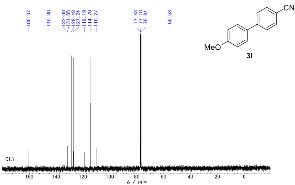
**Figure S20.**  $^{13}\text{C}$  NMR spectrum of **3i**.
