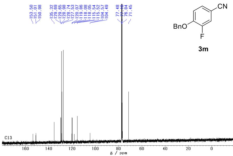
**Figure S26.**  $^{13}\text{C}$  NMR spectrum of **3m**.
