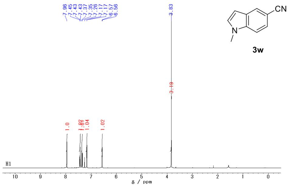
**Figure S45.**  $^1\text{H}$  NMR spectrum of **3w**.
