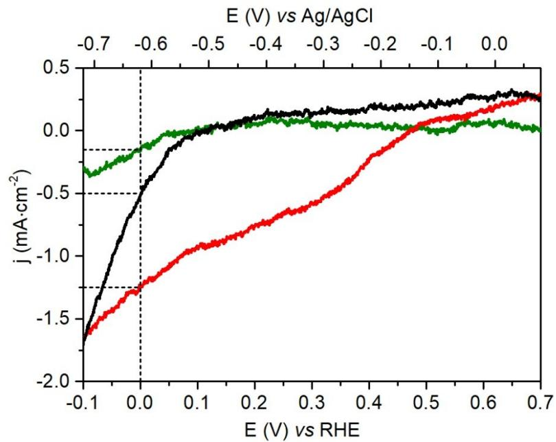
Figure S2. LSV ( $10 \text{ mV}\cdot\text{s}^{-1}$ ) of  $p\text{-Si}|ALD\text{-TiO}_2|SC\text{-TiO}_2|\text{CoC}_{11}\text{P}|ALD\text{-TiO}_2$  electrode (green trace),  $p\text{-Si}|ALD\text{-TiO}_2|SC\text{-TiO}_2$  electrode (black trace) and  $p\text{-Si}|ALD\text{-TiO}_2|SC\text{-TiO}_2|\text{CoC}_{11}\text{P}|ALD\text{-TiO}_2$  electrode (red trace) in  $1\text{M}$  phosphate buffer ( $\text{pH} 7$ ) under one Sun irradiation.
