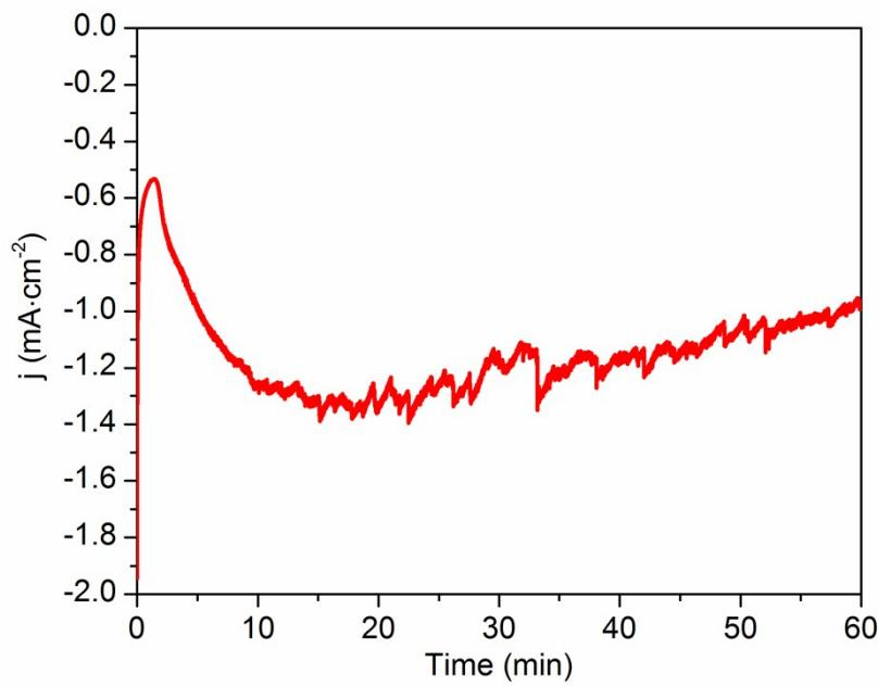
*Figure S6:* Chronoamperometric profile of  $p\text{-Si|ALD-TiO}_2|\text{SC-TiO}_2|\text{Co}_{C_{II}P}|\text{ALD-TiO}_2$  electrode recorded at 0 V vs RHE in 0.1 M NaOH (pH 13) for 60 min run under one Sun irradiation.
