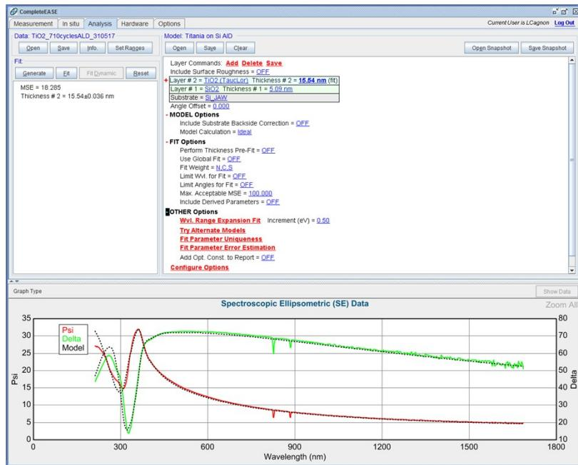
Figure S8: Ellipsometry spectra and corresponding fits for the p-Si|ALD-TiO<sub>2</sub> sample.
