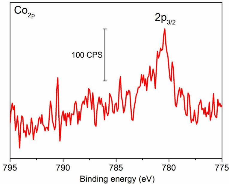
*Figure S7:* Co 2p core region XPS spectrum of  $p\text{-Si|ALD-TiO}_2|\text{SC-TiO}_2|\text{Co}_{C_{II}P}|\text{ALD-TiO}_2$  electrode analyzed after one hour of photoelectrolysis (0 V vs RHE) in 0.1 M NaOH.
