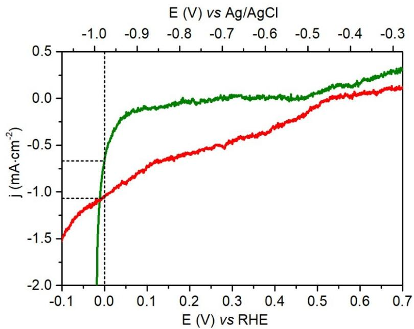
Figure S5: LSV ( $10 \text{ mV.s}^{-1}$ ) of  $p\text{-Si|ALD-TiO}_2|\text{SC-TiO}_2|\text{CoC}_{10}\text{P|ALD-TiO}_2$  electrode (green trace) and  $p\text{-Si|ALD-TiO}_2|\text{SC-TiO}_2|\text{CoC}_{11}\text{P|ALD-TiO}_2$  electrode (red trace) in 0.1 M NaOH (pH 13) under one Sun irradiation.
