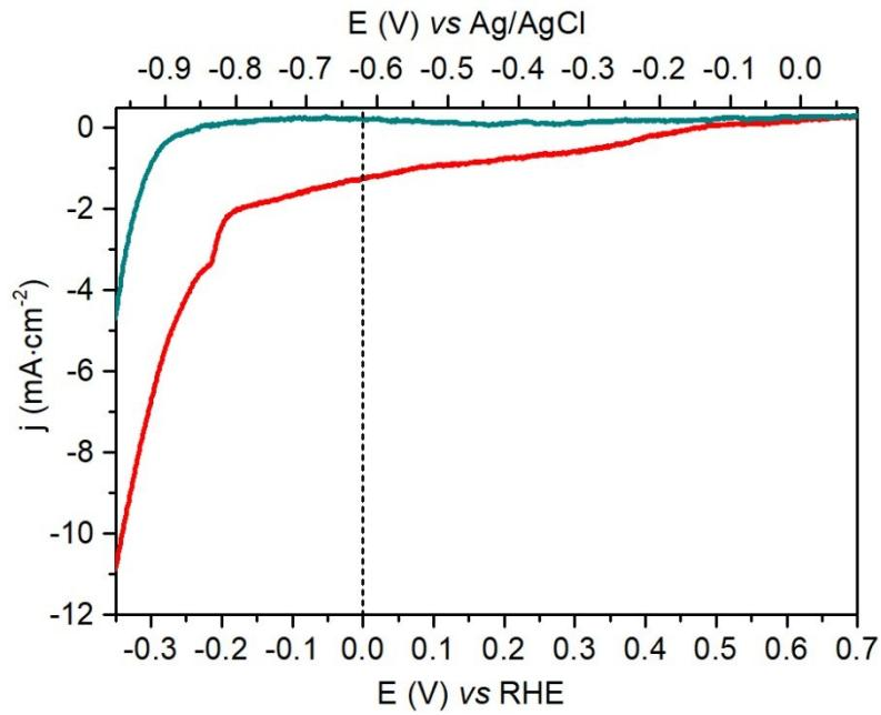
Figure S4: LSV ( $10 \text{ mV.s}^{-1}$ ) of  $p\text{-Si|ALD-TiO}_2|\text{SC-TiO}_2$  (cyan trace) and  $p\text{-Si|ALD-TiO}_2|\text{SC-TiO}_2|\text{CoC}_{11}\text{P|ALD-TiO}_2$  electrode (red trace) in 1M phosphate buffer (pH 7) under one Sun irradiation.
