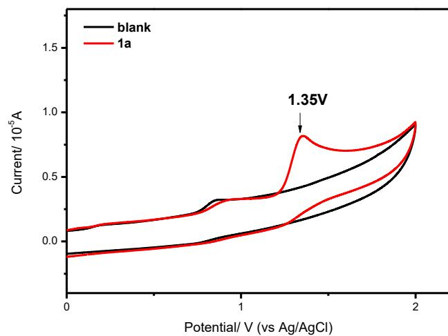
**Figure S1.** Cyclic voltammetry of **1a** ( $5 \times 10^{-4}$  M) in CH<sub>3</sub>CN with  ${}^n\text{Bu}_4\text{NBF}_4$  (0.01 M) under nitrogen at a scan rate of v=50 mV/s.
