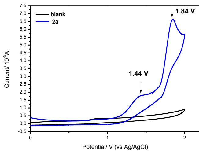
**Figure S2.** Cyclic voltammetry of **2a** (10<sup>-3</sup> M) in CH<sub>3</sub>CN with  ${}^n\text{Bu}_4\text{NBF}_4$  (0.01 M) under nitrogen at a scan rate of v=50 mV/s.
