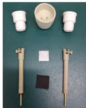
a. a carbon cloth, a Fe plate, two electrode
