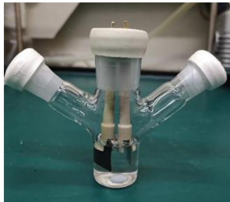
c. Assembly of electrochemical cell
