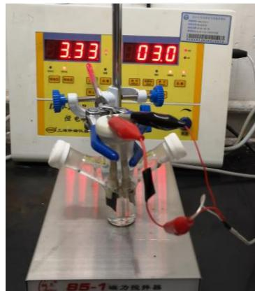
d. Current controlled electrolysis
