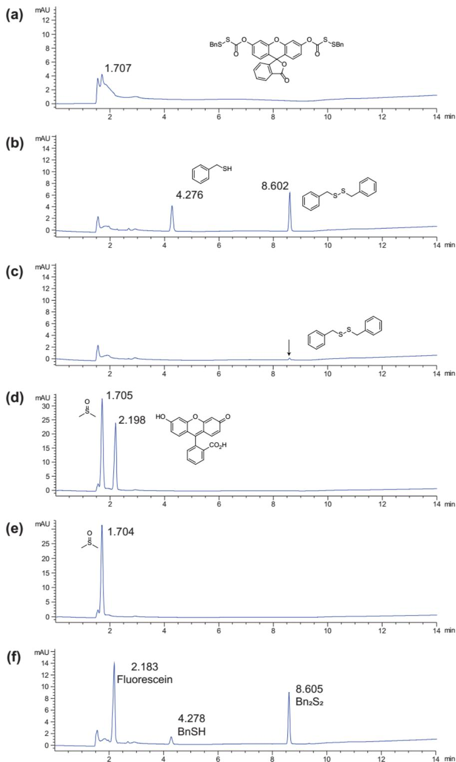
**Figure S3.** Reaction analysis by HPLC. (a) 10  $\mu\text{M}$  FLD-1 (b) 100  $\mu\text{M}$  BnSH containing  $\text{Bn}_2\text{S}_2$  due to aerobic oxidation (c) 20  $\mu\text{M}$   $\text{Bn}_2\text{S}_2$  (d) 10  $\mu\text{M}$  fluorescein (e) 0.1% (v/v) DMSO in 10 mM PBS (pH 7.4) (f) Reaction aliquot after 1 h.
