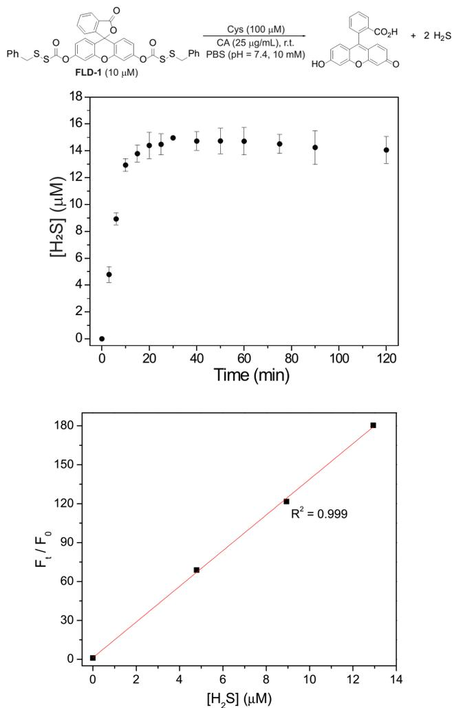
**Figure S2.** (Top) MB Measurement of H<sub>2</sub>S release from **FLD-1** (10 μM) upon Cys (100 μM) activation. (Bottom) Correlation between fluorescence measurement of **FLD-1** in Figure 1B and MB detection in the first 10-min reaction period. The experiments were performed in triplicate. The results are expressed as mean ± SD (n = 3)
