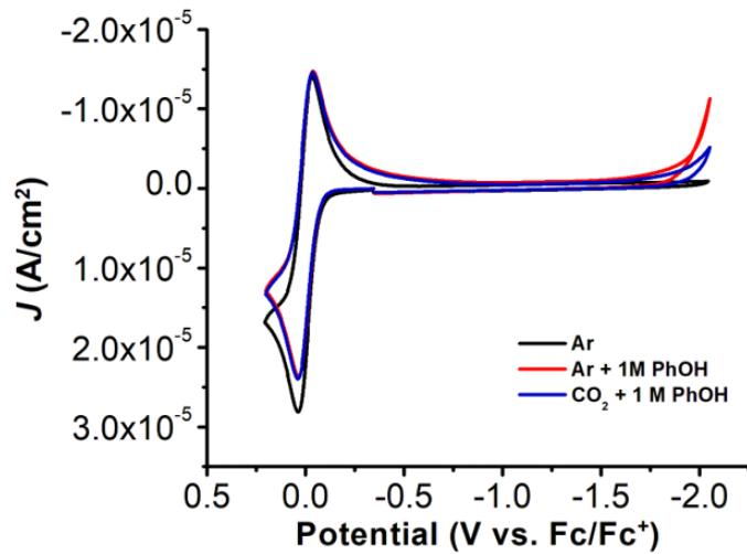
**Figure S17.** CVs showing CO<sub>2</sub> and PhOH control responses. Conditions: 0.1 M TBAPF<sub>6</sub>/MeCN, glassy carbon working electrode, glassy carbon counter electrode, Ag/AgCl pseudoreference electrode; scan rate 100 mV/s; referenced to internal ferrocene standard.
