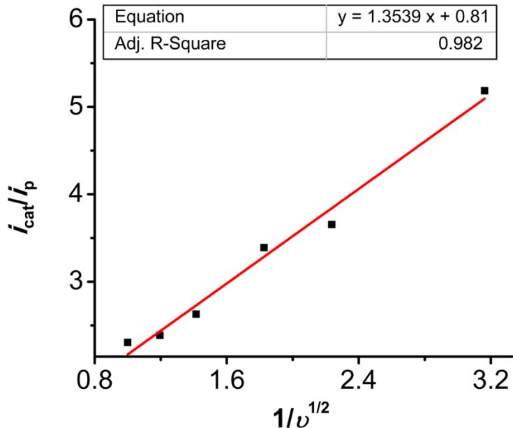
**Figure S19.** Linear fit between peak catalytic current over non-catalytic vs the inverse square root of the scan rate from the variable scan rate data in **Figure S18**.<sup>3</sup> This establishes the validity of using the equations for the FOWA.<sup>3</sup>
