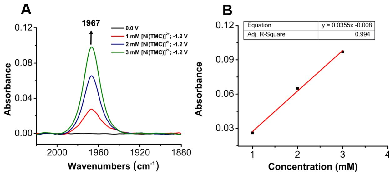
**Figure S33.** **A)** IR-SEC analysis of  $[\text{Ni}(\text{TMC})]^{2+}$  **1** with CO sparged into solution for  $\sim 30$  s to show the  $[\text{Ni}(\text{TMC})(\text{CO})]^+$  stretch at  $1967 \text{ cm}^{-1}$ . Conditions: 0.1 M TBAPF<sub>6</sub>/MeCN; referenced to internal ferrocene standard. **B)** Linear fit of  $[\text{Ni}(\text{TMC})(\text{CO})]^+$  absorbance.
