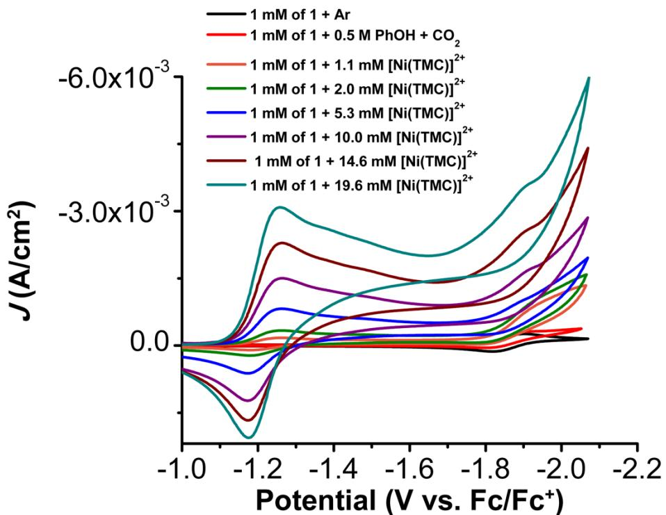
**Figure S27.** CVs of  $[\text{Ni}(\text{TPEN})](\text{PF}_6)_2$  **1** at 1 mM, obtained under  $\text{CO}_2$  saturation with 0.5 M PhOH and with  $[\text{Ni}(\text{TMC})]^{2+}$  titrations. Conditions: 1 mM analyte; 0.1 M TBAPF<sub>6</sub>/MeCN glassy carbon working electrode, glassy carbon counter electrode, Ag/AgCl pseudoreference electrode; scan rate 100 mV/s; referenced to internal ferrocene standard.
