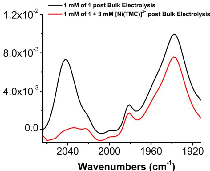
**Figure S26.** IR comparison between the post bulk electrolysis experiments of  $[\text{Ni}(\text{TPEN})](\text{PF}_6)_2$  **1** with and without  $[\text{Ni}(\text{TMC})]^{2+}$ .  $\text{Ni}(\text{CO})_4$  appears at  $2042 \text{ cm}^{-1}$  while the Ni-CO stretch is observed at  $1981 \text{ cm}^{-1}$  in both solutions.
