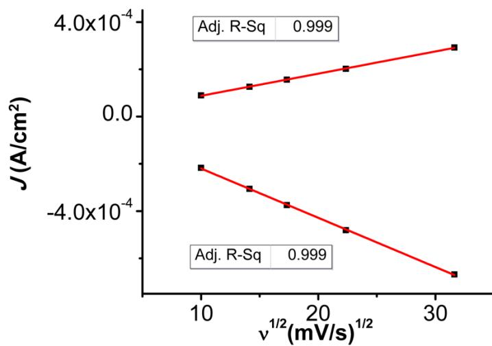
**Figure S10.** Linear Fit of variable scan rate data from **Figure 3** demonstrating that  $[\text{Ni}(\text{TPEN})](\text{PF}_6)_2 \mathbf{1}$  shows a diffusion-limited current response. Conditions: 1 mM analyte; 0.1 M TBAPF<sub>6</sub>/MeCN, glassy carbon working electrode, Pt wire counter electrode, Ag/AgCl pseudoreference electrode; varied scan rate; referenced to internal ferrocene standard.
