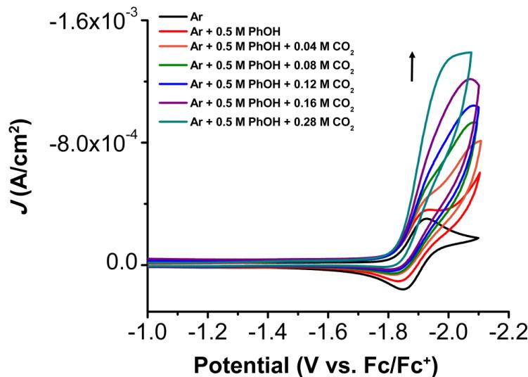
**Figure S13.** CVs of  $[\text{Ni}(\text{TPEN})](\text{PF}_6)_2$  **1**, obtained under variable  $\text{CO}_2$  concentrations with 0.5 M PhOH. Conditions: 1 mM analyte; 0.1 M TBAPF<sub>6</sub>/MeCN, glassy carbon working electrode, glassy carbon counter electrode, Ag/AgCl pseudoreference electrode; scan rate 100 mV/s; referenced to internal ferrocene standard.
