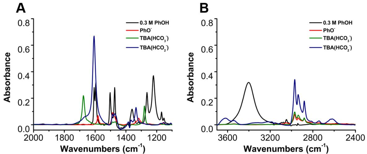
**Figure S22.** IR controls for the following with their corresponding  $v_{\text{max}}/\text{cm}^{-1}$  taken in MeCN: TBA( $\text{HCO}_2^-$ ) 1333  $\text{cm}^{-1}$  and 1608  $\text{cm}^{-1}$ ,<sup>6</sup> TBA( $\text{HCO}_3^-$ ) (1676  $\text{cm}^{-1}$ ),  $\text{PhO}^-$  (1589  $\text{cm}^{-1}$ ) and PhOH (3408  $\text{cm}^{-1}$ ) in MeCN.
