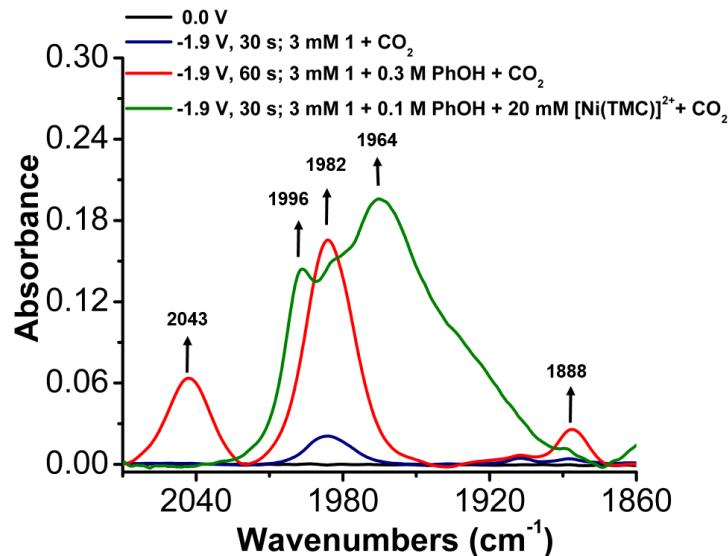
**Figure S35.** IR-SEC spectra overlaying of 3 mM Ni(TPEN)[PF<sub>6</sub>]<sub>2</sub> **1** with the addition of 20 mM [Ni(TMC)]<sup>2+</sup> to show the loss of Ni(CO)<sub>4</sub> formation upon the addition of the CO scavenger. Timepoints: blue 60 s; red 30 s; green 60 s.
