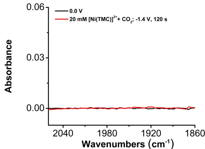
**Figure S32.** IR-SEC analysis of a 20 mM solution of  $[\text{Ni}(\text{TMC})]^{2+}$  with  $\text{CO}_2$ , without the addition of  $[\text{Ni}(\text{TPEN})](\text{PF}_6)_2$  **1**. No carbonyl-containing species are observed. Conditions: 0.1 M TBAPF<sub>6</sub>/MeCN; referenced to internal ferrocene standard.
