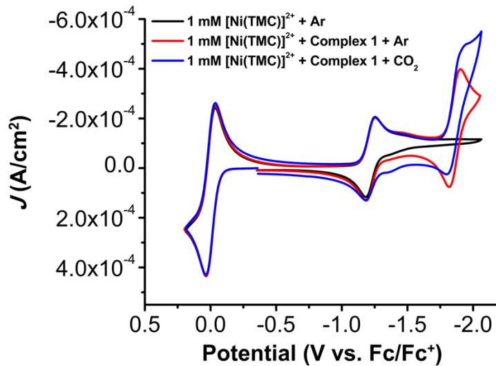
**Figure S31.** CVs of  $[\text{Ni}(\text{TPEN})](\text{PF}_6)_2\mathbf{1}$  (1 mM) obtained under Ar and then Ar and  $\text{CO}_2$  upon the addition of 1 mM of  $[\text{Ni}(\text{TMC})]^{2+}$ . Conditions: 0.1 M TBAPF<sub>6</sub>/MeCN, glassy carbon working electrode, glassy carbon counter electrode, Ag/AgCl pseudoreference electrode; scan rate 100 mV/s; referenced to internal ferrocene standard.
