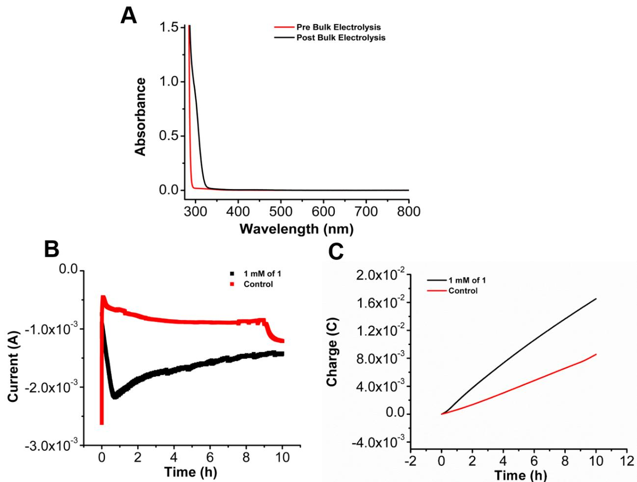
**Figure S25.** **A)** UV-Vis of the bulk solution before and after electrolysis. **B)** Current vs time plot of electrolysis experiment held at -2.05 V vs Fc/Fc<sup>+</sup>. **C)** Charge passed during electrolysis experiment. Conditions: 1 mM of [Ni(TPEN)](PF<sub>6</sub>)<sub>2</sub> **1**; 0.5 M PhOH; 0.1 M TBAPF<sub>6</sub>/MeCN, graphite working electrode, graphite carbon counter electrode, Ag/AgCl pseudoreference electrode, and 0.5 M Fc was used as a sacrificial oxidant.
