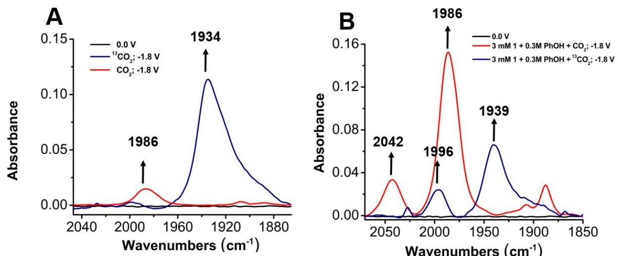
**Figure S23.** A comparison of the  $[\text{Ni}(\text{TPEN})(\text{CO})]^+$  stretch with labeled  $\text{CO}_2$  without (**A**) and with 0.3 M solution of PhOH (**B**). Conditions: 3 mM solution of (**1**),  $^{13}\text{CO}_2$  and  $\text{CO}_2$  sparged for ~30s; 0.1 M TBAPF<sub>6</sub>/MeCN; referenced to internal ferrocene standard.
