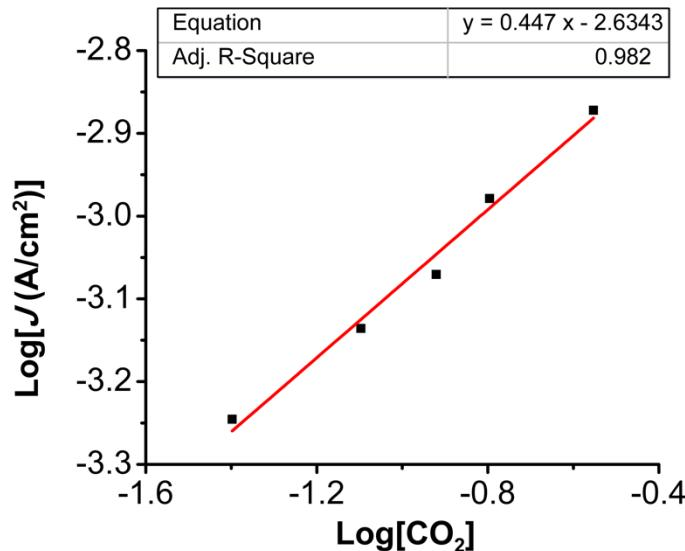
**Figure S14.** Log-log plot from data obtained from CVs of complex  $[\text{Ni}(\text{TPEN})](\text{PF}_6)_2$  **1** (1 mM) under variable  $\text{CO}_2$  concentration conditions with 0.5 M PhOH at -2.0 V vs  $\text{Fc}/\text{Fc}^+$ .
