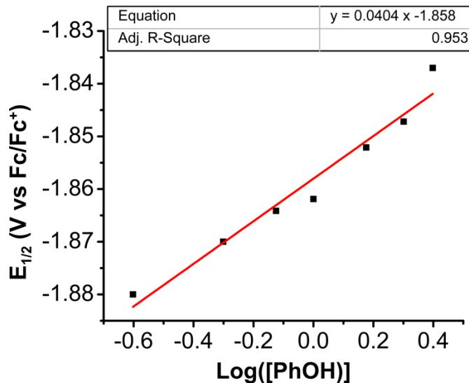
**Figure S12.** Plot displaying the Nernstian voltage dependence of  $[\text{Ni(TPEN)}](\text{PF}_6)_2 \mathbf{1}$  on the concentration of PhOH in MeCN under  $\text{CO}_2$  saturation. Conditions: 0.1 M TBAPF<sub>6</sub>/MeCN, glassy carbon working electrode, glassy carbon counter electrode, Ag/AgCl pseudoreference electrode; scan rate 100 mV/s; referenced to internal ferrocene standard. Uses data from **Figure 5** in main text.
