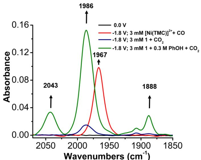
**Figure S34.** A comparison of the 3 mM solution of **(1)** with a 3 mM solution of  $[\text{Ni}(\text{TMC})]^{2+}$  to show the catalytic activity of  $[\text{Ni}(\text{TPEN})]^{2+}$ .
