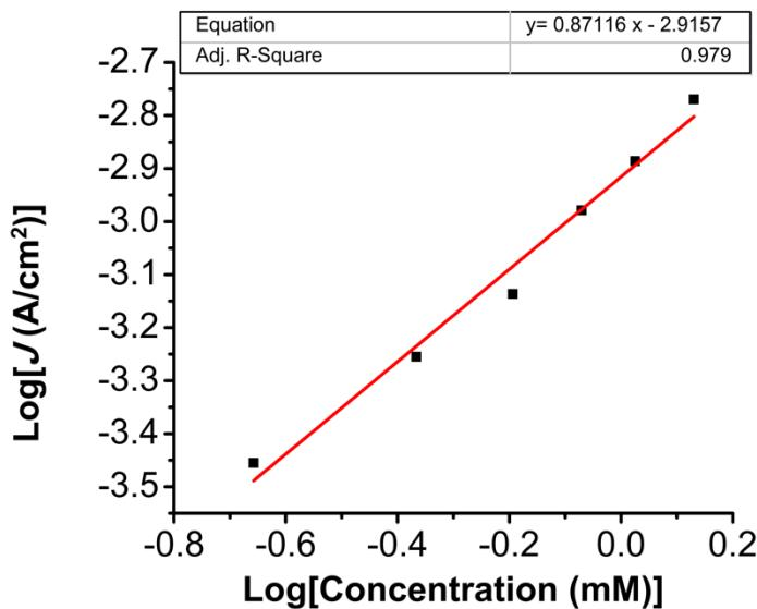
**Figure S16.** Log-log plot from data obtained from CVs of complex  $[\text{Ni}(\text{TPEN})](\text{PF}_6)_2 \mathbf{1}$  under variable concentration conditions with 0.5 M PhOH and  $\text{CO}_2$  saturation at -1.93 V vs  $\text{Fc}/\text{Fc}^+$ .
