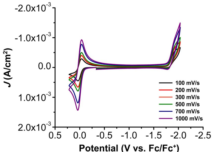
**Figure S18.** Cyclic voltammogram of [Ni(TPEN)](PF<sub>6</sub>)<sub>2</sub> (**1**) (1 mM) under CO<sub>2</sub> saturation and 0.5 M PhOH. Conditions: 0.1 M TBAPF<sub>6</sub>/MeCN; glassy carbon working electrode, glassy carbon counter electrode; Ag/AgCl pseudoreference electrode; varied scan rate; referenced to internal ferrocene standard.
