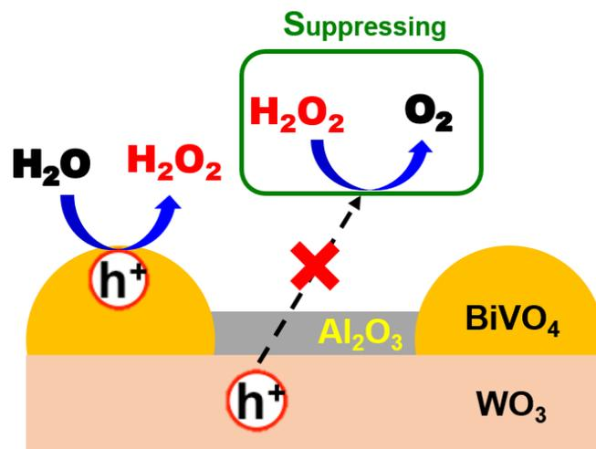
Figure S10 Speculated scheme for the suppression of  $\text{H}_2\text{O}_2$  decomposition on  $\text{Al}_2\text{O}_3(\text{CVD})/\text{BiVO}_4/\text{WO}_3$  photoelectrode.
