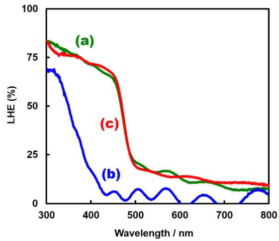
Figure S9. Light harvesting efficiency (LHE) of (a) BiVO<sub>4</sub>/WO<sub>3</sub>, (b) BiVO<sub>4</sub>, and (c) WO<sub>3</sub> photoelectrode by irradiation from the front side.
