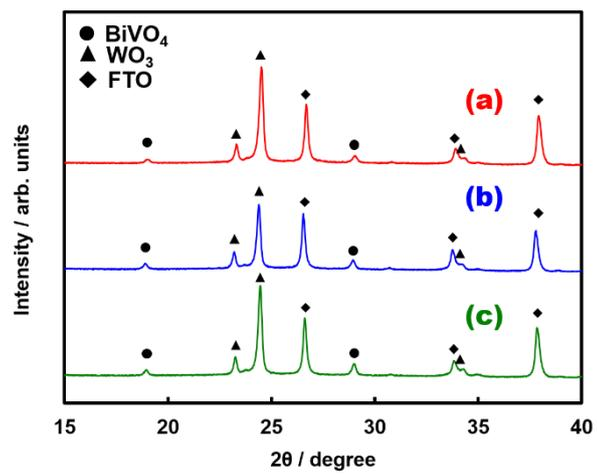
Figure S5. XRD patterns of (a)  $\text{Al}_2\text{O}_3(\text{CVD5})/\text{BiVO}_4/\text{WO}_3$ , (b)  $\text{Al}_2\text{O}_3(\text{MOD})/\text{BiVO}_4/\text{WO}_3$ , and (c)  $\text{BiVO}_4/\text{WO}_3$ .
