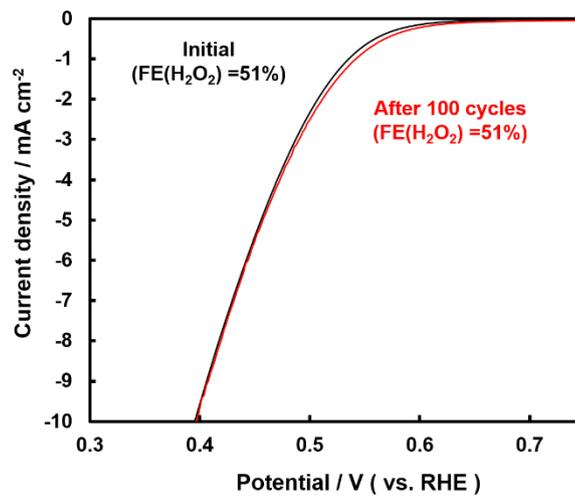
Figure S11 The comparison of I-V curve and faradaic efficiency (FE) for H<sub>2</sub>O<sub>2</sub> production on WSox/GnP-CP cathode. The cathode was utilized before / after 100 cycles of CV measurement operated under the same condition of Figure 7.
