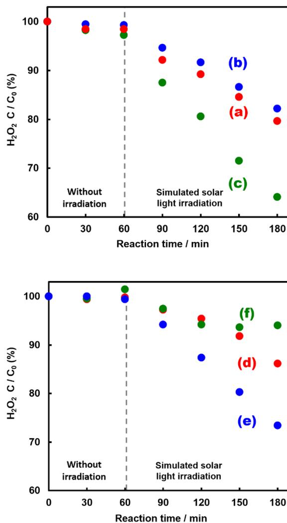
Figure S8. Photodecomposition rate ( $C/C_0$ ) of  $H_2O_2$  on each electrode ( $6\text{ cm}^2$ ): (a)  $Al_2O_3(\text{CVD5})/BiVO_4/WO_3$ , (b)  $Al_2O_3(\text{MOD})/BiVO_4/WO_3$ , (c)  $BiVO_4/WO_3$ , (d)  $BiVO_4$ , (e)  $WO_3$  and (f) FTO without external bias. Electrolyte solution:  $0.5\text{ M KHCO}_3$  aqueous solution with  $550\text{ }\mu\text{M H}_2\text{O}_2$  under  $CO_2$  bubbling and simulated solar irradiation.
