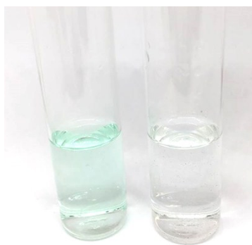
Fig. S5. Digital photograph of electrolyte after stability test of Ni foam (left) and G-4@Ni foam (Right).
