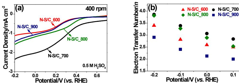
**Fig. S8.** (a) LSVs of N-S/C\_600, N-S/C\_700, N-S/C\_800, and N-S/C\_900 recorded at 400 rpm and 5 mV s<sup>-1</sup> in oxygen-saturated H<sub>2</sub>SO<sub>4</sub> (0.5 M). (b) Number of electrons transferred for N-S/C\_600, N-S/C\_700, N-S/C\_800, and N-S/C\_900 derived from the LSV results.
