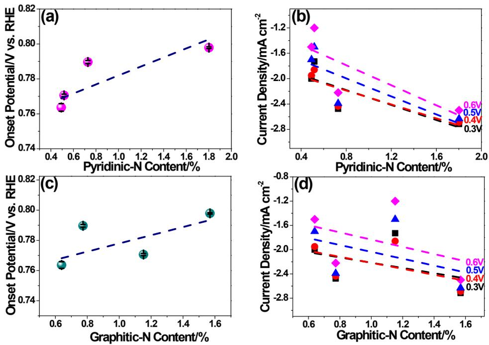
**Fig. S5.** Correlation of onset potential with content of (a) pyridinic nitrogen and (c) graphitic nitrogen. Correlation of current density (0.3 V, 0.4 V, 0.5 V and 0.6 V vs. RHE) with content of (b) pyridinic nitrogen and (d) graphitic nitrogen.
