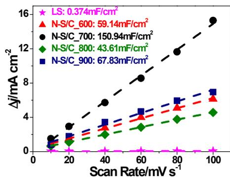
**Fig. S7.** Current density of CV experiments of LS, N-S/C\_600, N-S/C\_700, N-S/C\_800, and N-S/C\_900 at 0.65 V (vs. RHE) as a function of scan rate. The slope of each line shows the double layer capacitor of corresponding catalyst.
