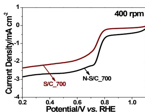
**Fig. S4.** LSVs of LS annealed at 700 °C (S/C\_700) and N-S/C\_700 recorded at 400 rpm in O<sub>2</sub>-saturated aqueous KOH (0.1 M).
