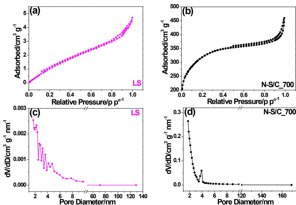
**Fig. S3.** Nitrogen sorption isotherms of (a) LS and (b) N-S/C\_700 at 77 K. Pore size distribution profiles of (c) LS and (d) N-S/C\_700.
