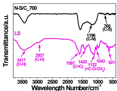
**Fig. S1.** FTIR spectra of original lignosulfonate (LS) and N-S/C<sub>700</sub>. Characteristic anti-symmetry and symmetry stretching vibrations of sulfonic group (1043 cm<sup>-1</sup> and 621 cm<sup>-1</sup>), O-H (3417 cm<sup>-1</sup>), C-H (2927 cm<sup>-1</sup>), C=C (1597 cm<sup>-1</sup> and 1420 cm<sup>-1</sup>), and =C-O-CH<sub>3</sub> (1122 cm<sup>-1</sup>) were observed in the LS [1].
