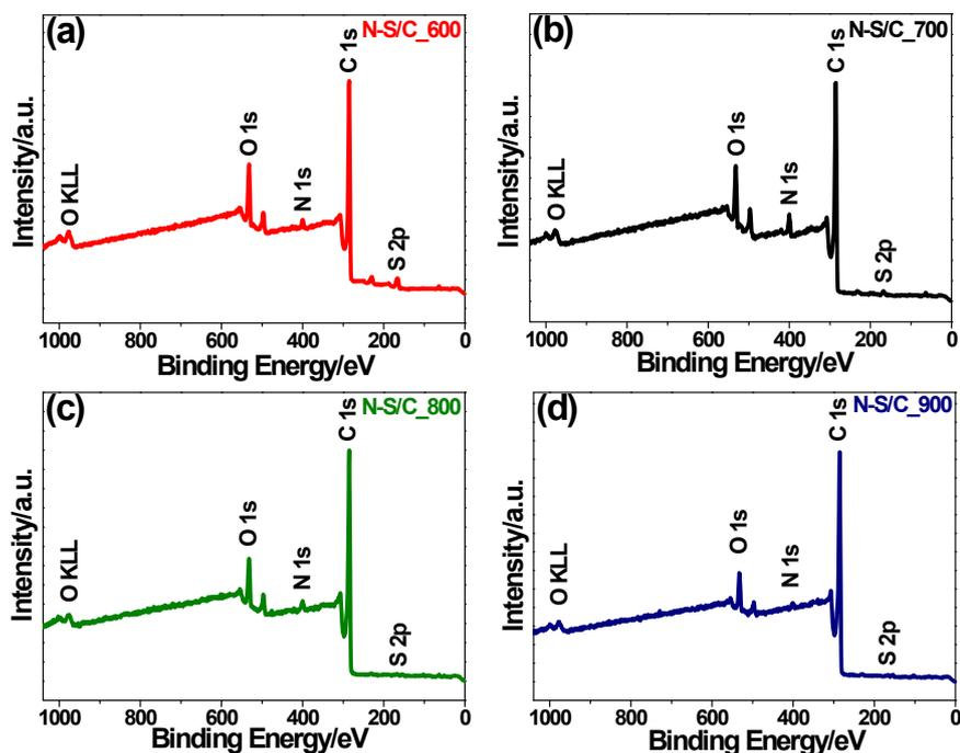
**Fig. S2.** Wide-survey XPS spectra of (a) N-S/C\_600, (b) N-S/C\_700, (c) N-S/C\_800, and (d) N-S/C\_900.
