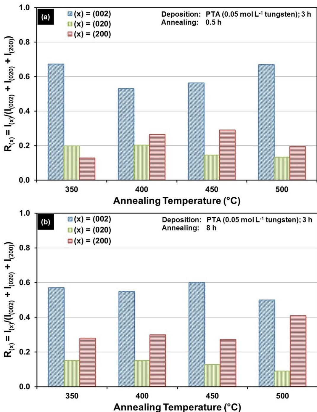
**Figure S2.** Relative XRD intensities  $R_{(x)} = (I_{(x)}) / (I_{(002)} + I_{(020)} + I_{(200)})$  (where  $(x) = (002)$ ,  $(020)$ , or  $(200)$ ) as a function of annealing temperature for the films deposited from PTA consisting of 0.05 mol L<sup>-1</sup> tungsten and annealed for (a) 0.5 h or (b) 8 h.
