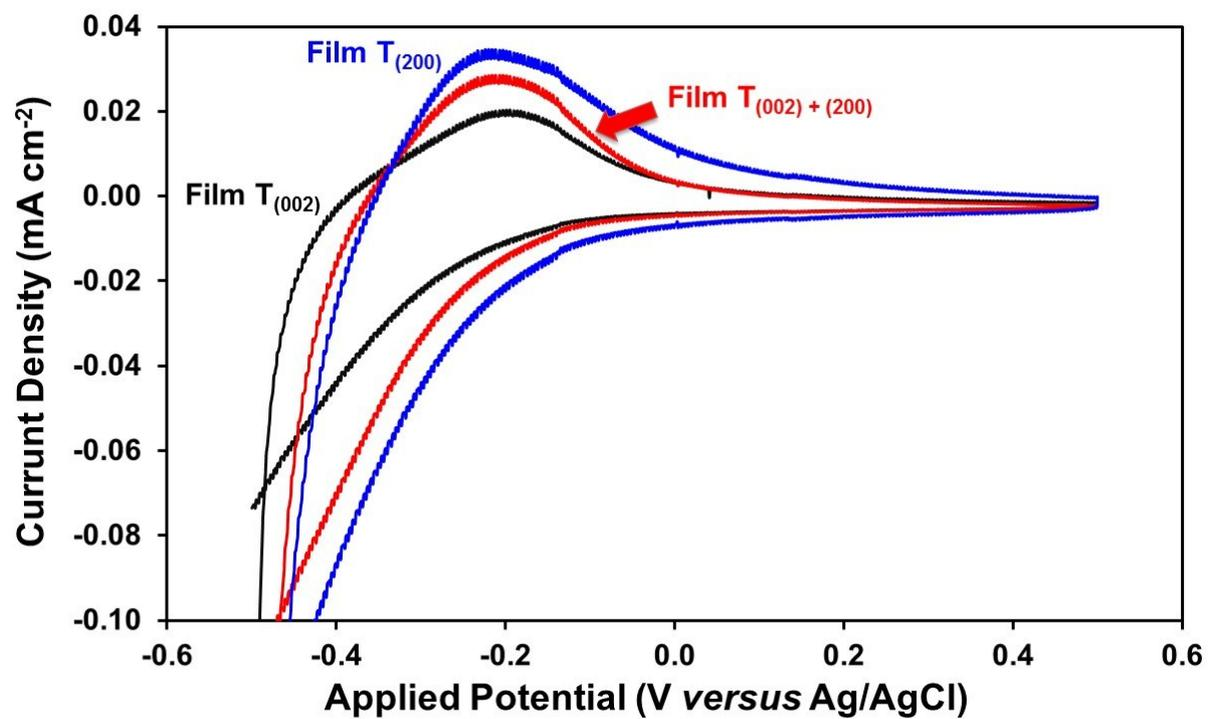
**Figure S4.** Cyclic voltammograms of films  $T_{(002)}$ ,  $T_{(002) + (200)}$ , and  $T_{(200)}$  measured in 0.5 mol L<sup>-1</sup> NaCl aqueous solution in dark environment.
