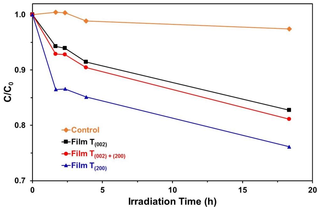
**Figure S8.** Photocatalytic degradation of methylene blue as a function of irradiation time  $t$ ;  $C$  and  $C_0$  are the concentrations of methylene blue at irradiation time  $t$  and  $t = 0$ , respectively; major spectral output: 365 nm;  $C_0 = 4.5$  ppm.
