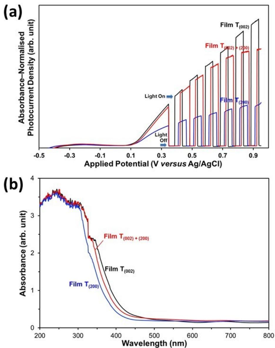
**Figure S7.** (a) Photocurrent densities normalised to the total optical absorbances of films  $T_{(002)}$ ,  $T_{(002) + (200)}$ , and  $T_{(200)}$ ; the total optical absorbances were obtained by calculating the area under the optical absorbance-wavelength curves shown in **Figure S7 (b)**.
