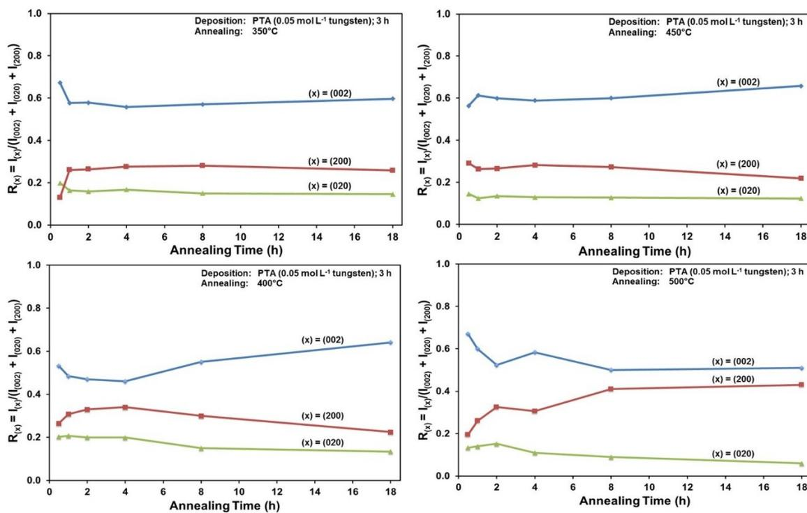
**Figure S1.** Relative XRD intensities  $R_{(x)} = I_{(x)} / (I_{(002)} + I_{(020)} + I_{(200)})$  (where (x) = (002), (020), or (200)) as a function of annealing time for the films deposited from PTA consisting of 0.05 mol L<sup>-1</sup> tungsten and annealed at fixed temperatures in the range 350°-500°C.
