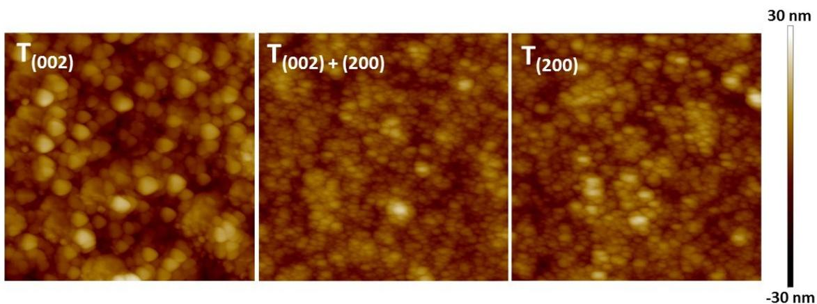
**Figure S5.** AFM images (scanned area:  $3 \mu\text{m} \times 3 \mu\text{m}$ ) of films  $T_{(002)}$ ,  $T_{(002) + (200)}$ , and  $T_{(200)}$ . The surface area ratios (3D surface area/2D projected surface area), analysed using Bruker NanoScope Analysis v1.4 software, were very similar ( $1.0085 \pm 0.0006$ ) and so are unlikely to be a factor contributing to the differences in the photoelectrochemical and photocatalytic performances.
