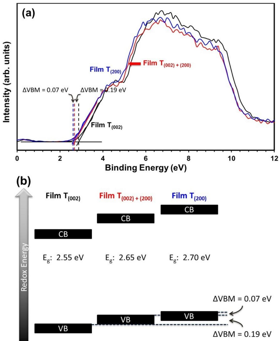
**Figure S6.** (a) XPS valence band and (b) electronic band structure of films T<sub>(002)</sub>, T<sub>(002)+(200)</sub>, and T<sub>(200)</sub> determined using XPS (Figure S6(a)) and UV-Visible spectrophotometry (Figure 7);  $E_g$ , CB, VB, and  $\Delta\text{VBM}$  are optical indirect band gap, conduction band, valence band, and energy difference in valence band maxima, respectively.
