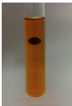
Figure S1. Top: Sealed reaction vessel equipped with oxygen sensor spots, mounted inside in a custom air cooling reactor. Bottom: Catalytic solution, containing [\text{Ru}(\text{dpp})(\text{pic})_2](\text{PF}_6)_2 (2.6 \mu\text{M} ) as catalyst and [\text{Ru}(\text{dceb})_2(\text{bpy})](\text{PF}_6)_2 (0.3 mM) as photosensitizer.
