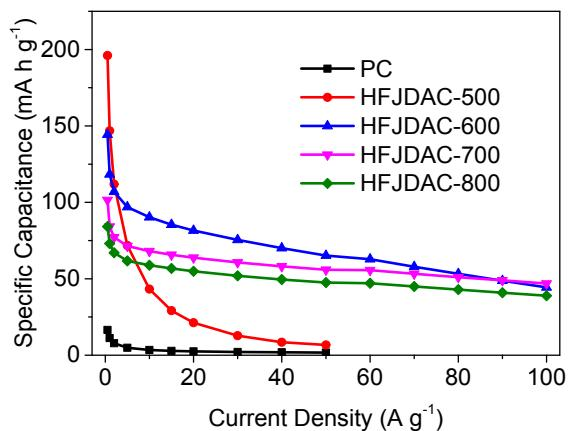
**Fig. S8** Specific capacitances ( $\text{mA h g}^{-1}$ ) at different current densities.
