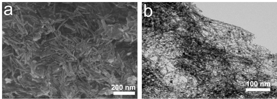
**Fig. S12** (a) SEM image and (b) TEM image of  $\text{NiCo}_2\text{O}_4/\text{GR}$ , (c) XRD pattern of  $\text{NiCo}_2\text{O}_4/\text{GR}$ , the diffraction peak marked with \* is indexed as (002) graphitic peak associated with the graphene nanoflakes, while the other peaks are indexed as equilibrium  $\text{NiCo}_2\text{O}_4$ .
