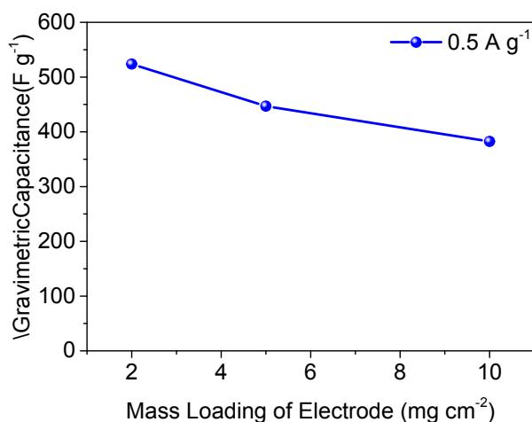
**Fig. S9** Comparison of the gravimetric capacitance of the HFJDAC-600 electrodes at different mass loading tested in a 2 M KOH electrolyte at a current density of  $0.5 \text{ A g}^{-1}$  between -1 and 0 V.
