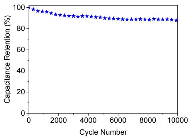
**Fig. S10** Cycling stability of HFJDAC-600 tested at  $20 \text{ A g}^{-1}$  for 10,000 cycles.
