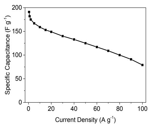
**Fig. S14** Specific capacitances of AC at different current densities in a three-electrode system tested in 2M KOH.
