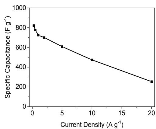
**Fig. S13** Specific capacitances of  $\text{NiCo}_2\text{O}_4/\text{GR}$  at different current densities in a three-electrode system tested in 2M KOH.
