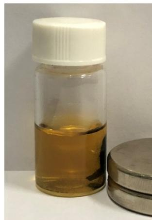
**Fig. S2** Images of biorefinery corncob lignin after catalytic hydrogenolysis reaction over the Ni/AC catalyst.
