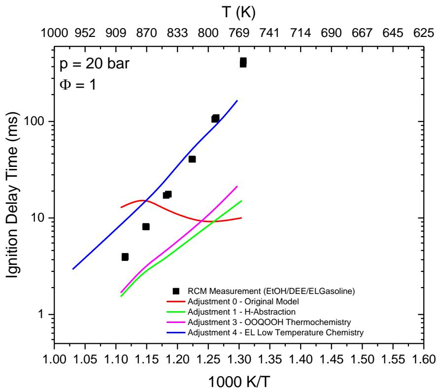
Figure S2. Comparison of modifications made to the kinetic model developed in this work. Adjustment 1 refers to the standardization of all the H-abstraction rate constants, and Adjustment 2 refers to the increasing of the formation enthalpy of the peroxy alkylhydroperoxide radicals (OOQOOH) in the diethyl ether sub model by 10 kJ/mol. Adjustment 3 refers to the addition of the EL low temperature combustion pathways.
