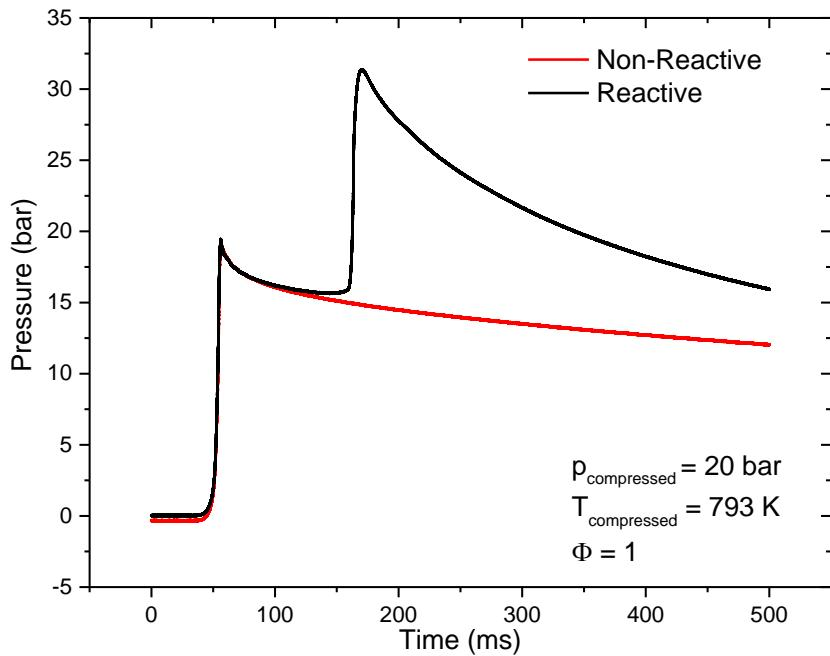
Figure S1. Exemplar rapid compression machine experimental pressure histories for the EL/DEE/EtOH Gasoline at compressed conditions of 20 bar, 793 K and  $\Phi = 1.0$ .
