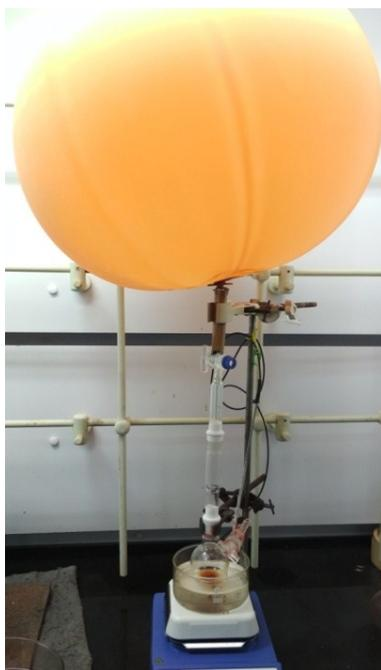
Figure. S24: Digital image of the experimental setup used for the conversion of epoxides to cyclic carbonates under CO<sub>2</sub> filled balloon condition.
