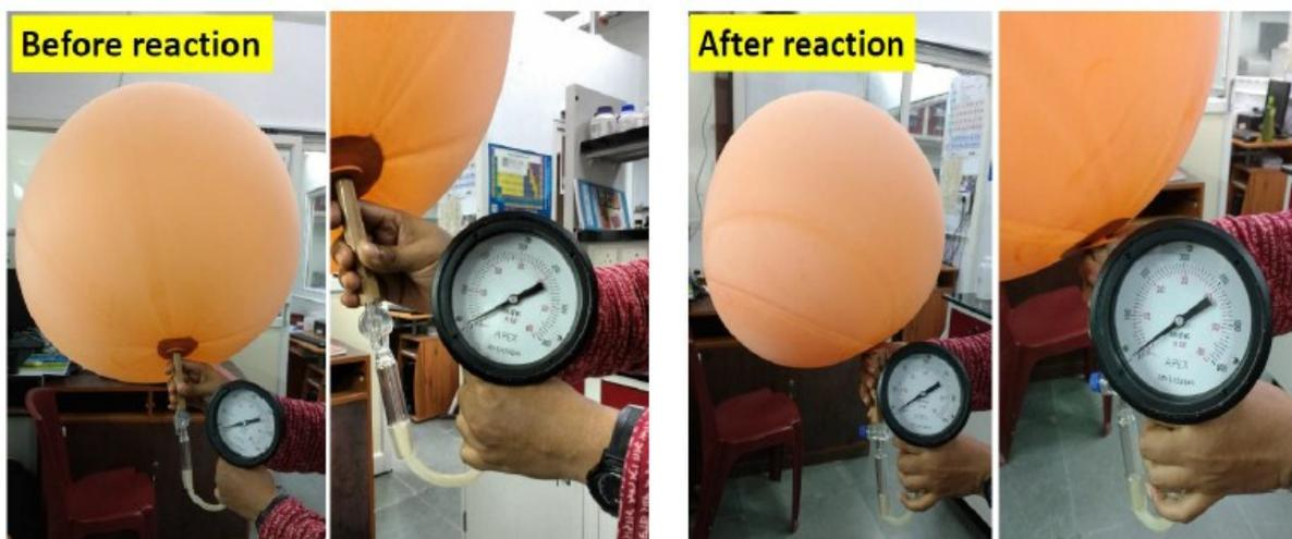
Figure.S23: Digital images showing the measurement of balloon pressure before and after the reaction
