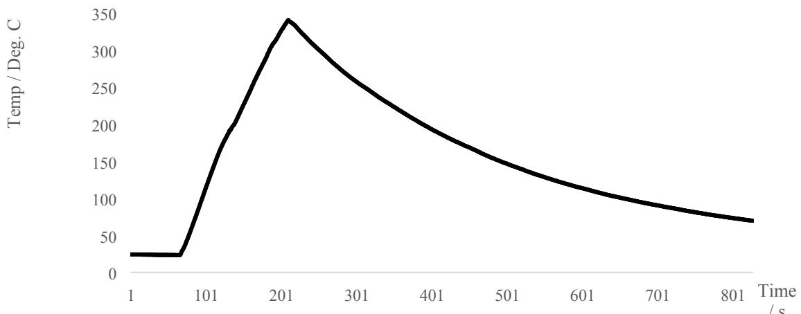
**Figure S1.** Typical temperature profile for the HTL reaction
