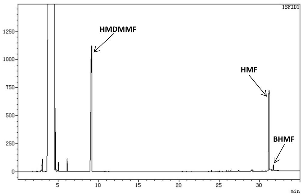
**Fig. S4** GC chromatogram for the CTH of HMF in MeOH over Hf-DTMP.
