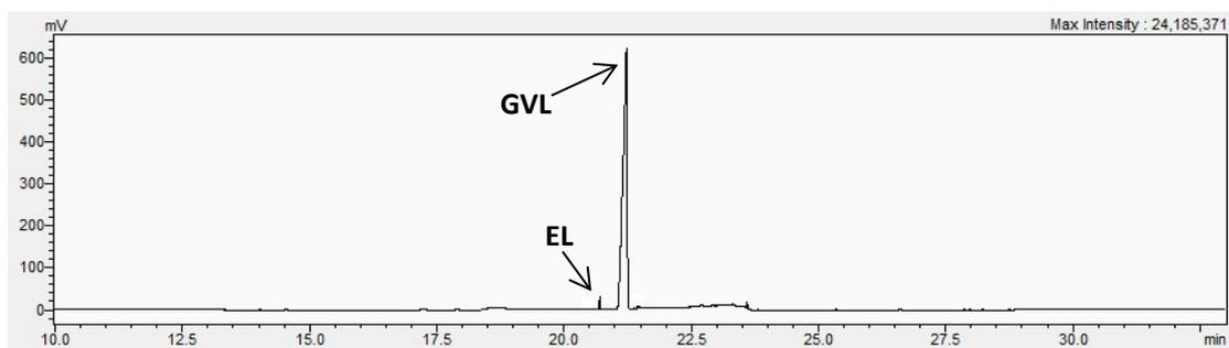
**Fig. S16** GC chromatogram for the CTH of EL in sBuOH over Hf-DTMP.
