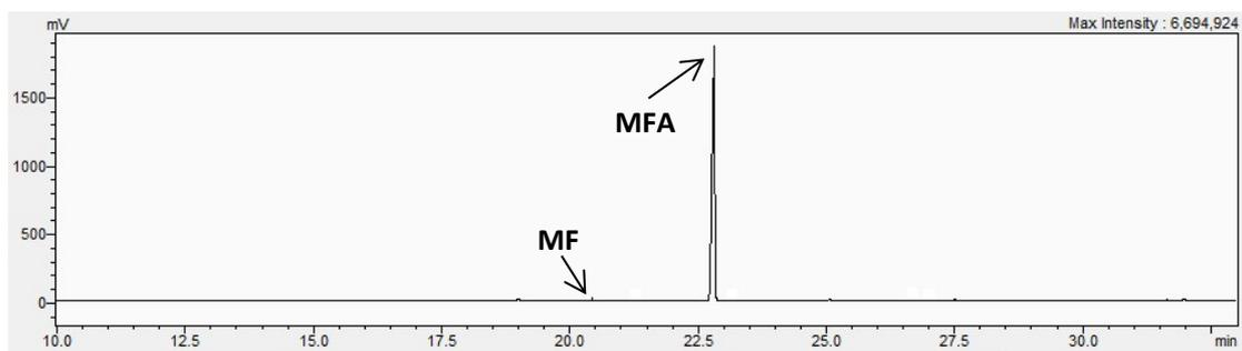
**Fig. S11** GC chromatogram for the CTH of MF in sBuOH over Hf-DTMP.
