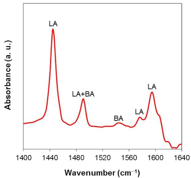
**Fig. S6** Pyridine-adsorbed FT-IR spectrum of Hf-DTMP.
