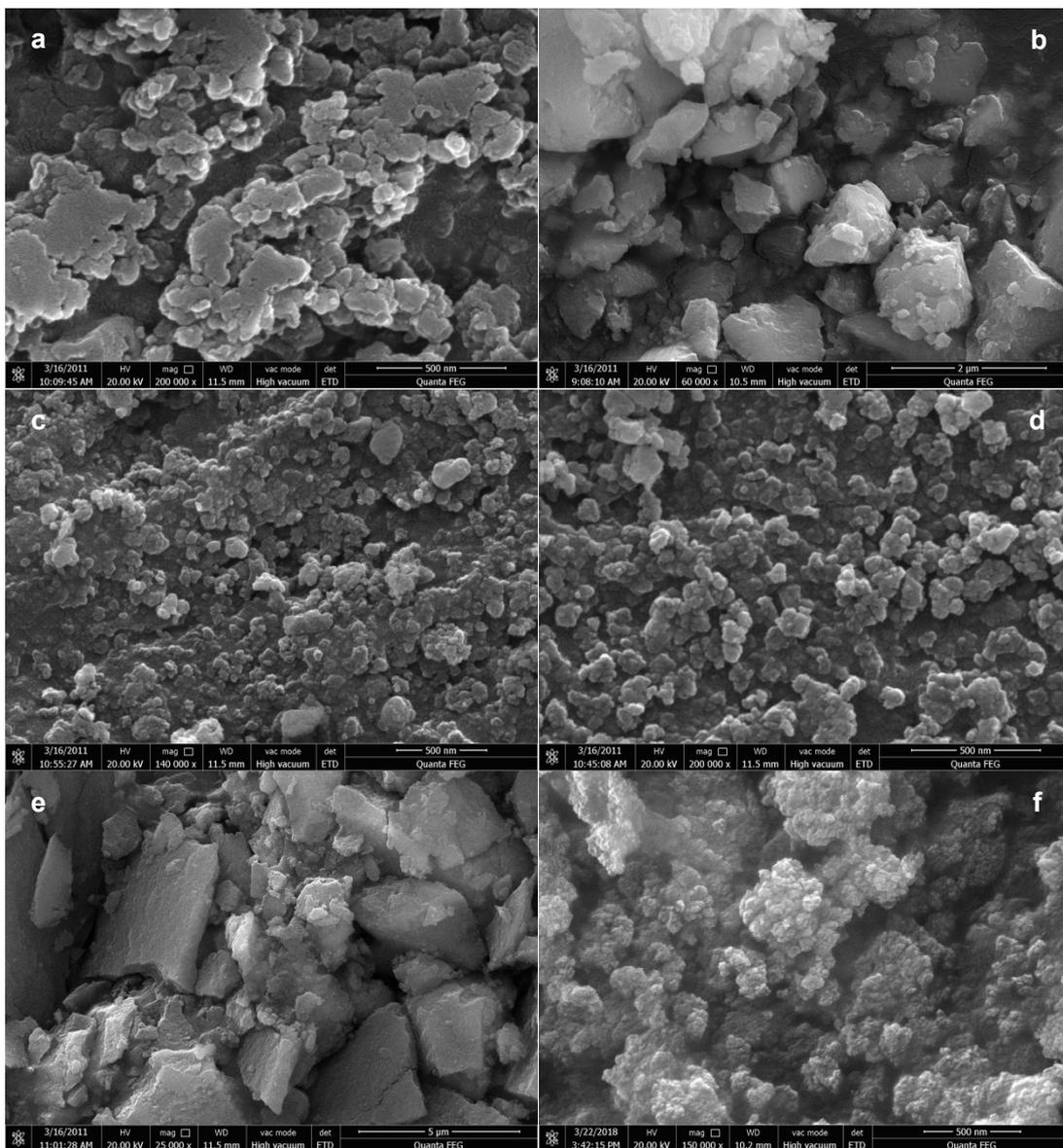
**Fig. S2** SEM images of Hf-BTC (a), Hf-ICA (b), Hf-IHP (c), Hf-ATMP (d), Sn-DTMP (e) and Nb-DTMP (f).
