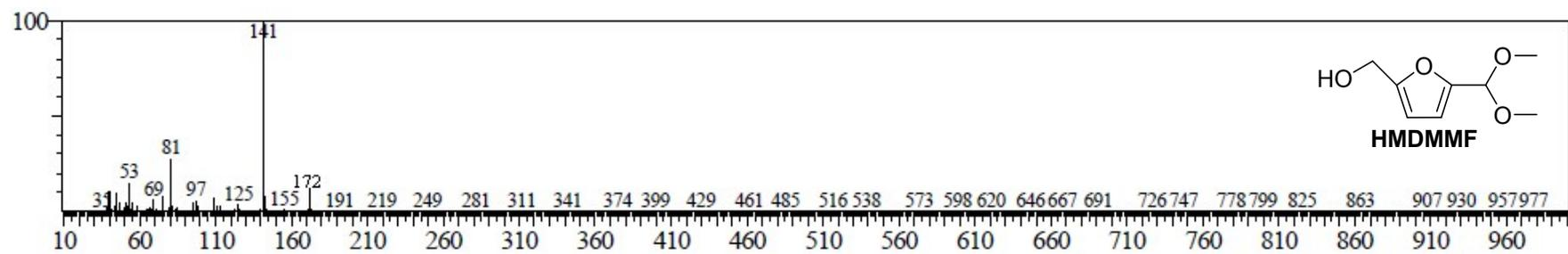
**Fig. S5** MS spectrum of HMDMMF.
