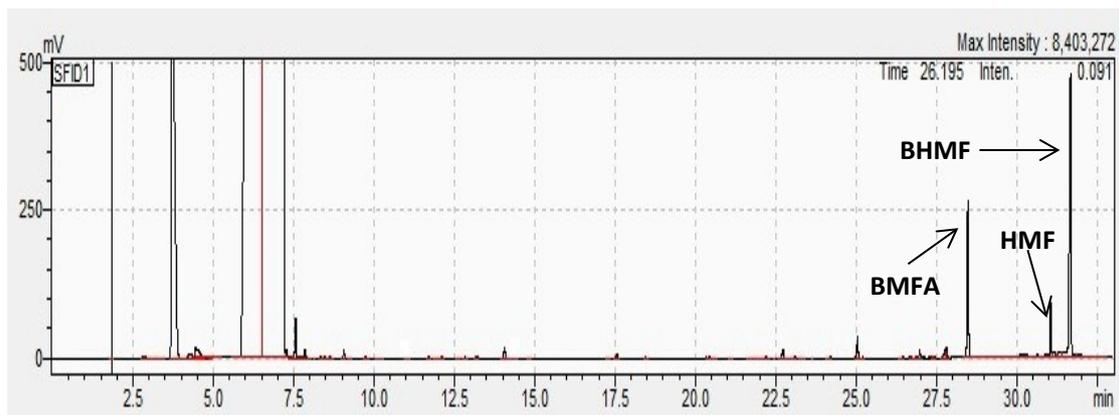
**Fig. S7** GC chromatogram for the CTH of HMF in sBuOH over Hf-DTMP.
