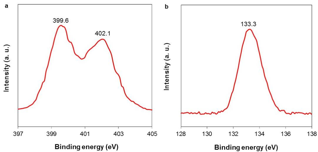
**Fig. S3** XPS spectra of N 1s (a) and P 2p (b) of Hf-DTMP.
