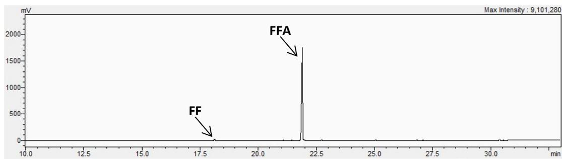
**Fig. S13** GC chromatogram for the CTH of FF in sBuOH over Hf-DTMP.
