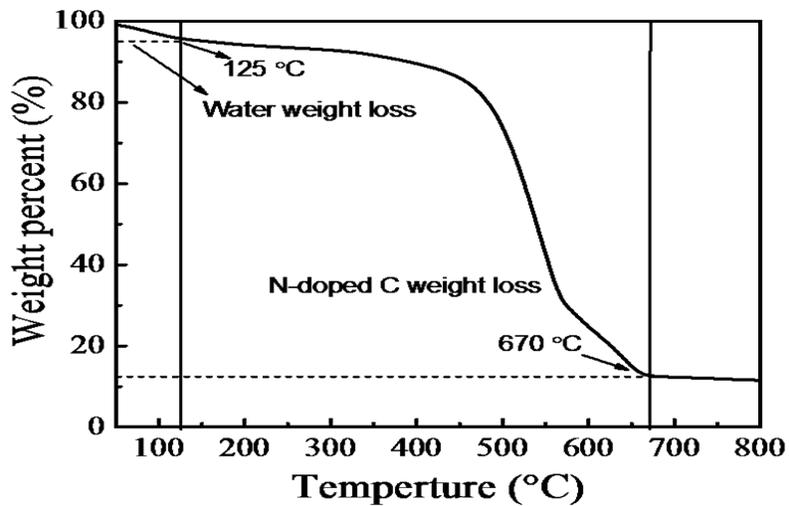
Fig. S2: TGA thermograms of ZnO-NC composite.
