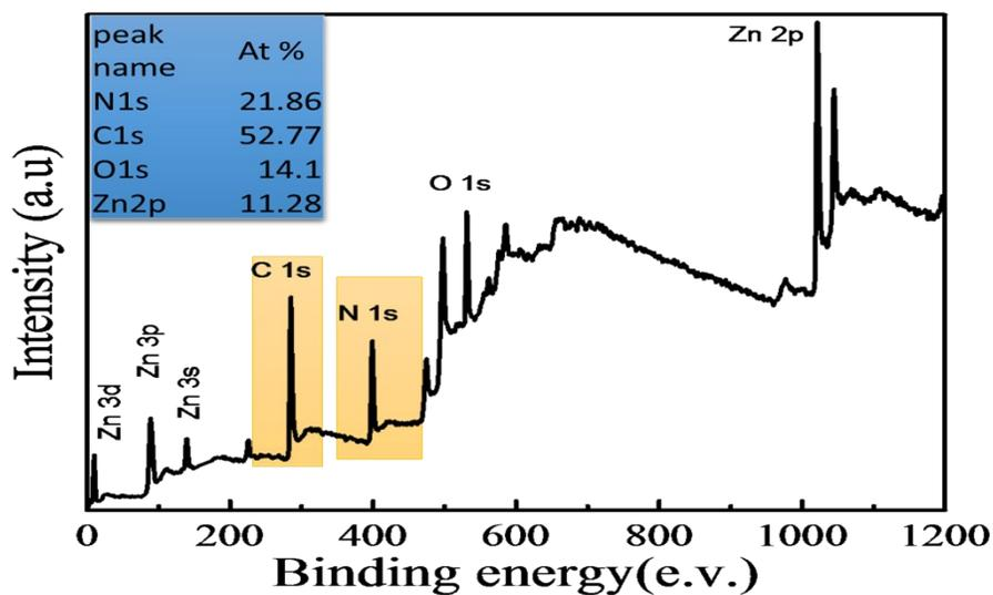
Fig. S4 XPS full-spectrum of ZnO-NC nanocomposite derived ZIF-8.
