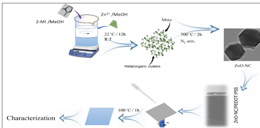
**Fig. S1:** Schematics for the prepare of ZnO-NC/PEDOT: PSS CE
