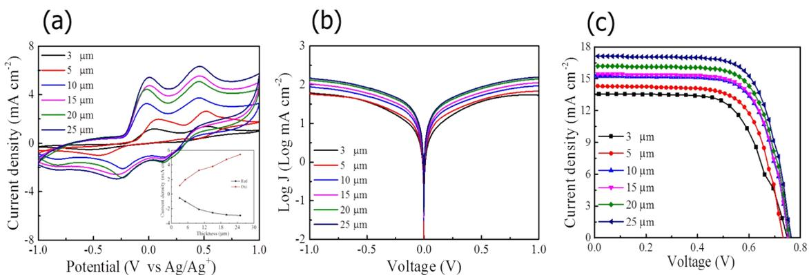
**Fig. S6** (a) CV curves, (b) Tafel polarization curves and (c) J-V curves of the DSSCs with 7% ZnO-NC/PEDOT: PSS CEs with different thickness.
