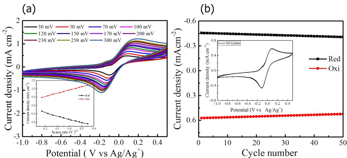
**Fig. S7** (a) CV curves at different scan rates; inside the relationship between peak current density and the square root of scan rates, and (b) 50 times continuous cycle scans CVs of the 7% ZnO-NC/PEDOT:PSS CE with the scan rate of 50 mV s<sup>-1</sup>.
