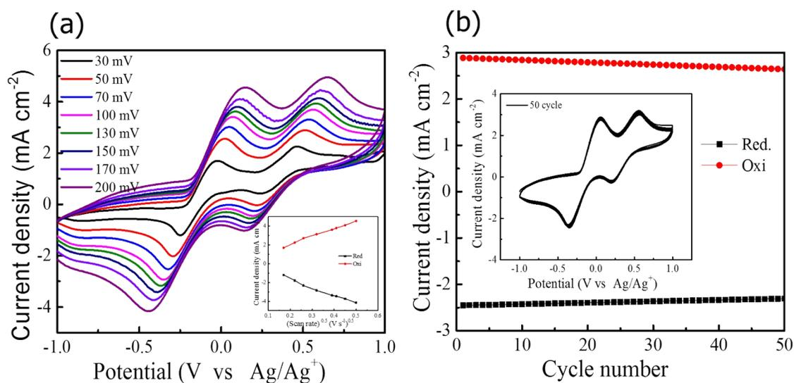
Fig.S4 (a) CV curves at different scan rates; inside the relationship between peak current density and the square root of scan rates, and (b) 50 times continuous cycle scans CVs of the 7% ZnO-NC/PEDOT: PSS CE with the scan rate of  $50 \text{ mV s}^{-1}$ .
