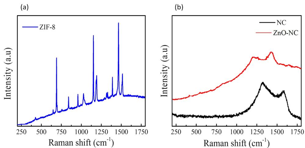
Fig. S3 Raman spectra of (a) ZIF-8 and (b) NC and ZnO-NC.
