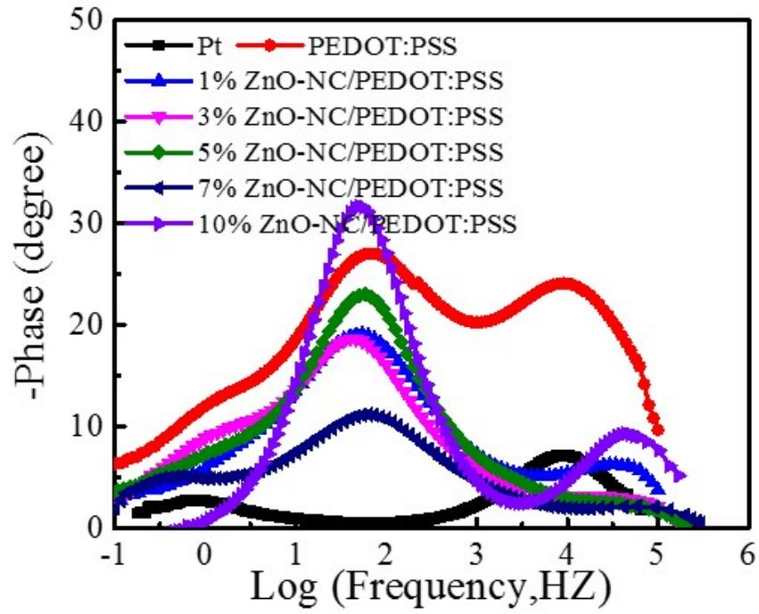
**Fig. S5** Bode plot of Pt, PEDOT: PSS and ZnO-NC/PEDOT: PSS based symmetric cells.
