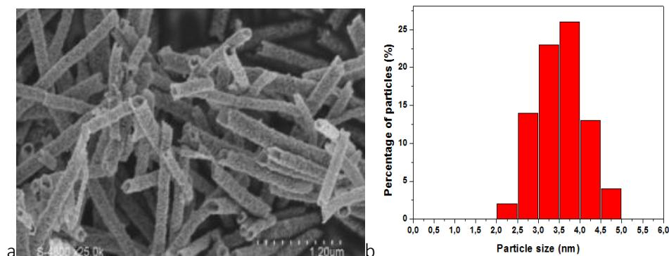
Figure SI1. SEM micrographs of ATO (a) and Pt size distribution histograms obtained by TEM analysis of Pt/ATO (b).
