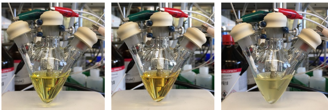
Figure S20 – Photos of a CPE experiment containing Ni(TAPPy) 2 (0.50 mM) and 0.1 M n Bu 4 NPF 6 in DMF at 0 h (left), 2 h (middle), and 6 h (right). Conditions: Pt mesh WE, Mg rod CE, Ag/AgCl pseudoreference, -2.5 V applied potential vs. Fc +0 .
