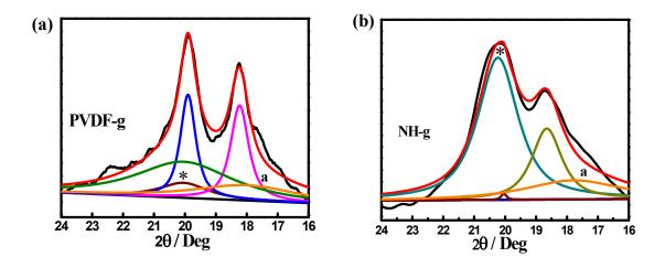
**Figure S3:** Deconvolation of **(a)** PVDF graft with P3-HT; **(b)** NH graft with P3-HT .The (a) peak indicate the area of the amorphous phase of PVDF-g and NH-g system and the (\*) peak indicate the area of the piezoelectric β-phase of PVDF-g and NH-g specimens. The β-phase fractions after grafting were 8 and 59% in PVDF-g and NH-g, respectively. This is to mention that PVDF does not possess any β-phase before irradiation while ~25% polar β-phase is observed in NH.
