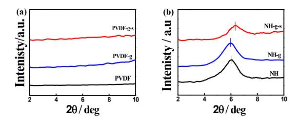
**Figure S2:** XRD patterns of (a) PVDF, PVDF-g and PVDF-g-s and (b) NH, NH-g, and NH-g-s to understand the nanostructure and marked lines indicate the peak positions of nanoclay dispersed in polymer matrix. The nanostructural investigation of the nanohybrid, before and after sulphonation, has been presented in **Supplementary fig. S2.** Pristine PVDF does not show any nanostructure peak in XRD pattern while in nanohybrids peak at  $2\theta = 6.1^{\circ}$  indicating intercalated structure.
