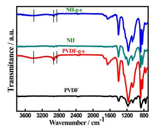
**Figure S1:** FTIR spectra of before irradiation (PVDF, NH) and after irradiation and grafting (PVDF-g, NH-g) (functionalized membrane) and indicating the stretching vibration frequency through the vertical lines.
