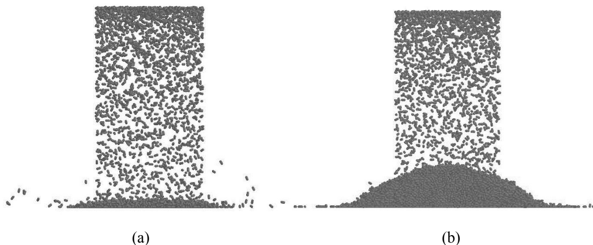
Suppl. Fig. 1 Snapshot of the “rainfall-like” piling method at different time, where: (a) 0.5 s; and (b) 3 s with the aspect ratio of the spherocylinder AR = 1.5 .
