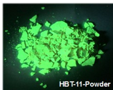
Fig. S9 Photograph showing the color of HBT-11 powder under illumination of 365 nm light.
