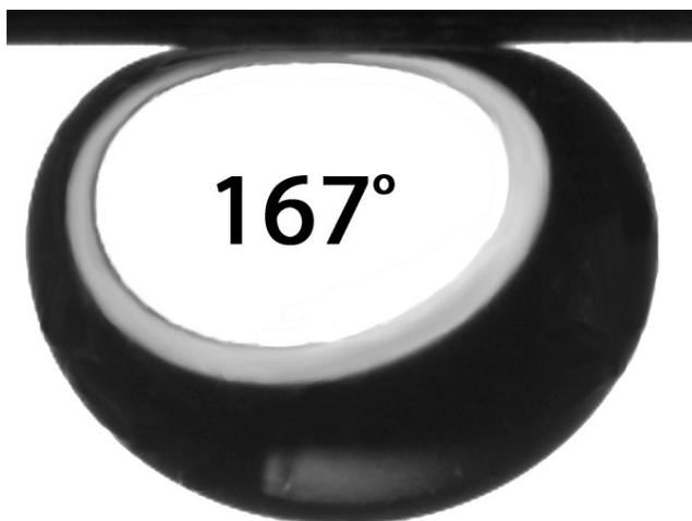
**Fig. S2:** Underwater contact angle of hexadecane on a 22 nm-thick smooth gold film.
