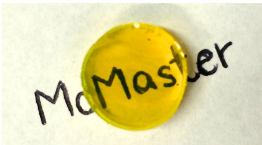
**Figure S-6:** Image of as formed PMM-CVS<sub>30</sub>-f 5% w/v HS-PEG-SH hydrogel, demonstrating high transparency.
